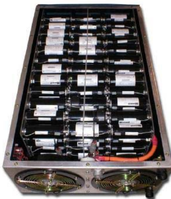
Figure 13: Supercapacitor Bank, 360 V -150 kW 320 Wh
