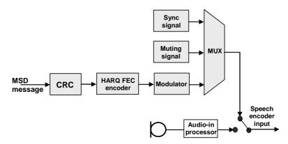
Figure 5: IVS transmitter block diagram
