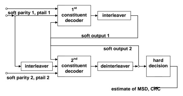
Figure 18: Turbo decoder
