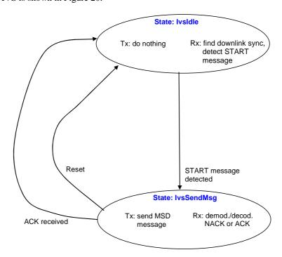
Figure 20: State model of the IVS
