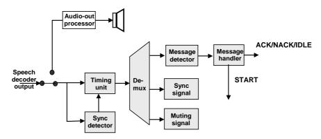
Figure 13: IVS receiver block diagram
