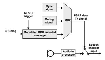
Figure 15: PSAP transmitter block diagram
