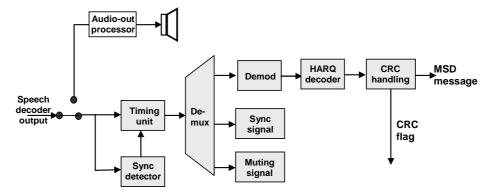
Figure 17: PSAP receiver block diagram
