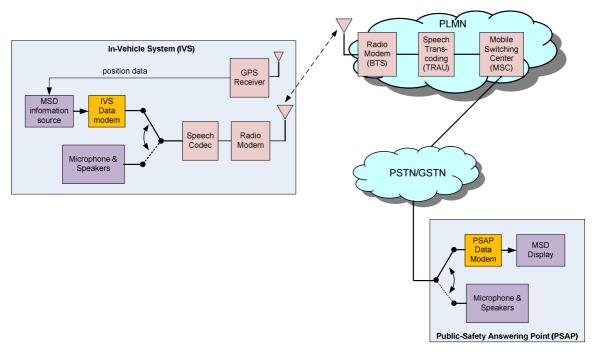
Figure 2: eCall system within the cellular system architecture
