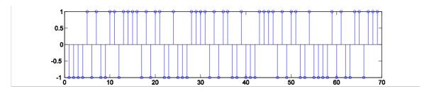
Figure 10: Pulse sequence for generation of synchronization preamble
