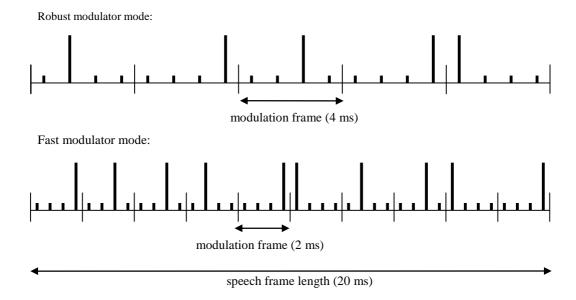
Figure 8: Slot structure of uplink modulator
