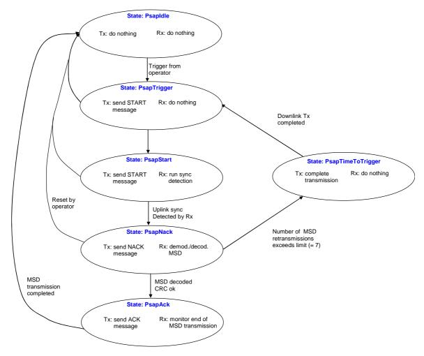
Figure 19: State model of the PSAP
