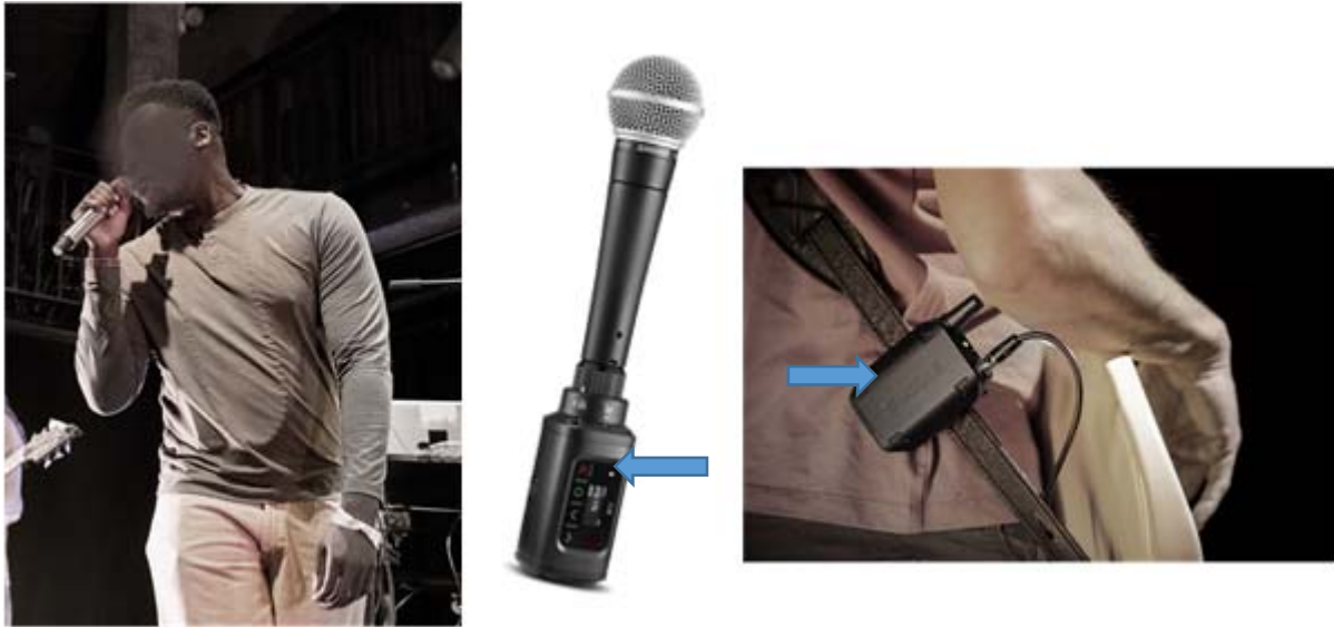
Figure 2: Singer using a handheld microphone (left), plug-on transmitter (middle), bodypack transmitter (right)
