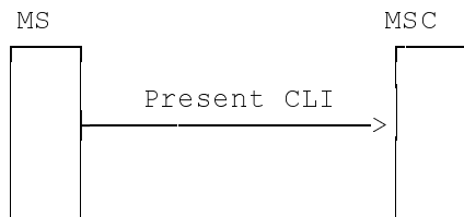
Figure 2.1: MS indicating presentation of CLI when CLIR is provisioned in temporary mode with default value "presentation restricted"
