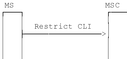
Figure 2.2: MS invoking CLIR, when CLIR is provisioned in temporary mode with default value "presentation allowed"
