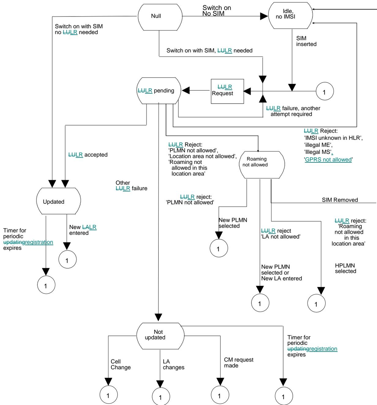
NOTE: Whenever the MS goes to connected mode and then returns to idle mode again the MS selects appropriate state.
