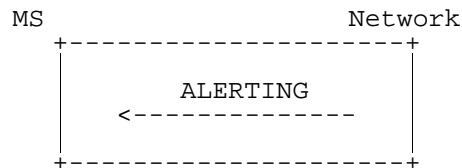
Figure 5.4/3GPP TS 04.08: Call confirmation at mobile originating call establishment
