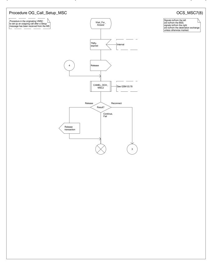
Figure 8g: Procedure Outgoing\_Call\_Setup \_MSC (sheet 7)
