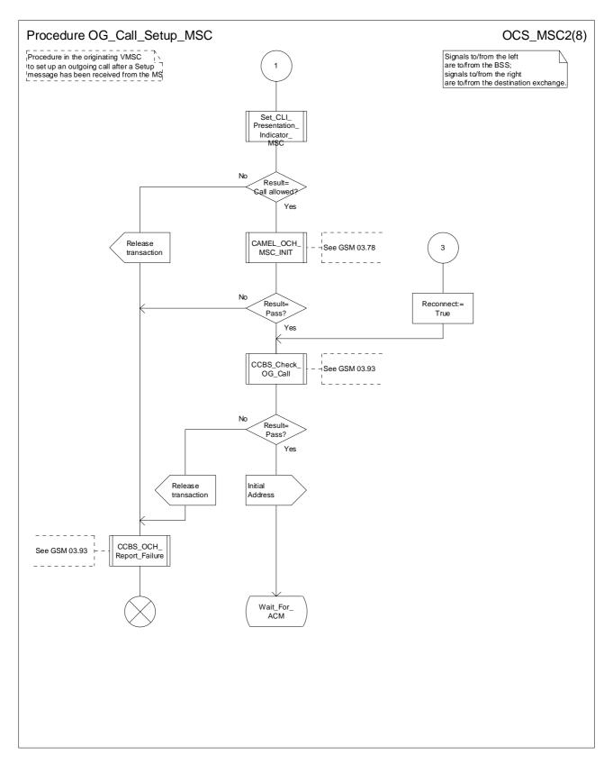
Figure 8b: Procedure Outgoing\_Call\_Setup \_MSC (sheet 2)
