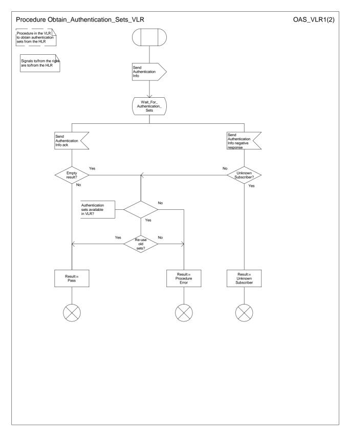
Figure 25a: Procedure Obtain\_Authentication\_Sets\_VLR (sheet 1)
