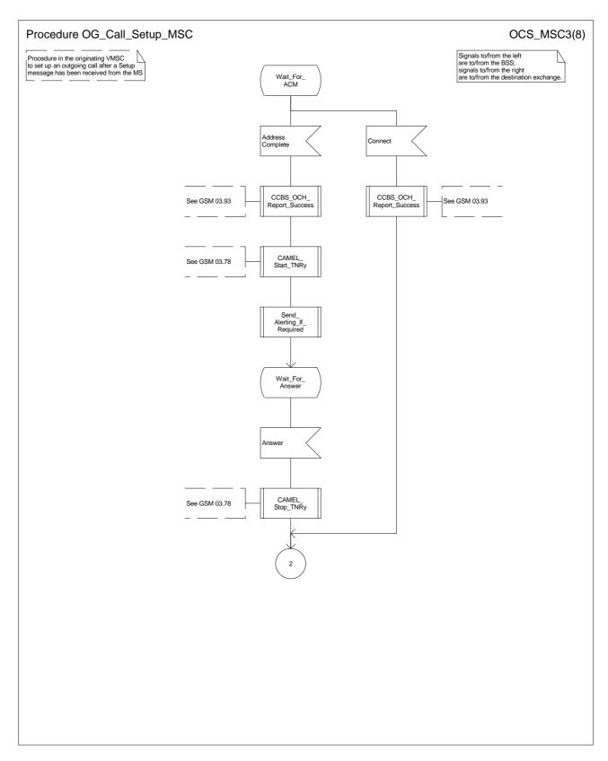
Figure 8c: Procedure Outgoing\_Call\_Setup \_MSC (sheet 3)
