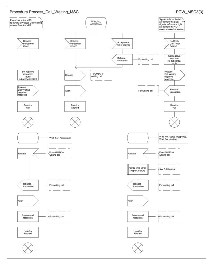
Figure 62c: Procedure Process\_Call\_Waiting\_MSC(sheet 3)
