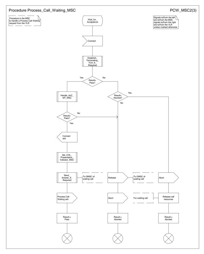
Figure 62b: Procedure Process\_Call\_Waiting\_MSC (sheet 2)
