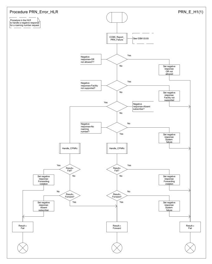
Figure 47: Procedure PRN\_Error\_HLR
