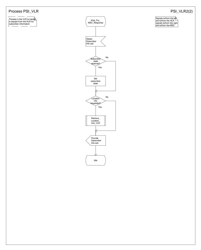
Figure 56b: Process PSI\_VLR (sheet 2)
