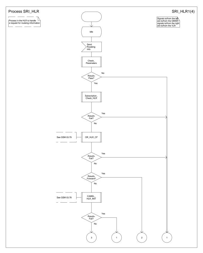
Figure 43a: Process SRI\_HLR (sheet 1)
