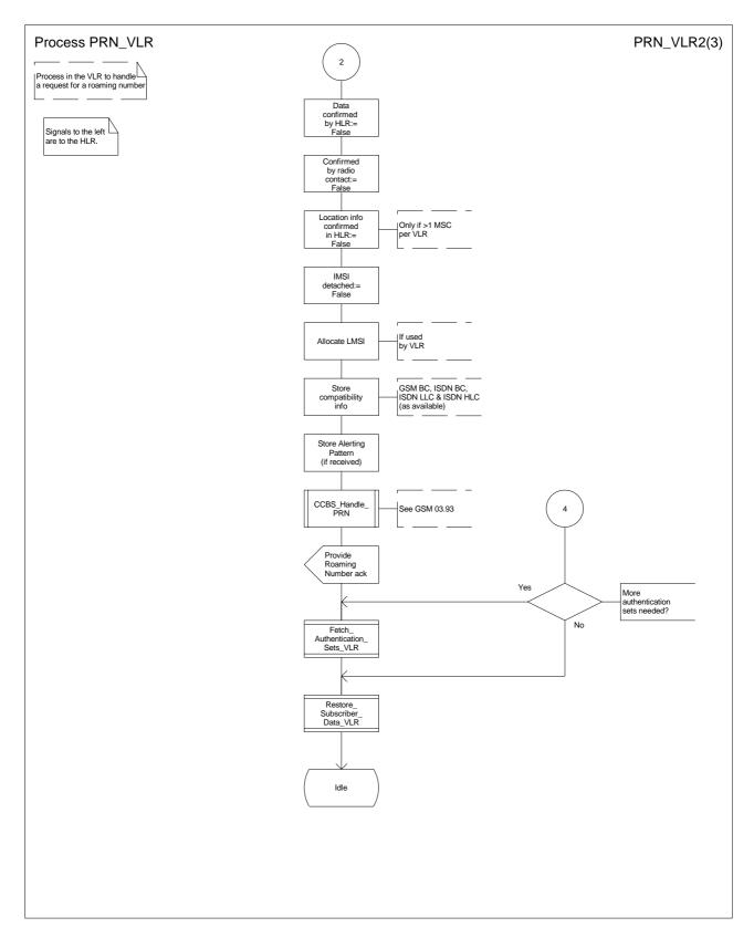
Figure 54b: Process PRN\_VLR (sheet 2)
