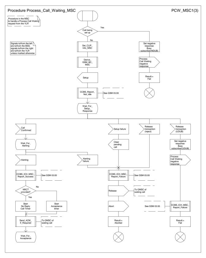
Figure 62a: Procedure Process\_Call\_Waiting\_MSC (sheet 1)
