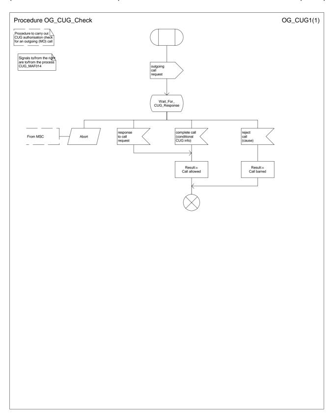
Figure 31: Procedure OG\_CUG\_Check
