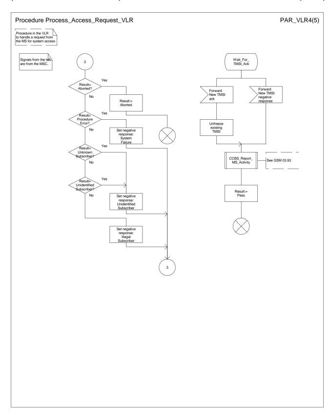
Figure 20d: Procedure Process\_Access\_Request\_VLR (sheet 4)
