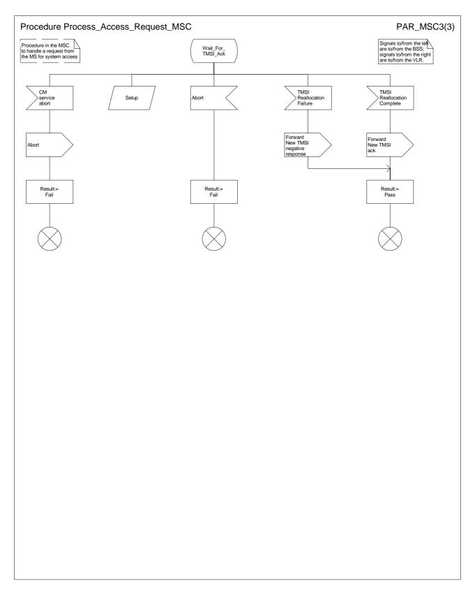
Figure 7c: Procedure Process\_Access\_Request\_MSC (sheet 3)
