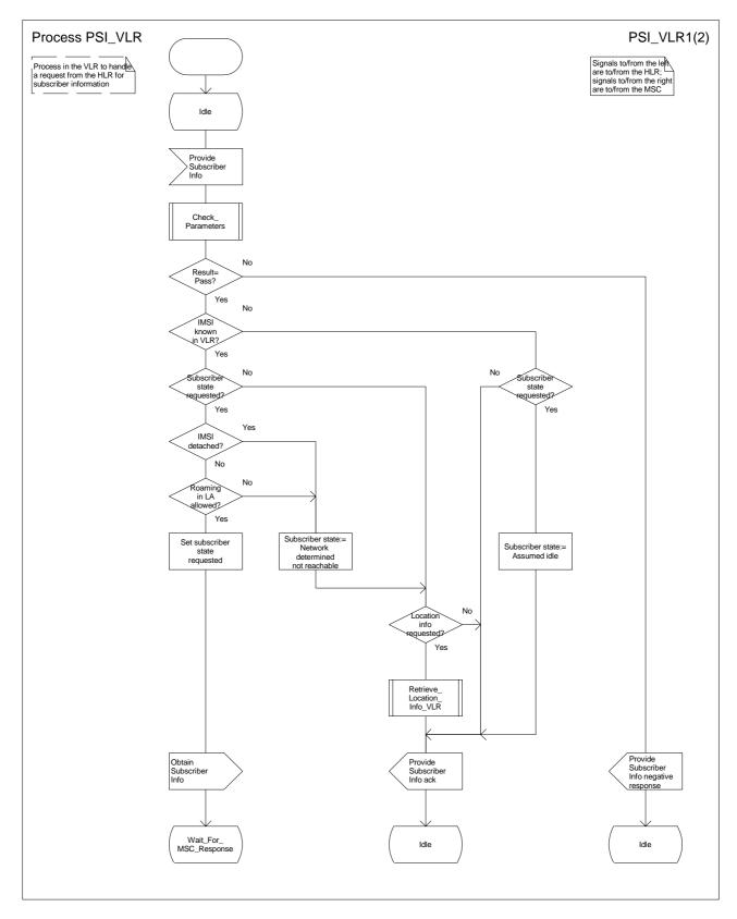
Figure 56a: Process PSI\_VLR (sheet 1)
