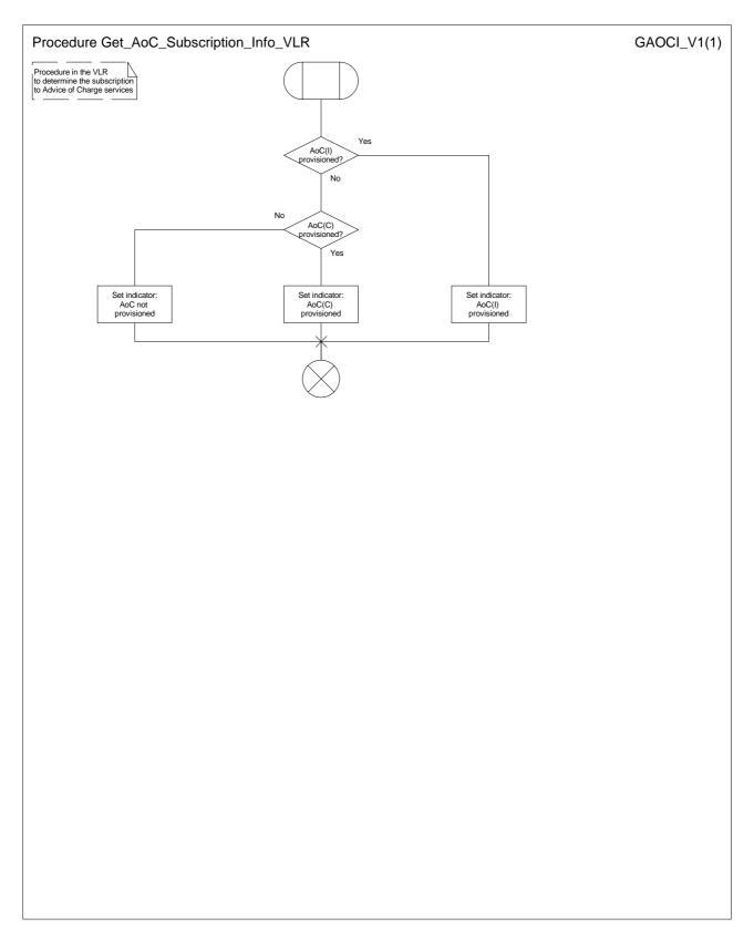
Figure 33: Procedure Get\_AoC\_Subscription\_Info\_VLR
