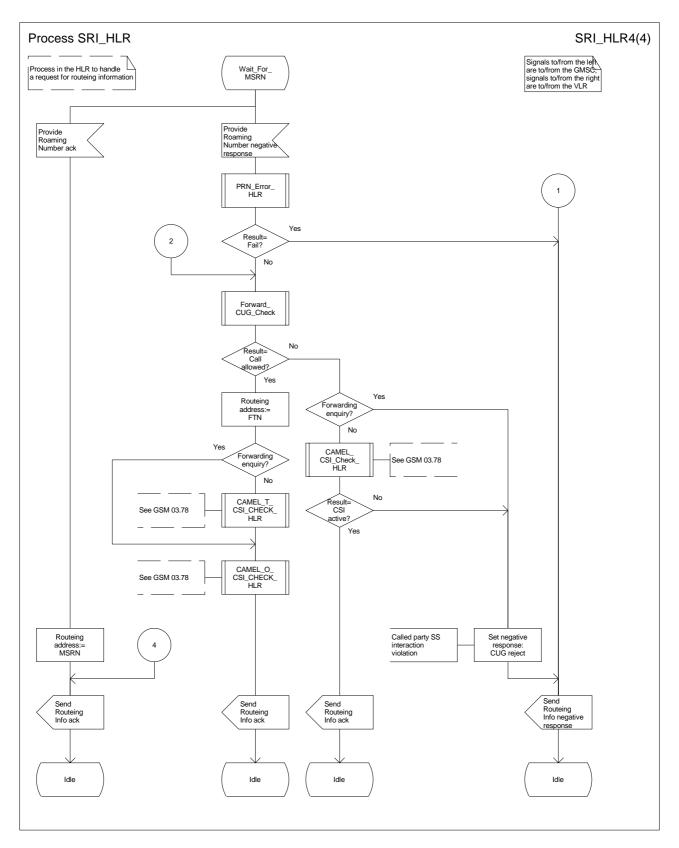
Figure 43d: Process SRI\_HLR (sheet 4)
