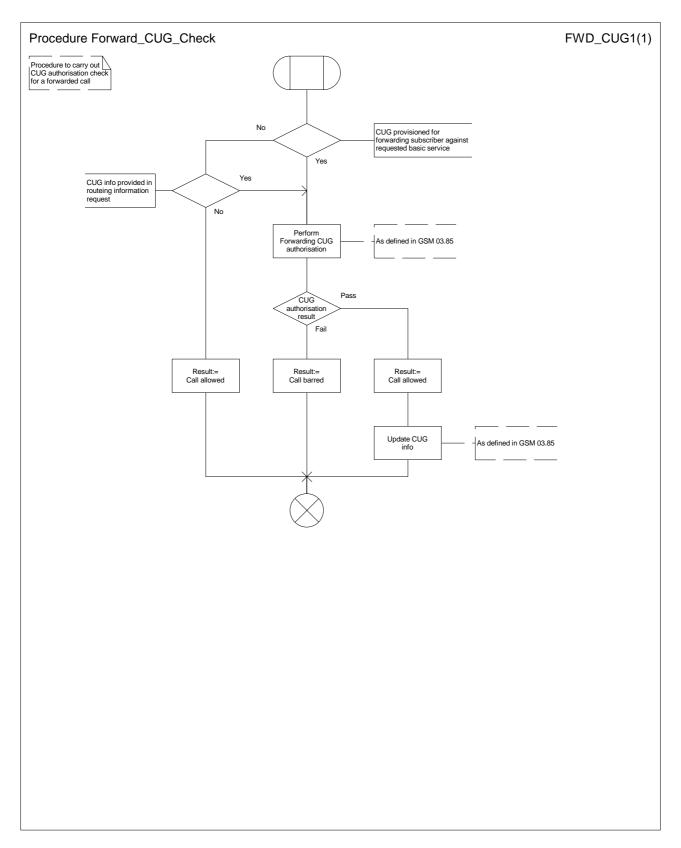
Figure 48: Procedure Forward \_CUG\_Check
