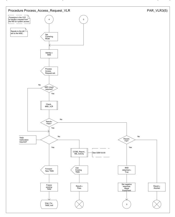
Figure 20c: Procedure Process\_Access\_Request\_VLR (sheet 3)
