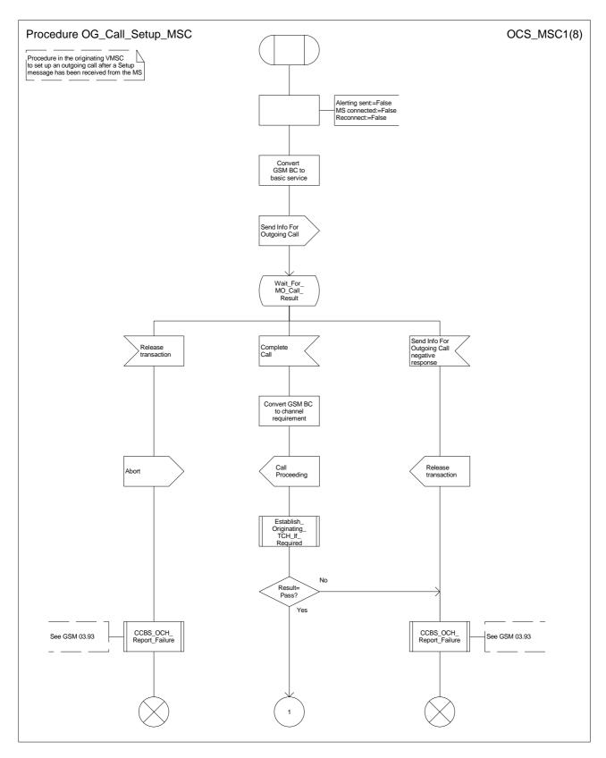
Figure 8a: Procedure Outgoing\_Call\_Setup\_MSC (sheet 1)
