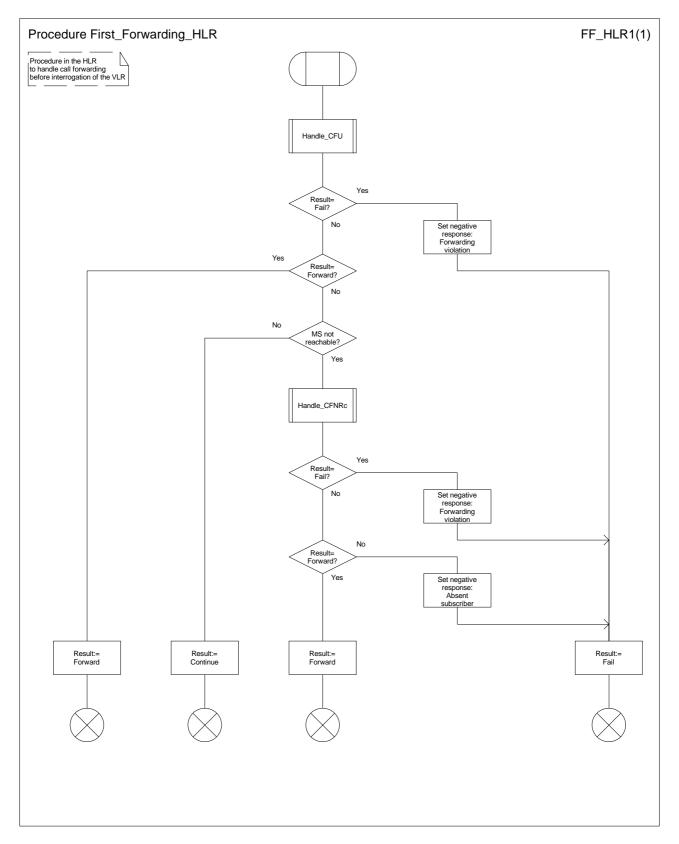
Figure 46: Procedure First\_Forwarding\_HLR
