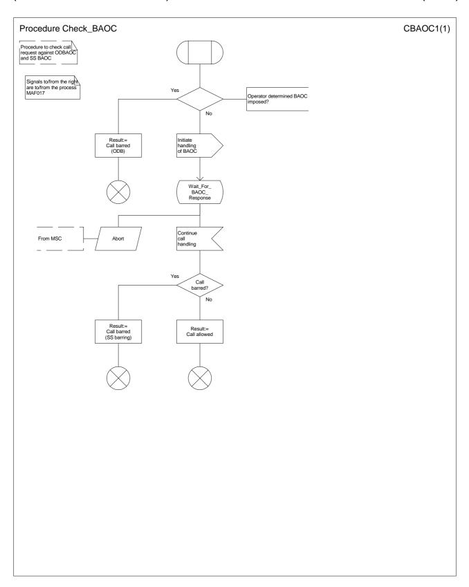
Figure 30: Procedure Check\_BAOC
