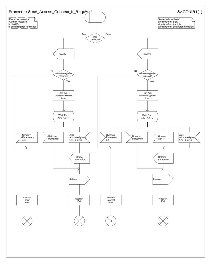
Figure 18: Procedure Send\_Access\_Connect\_If\_Required
