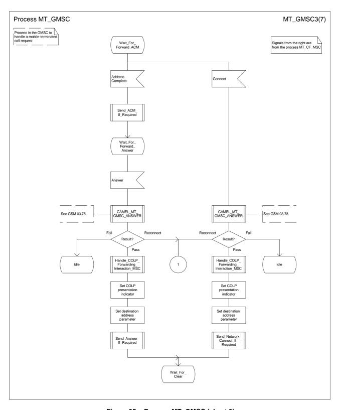
Figure 35c: Process MT\_GMSC (sheet 3)
