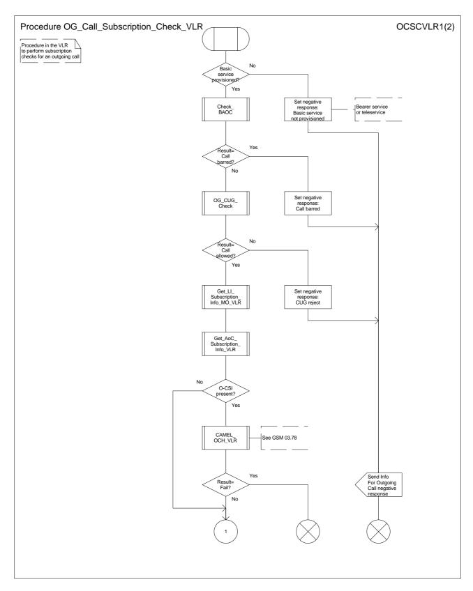
Figure 21a: Procedure OG\_Call\_Subscription\_Check\_VLR (sheet 1)
