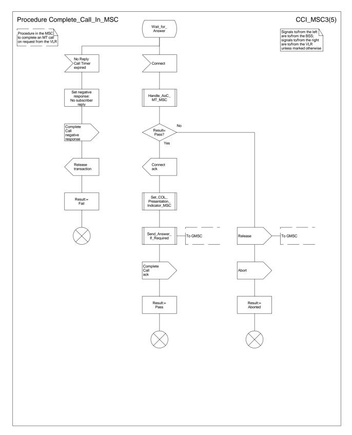
Figure 61c: Procedure Complete\_Call\_In\_MSC (sheet 3)
