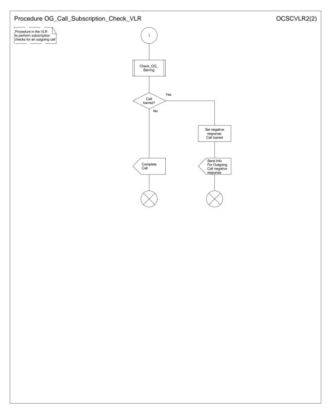
Figure 21b: Procedure OG\_Call\_Subscription\_Check \_VLR (sheet 2)
