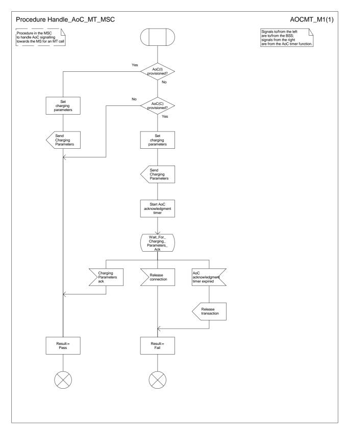
Figure 66: Procedure Handle\_AoC\_MT\_MSC
