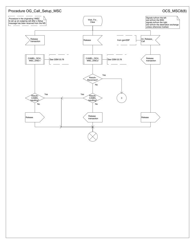
Figure 8h: Procedure Outgoing\_Call\_Setup \_MSC (sheet 8)
