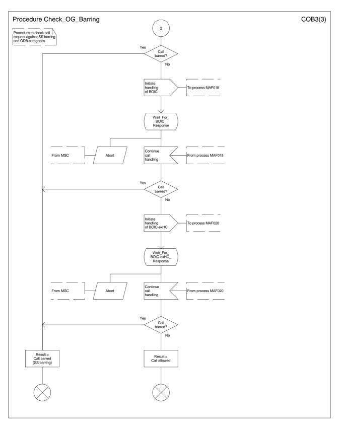
Figure 34c: Procedure Check\_OG\_Barring (sheet 3)
