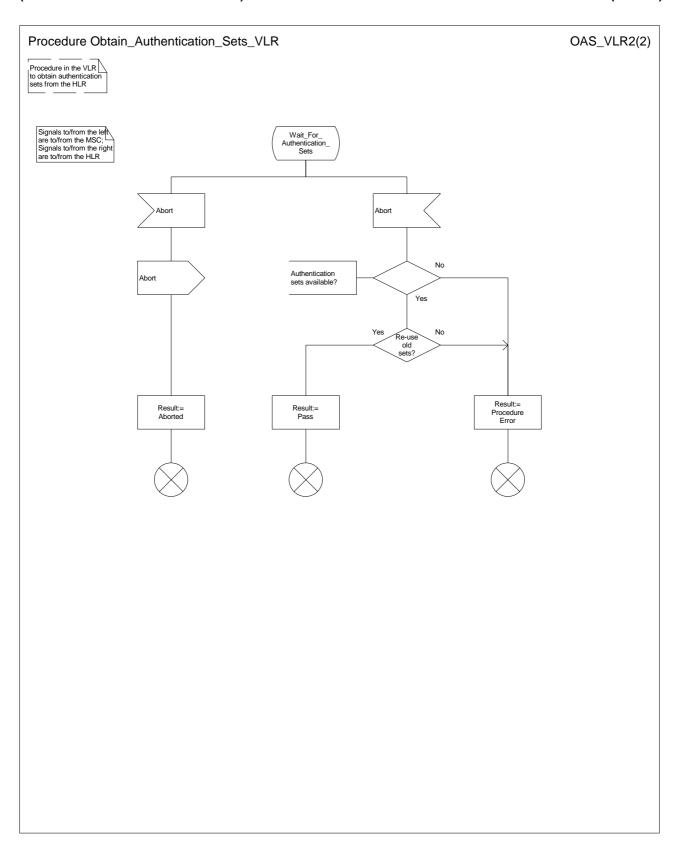
Figure 25b: Procedure Obtain\_Authentication\_Sets\_VLR (sheet 2)
