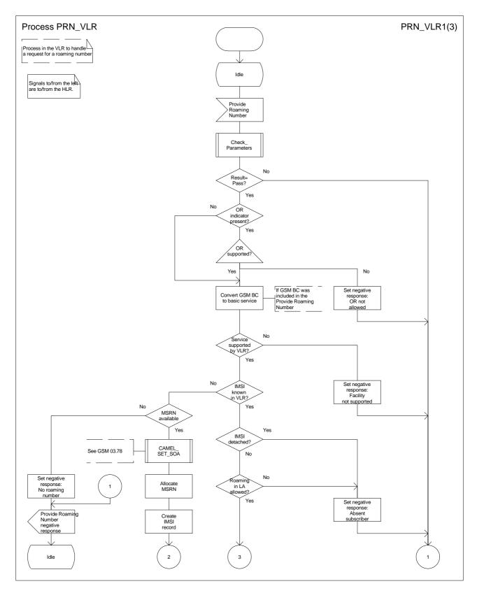
Figure 54a: Process PRN\_VLR (sheet 1)
