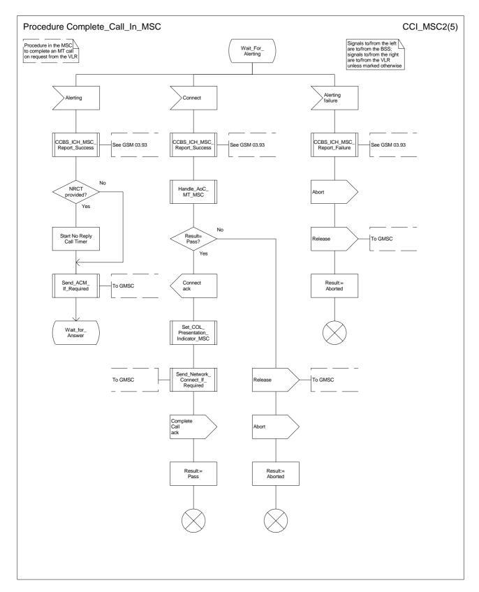
Figure 61b: Procedure Complete\_Call\_In\_MSC (sheet 2)
