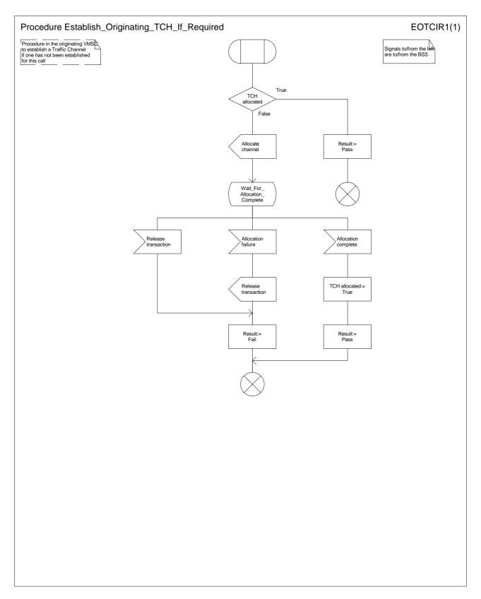
Figure 13: Procedure Establish\_Originating\_TCH\_If\_Required
