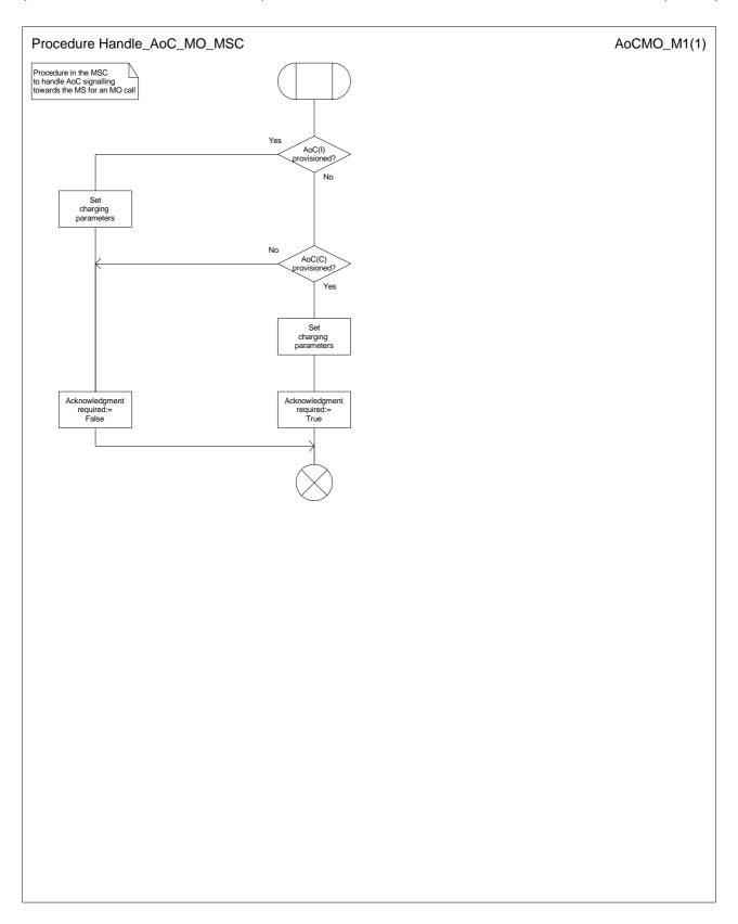
Figure 17: Procedure Handle\_AoC\_MO\_MSC
