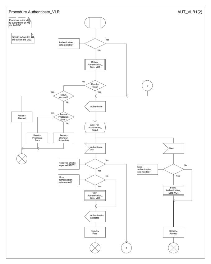
Figure 24a: Procedure Authenticate\_VLR (sheet 1)
