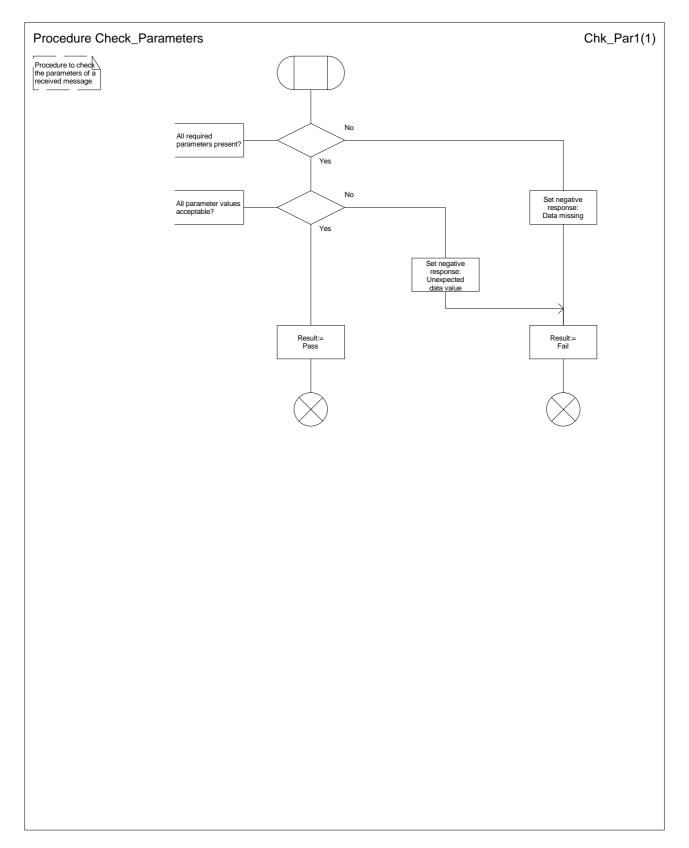
Figure 44: Procedure Check\_Parameters
