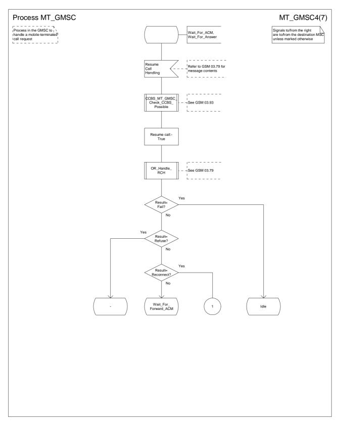
Figure 35d: Process MT\_GMSC (sheet 4)
