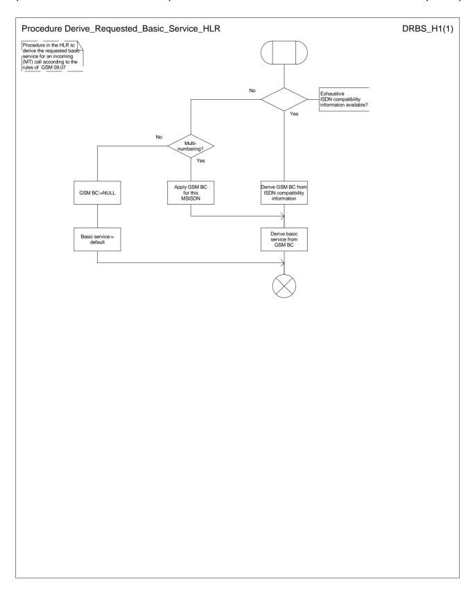
Figure 49: Procedure Derive\_Requested\_Basic\_Service\_HLR
