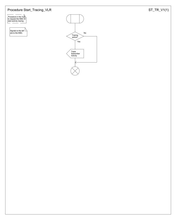
Figure 26: Procedure Start\_Tracing\_VLR
