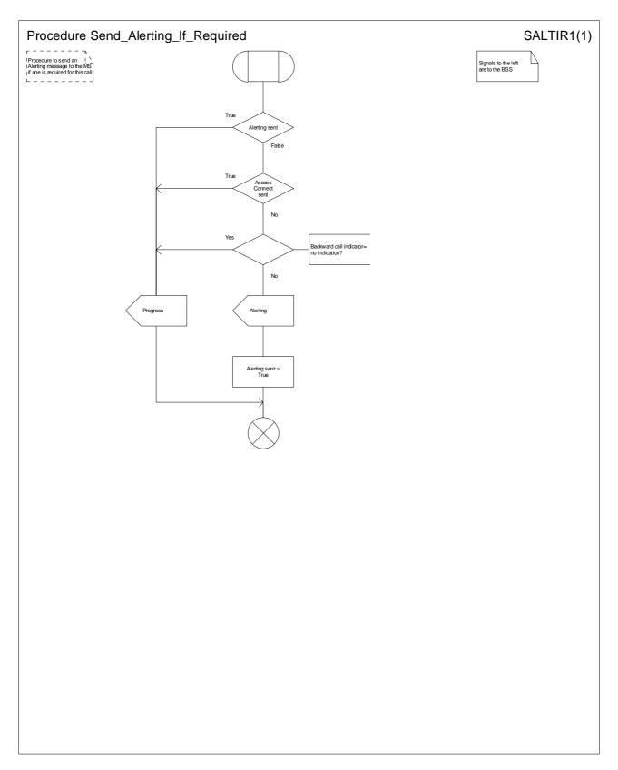
Figure 15: Procedure Send\_Alerting\_If\_Required
