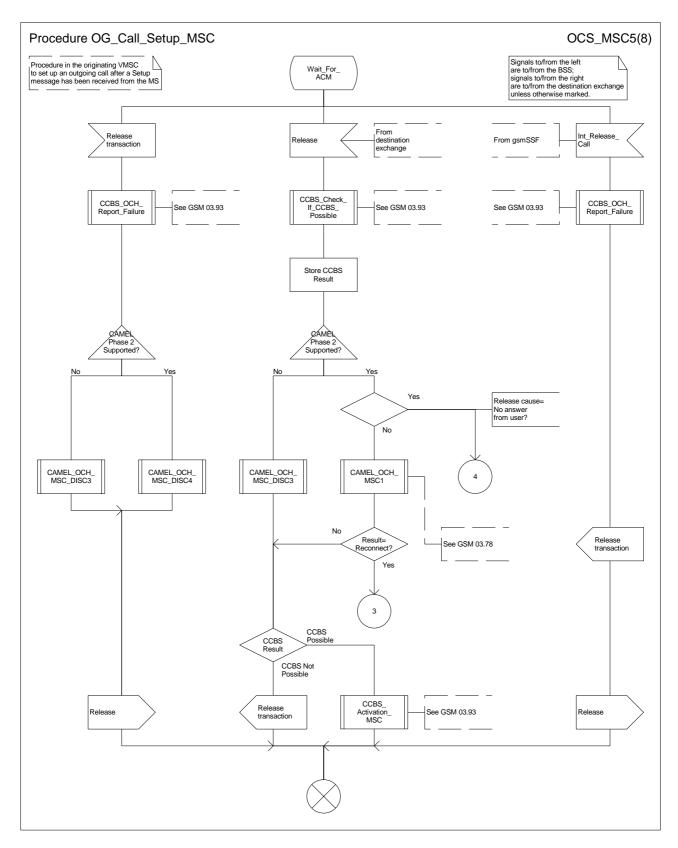
Figure 8e: Procedure Outgoing\_Call\_Setup \_MSC (sheet 5)
