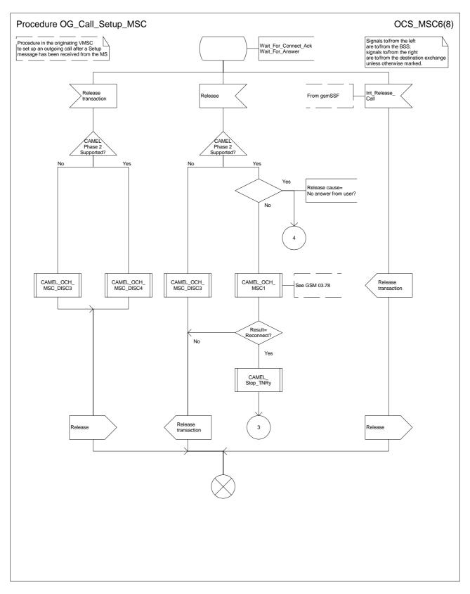
Figure 8f: Procedure Outgoing\_Call\_Setup \_MSC (sheet 6)
