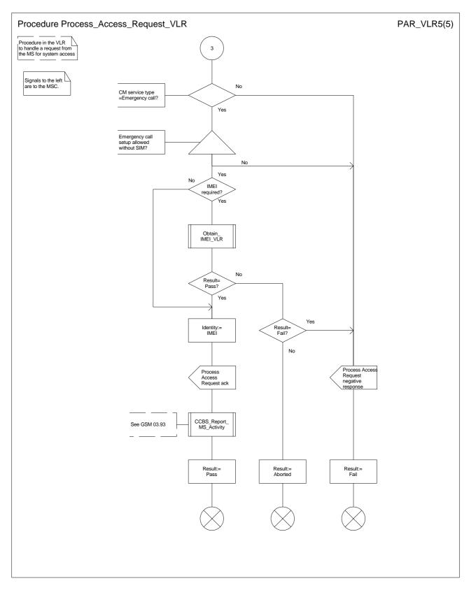
Figure 20e: Procedure Process\_Access\_Request\_VLR (sheet 5)
