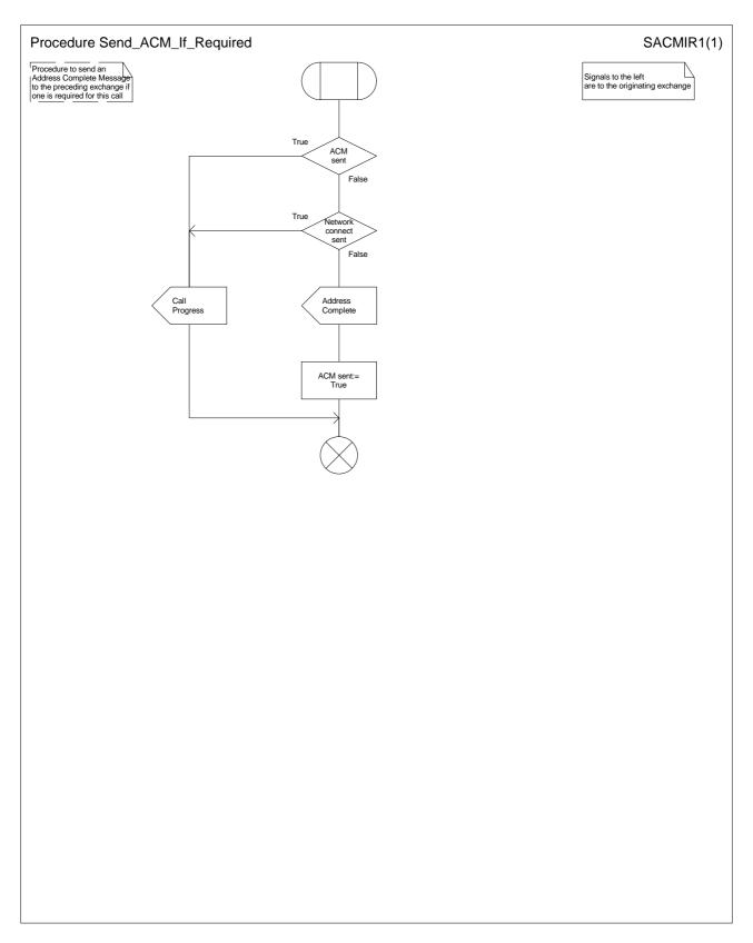
Figure 37: Procedure Send\_ACM\_If\_Required
