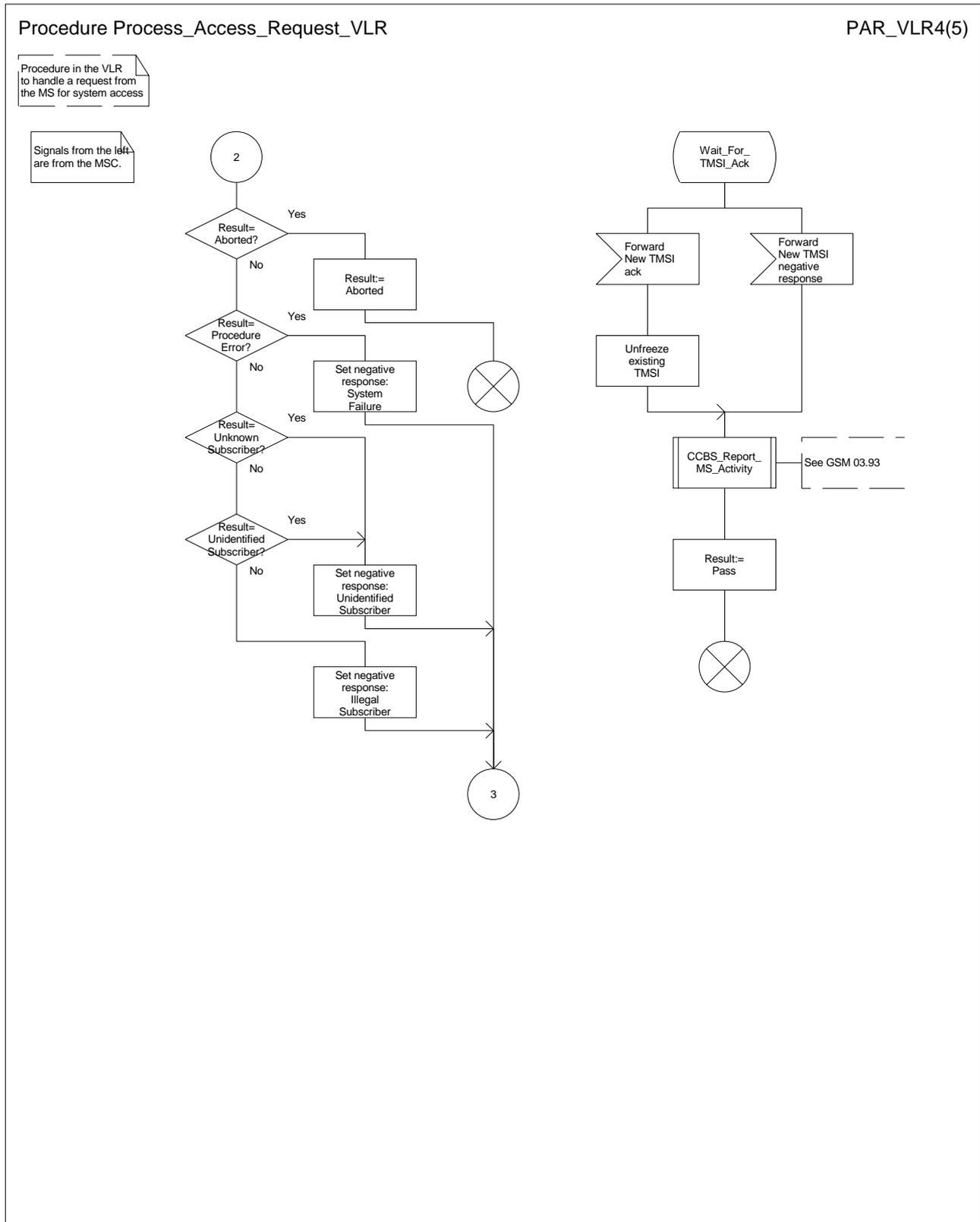
Figure 20d: Procedure Process\_Access\_Request\_VLR (sheet 4)
