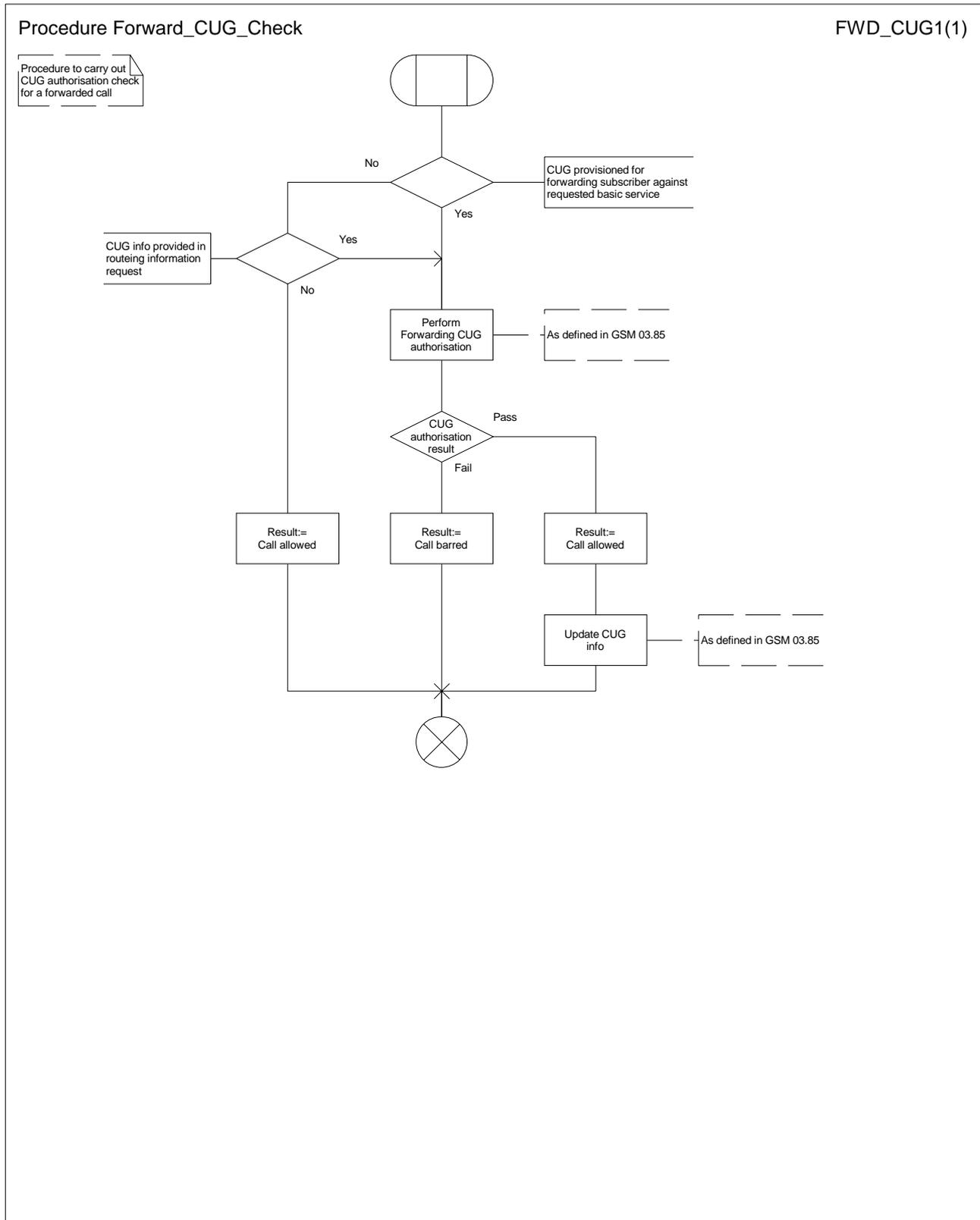
Figure 48: Procedure Forward\_CUG\_Check
