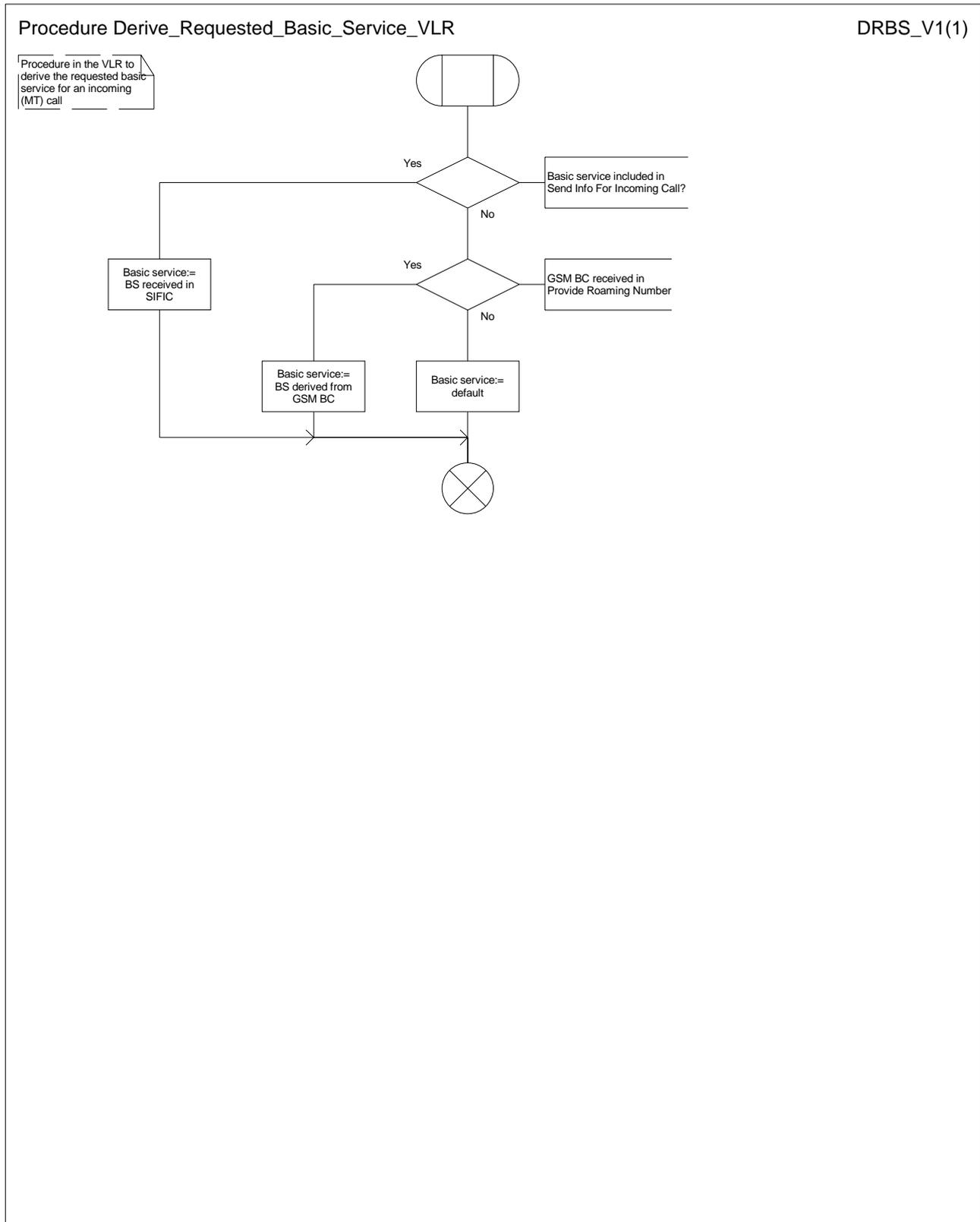
Figure 70: Procedure Derive\_Requested\_Basic\_Service\_VLR
