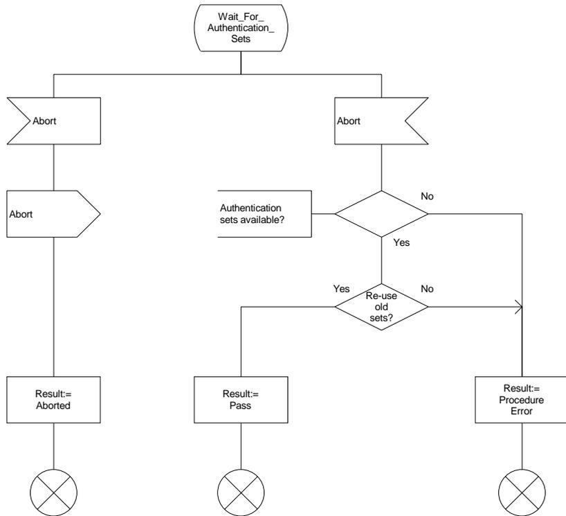
Figure 25b: Procedure Obtain\_Authentication\_Sets\_VLR (sheet 2)
