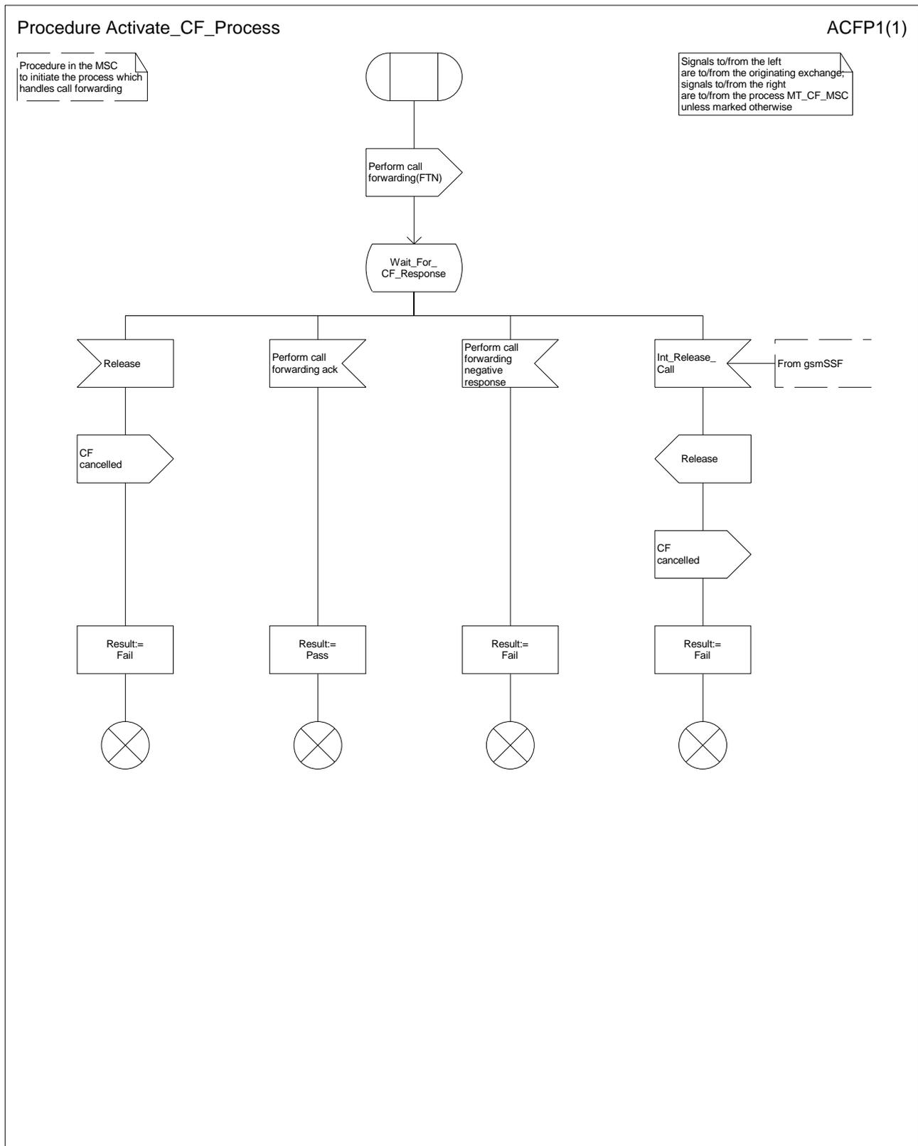
Figure 41: Procedure Activate\_Call\_Forwarding\_Process
