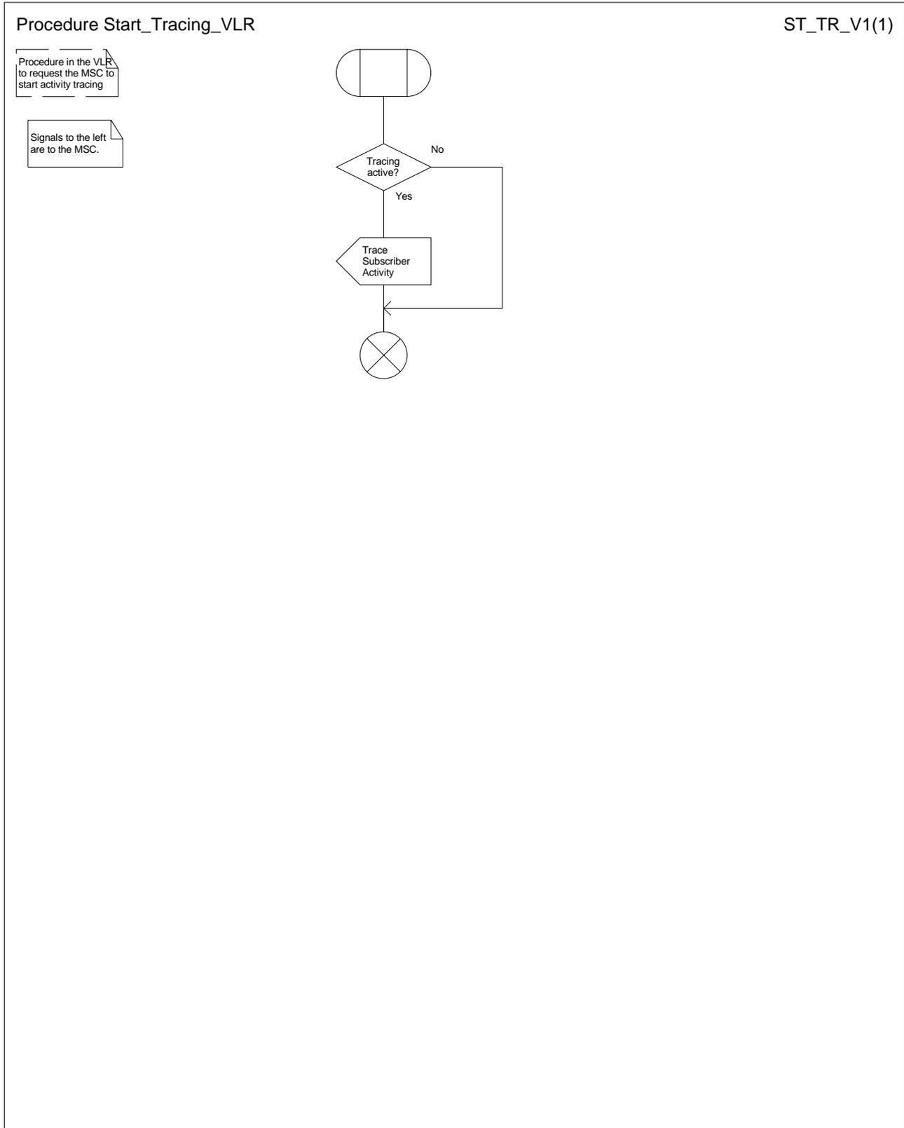
Figure 26: Procedure Start\_Tracing\_VLR
