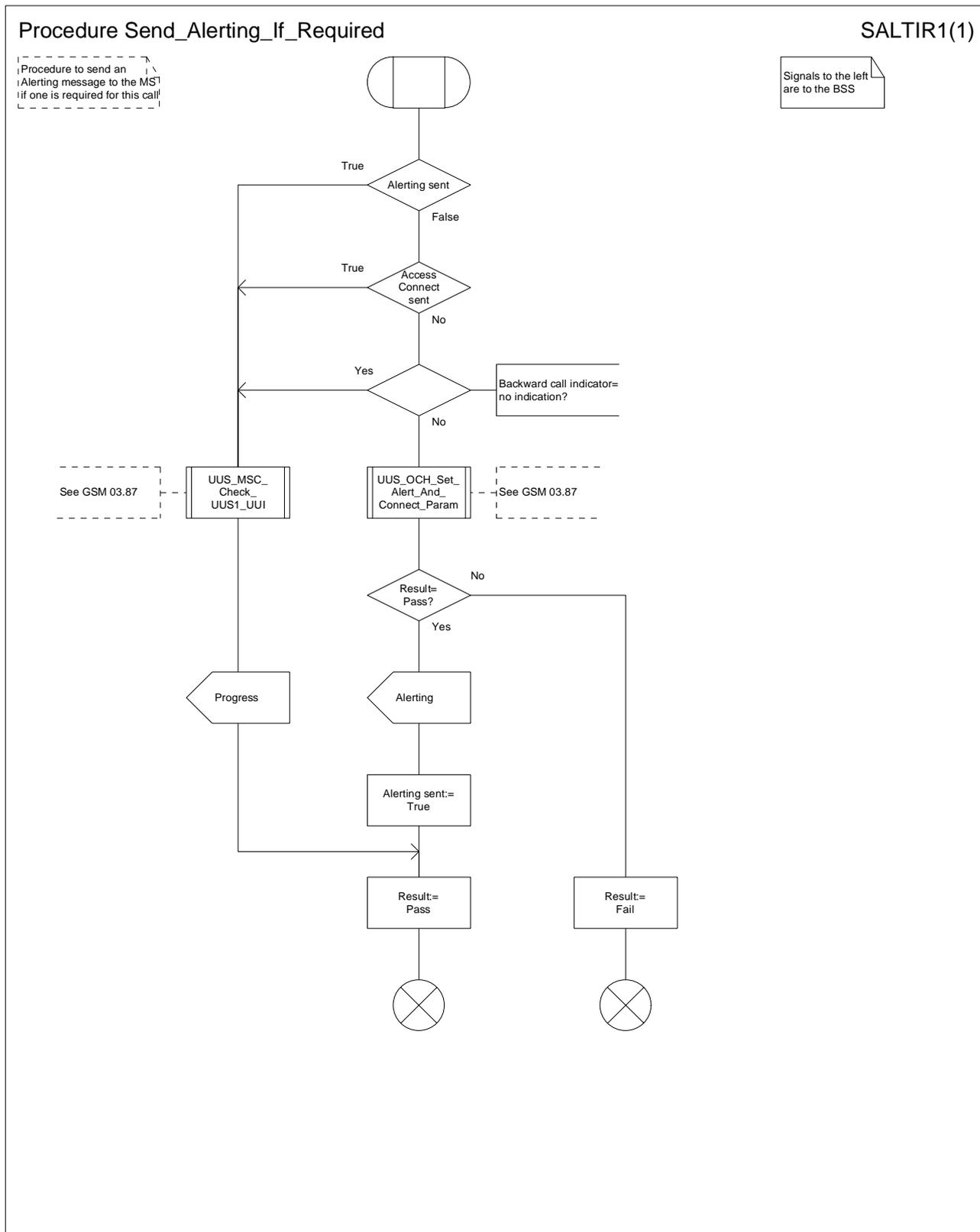
Figure 15: Procedure Send\_Alerting\_If\_Required
