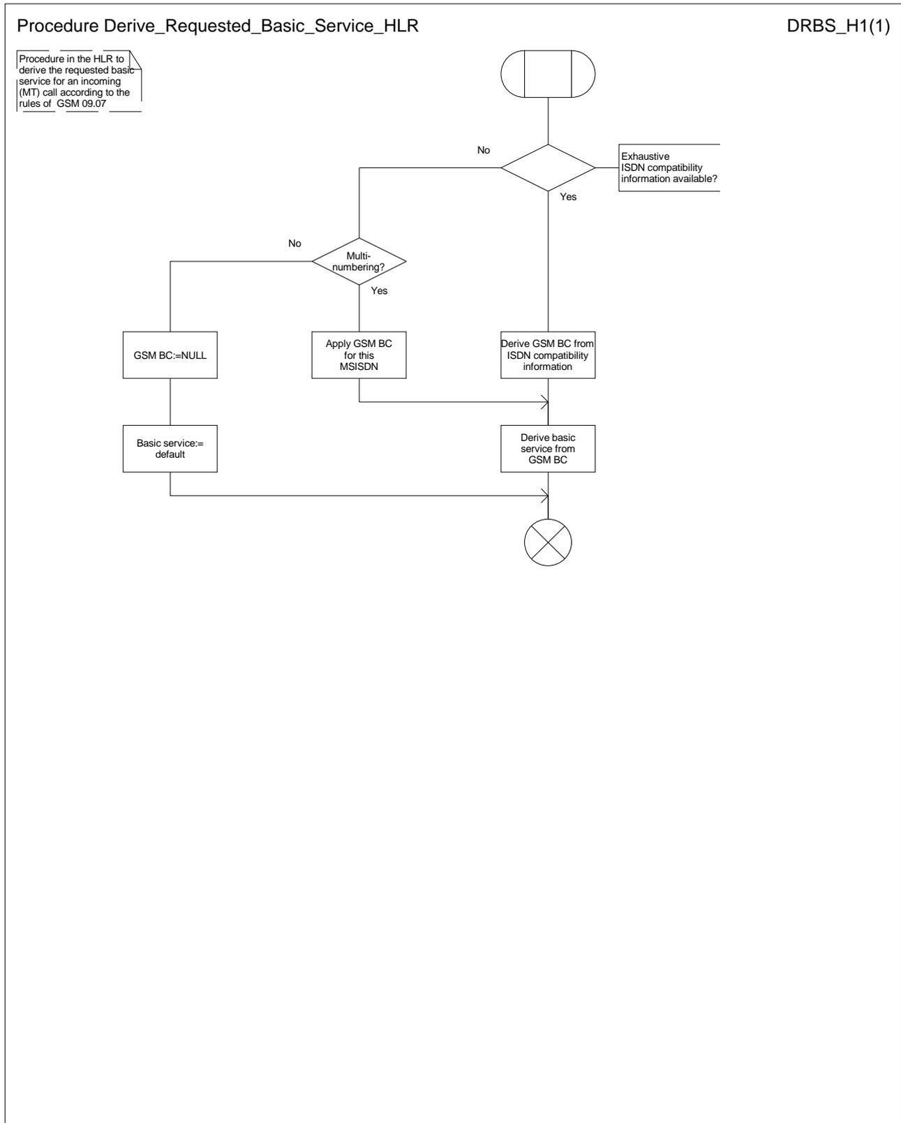
Figure 49: Procedure Derive\_Requested\_Basic\_Service\_HLR
