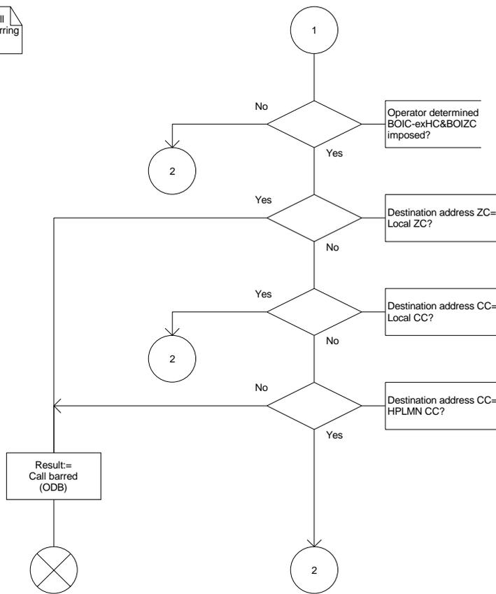
Figure 34b: Procedure Check\_OG\_Barring (sheet 2)
