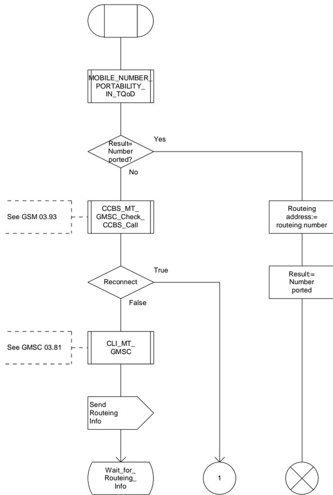
Figure 36a: Procedure Obtain\_Routeing\_Address (sheet 1)
