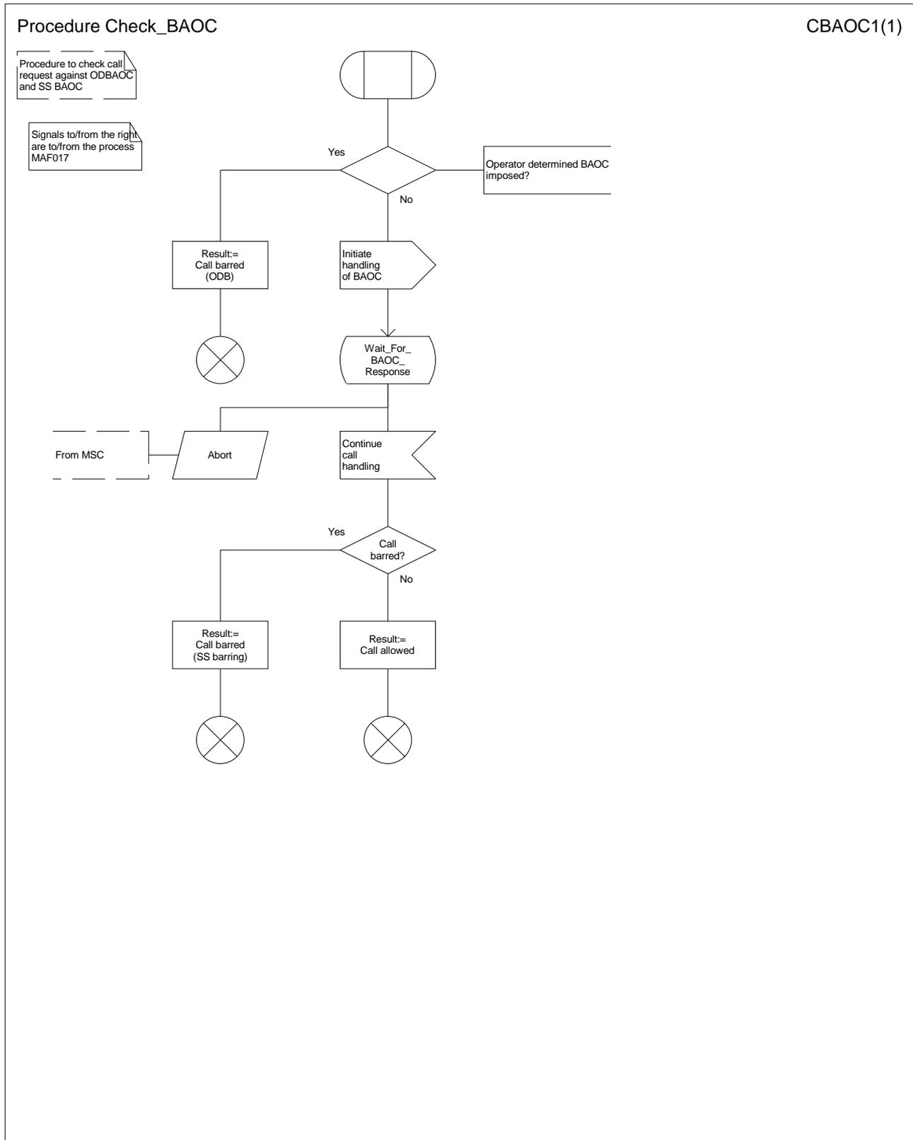
Figure 30: Procedure Check\_BAOC
