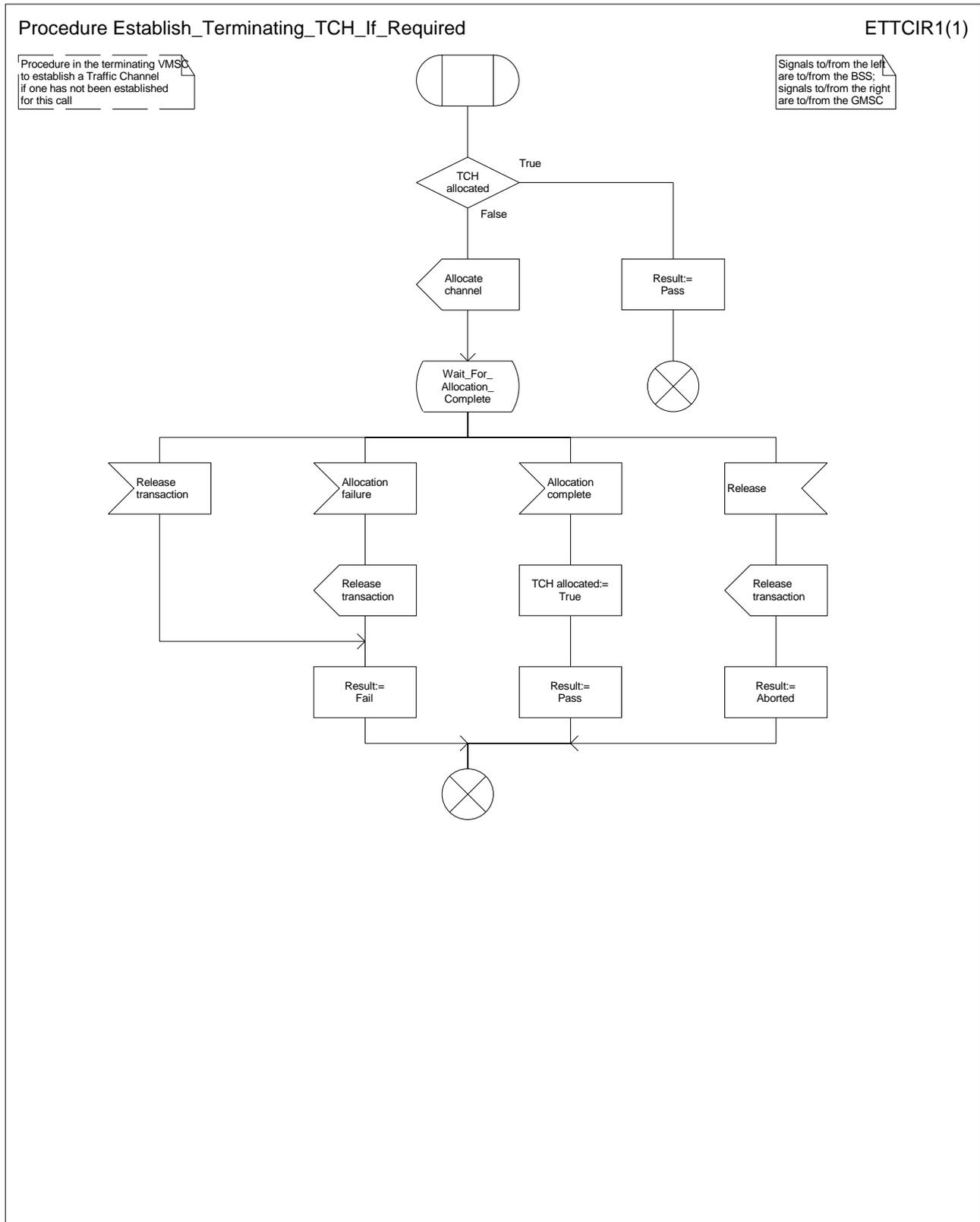
Figure 66: Procedure Establish\_Terminating\_TCH\_If\_Required
