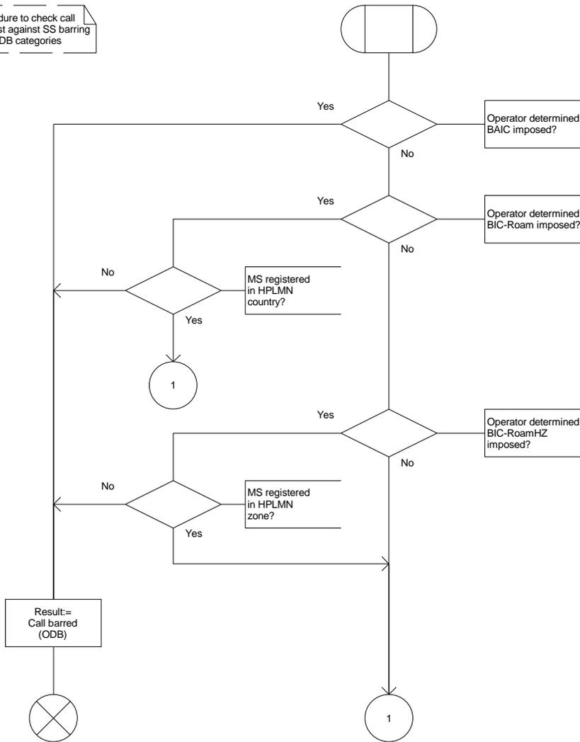
Figure 50a: Procedure Check\_IC\_Barring (sheet 1)
