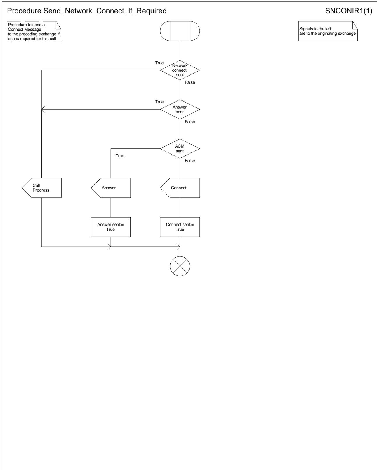
Figure 39: Procedure Send\_Network\_Connect\_If\_Required
