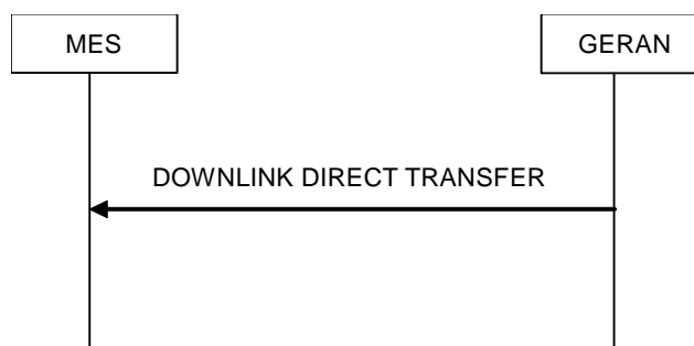
Figure 7.17.2.0.1: Downlink Direct transfer, normal flow
