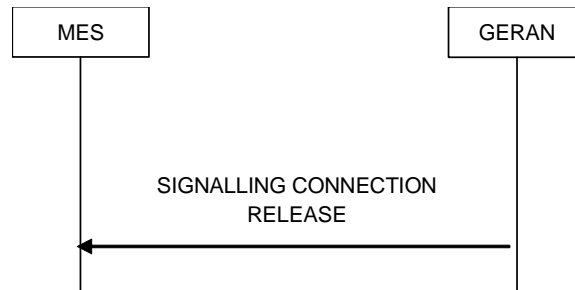
Figure 7.15.1.1.1: Signalling Connection Release procedure, normal case
