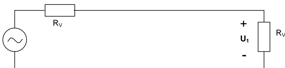
Figure F.1: Voltage across the load
