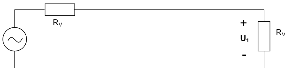
Figure ZC.1: Voltage across the load
