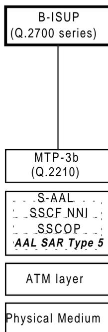
Figure 5.3: Protocol stack at the NNI.easi interface
