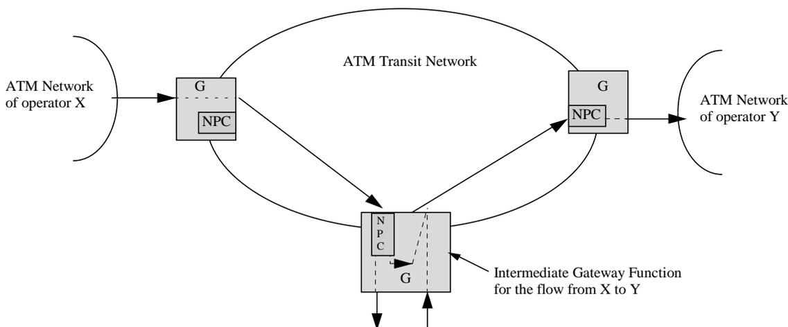
**Figure 5.1: Location of NPC functions in the ATM Transit Network**
