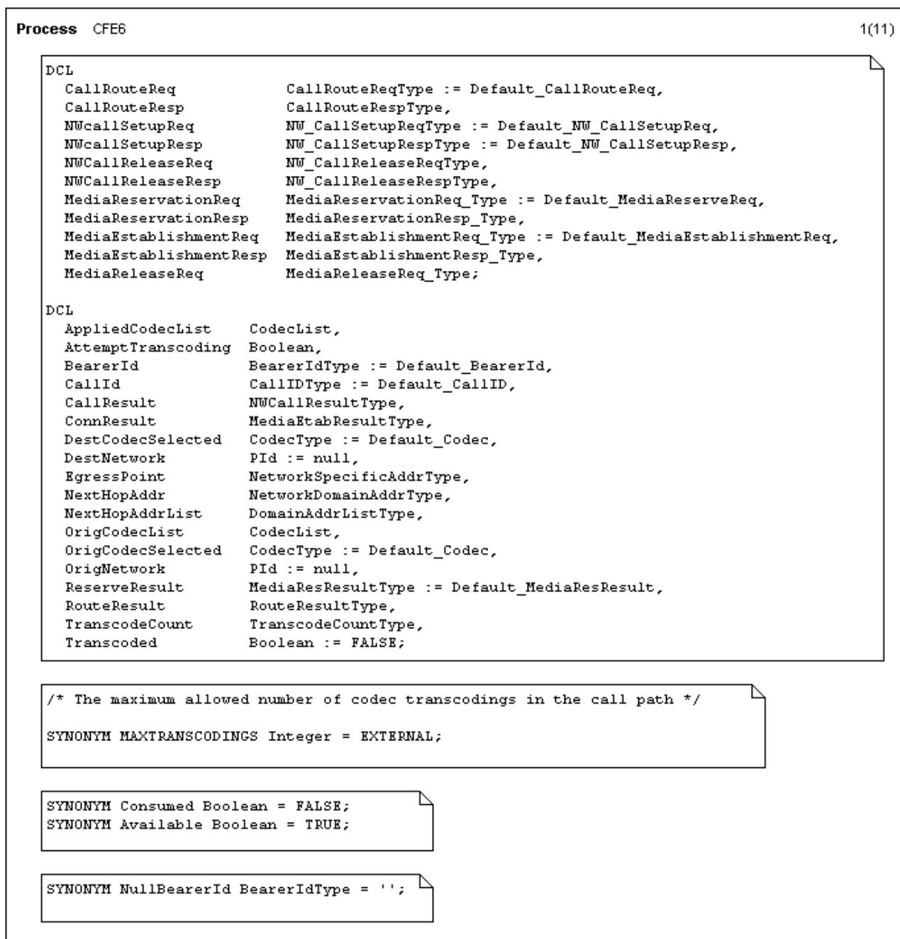
Figure 18 (sheet 1 of 11): SDL process diagram for functional entity CFE6 INC
