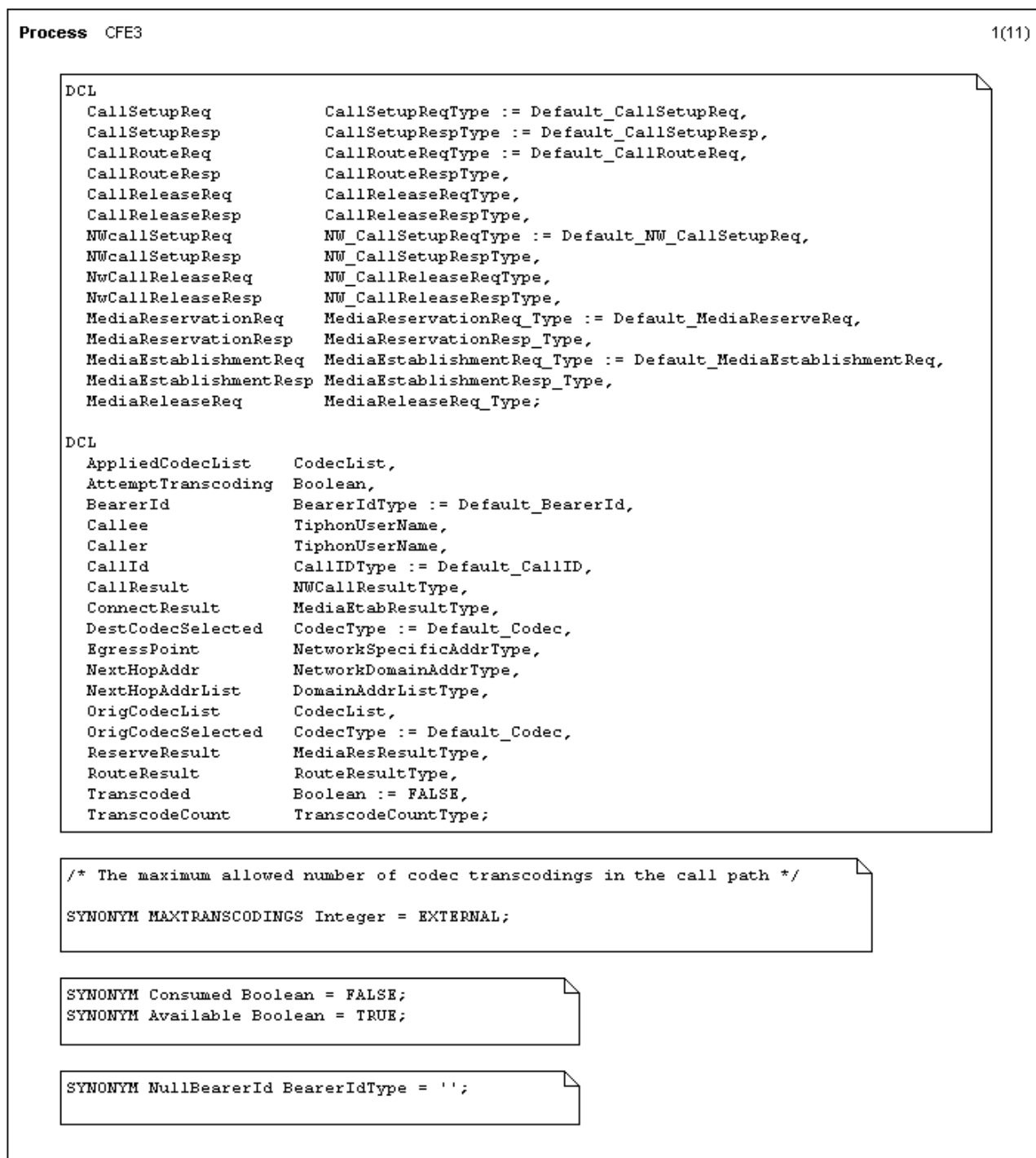
Figure 15 (sheet 1 of 11): SDL process diagram for functional entity CFE3 ONC
