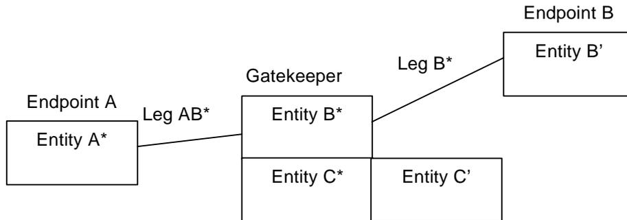
**Figure 10: H.450.2 single step call transfer model – single gatekeeper involved on behalf of endpoint B and endpoint C**
