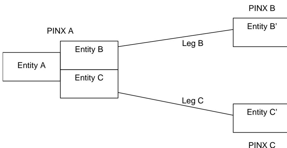
**Figure 2: Call transfer by join model for QSIG**
