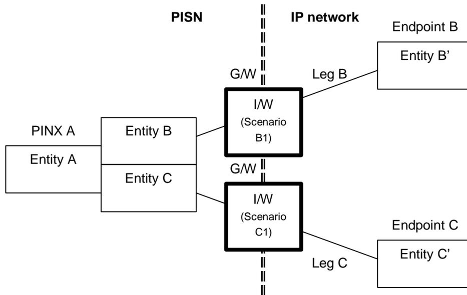
**Figure 11: Interworking – transfer by join in a PISN**
