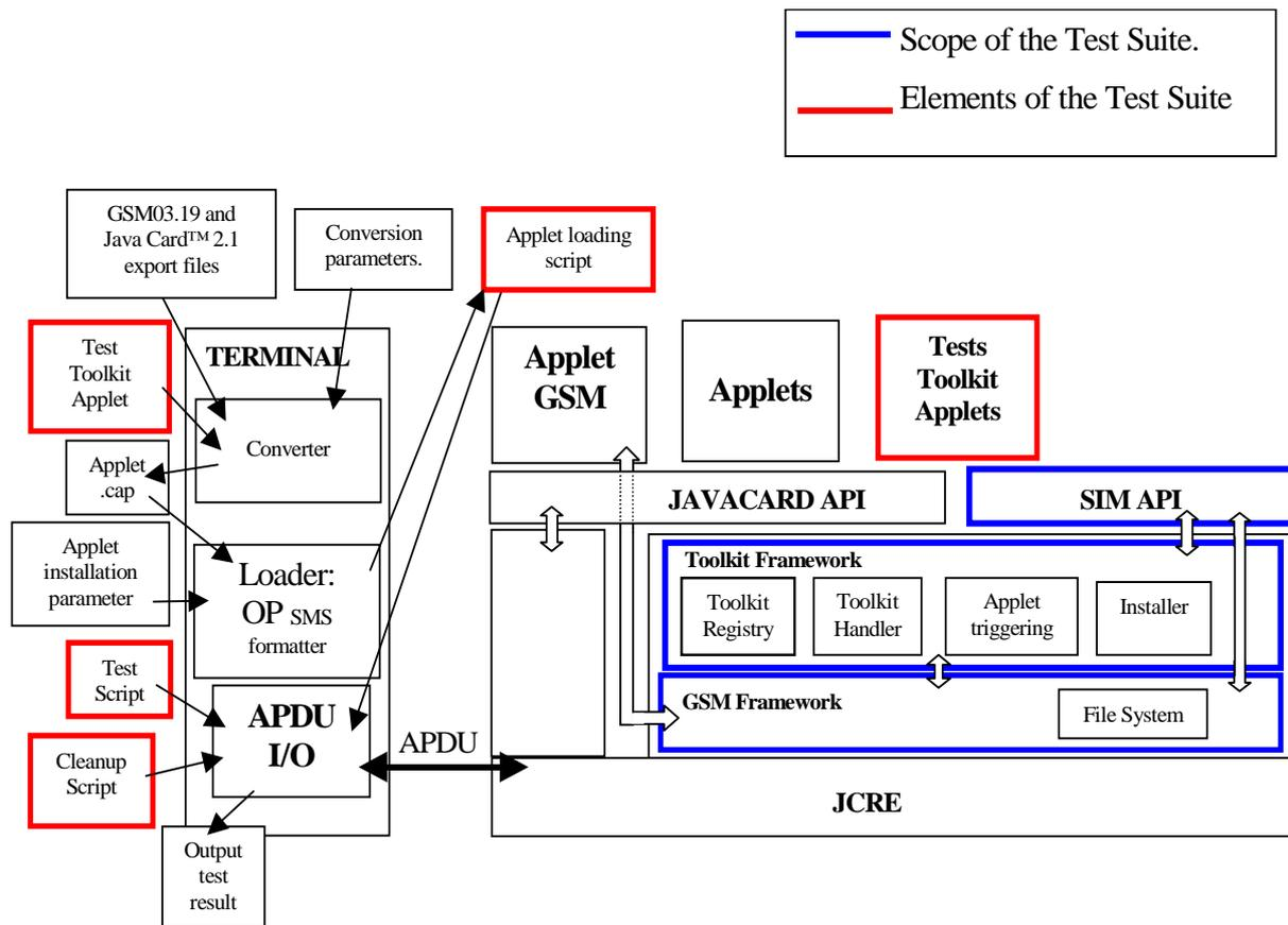
NOTE: This diagram shows the test architecture required to test interoperability at both API and bytecode level. The latter is currently not included in the present document. The diagram is for information.
