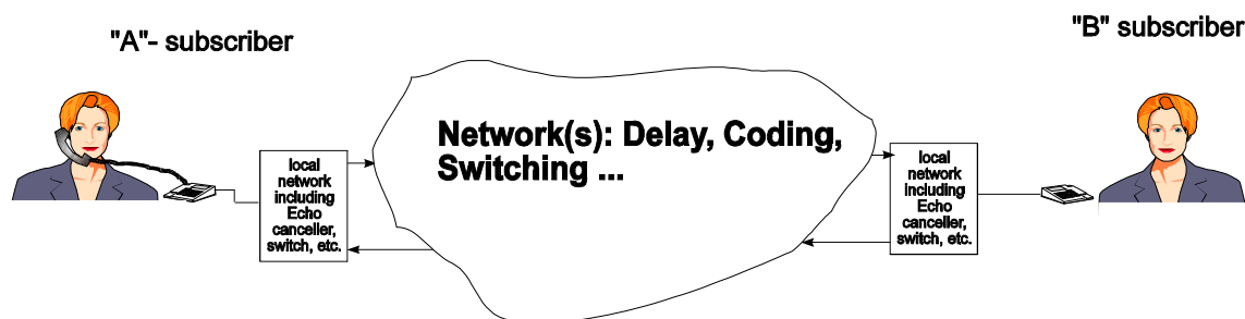
Figure D.1: Typical test set-up for determining the speech transmission quality from end to end by subjective evaluation of the speech quality relevant parameters (example for handset/hands-free communication)
