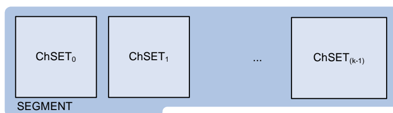
Figure 8-3: Segment with Encoded and Packed Channel Sets
