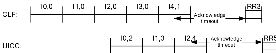
Figure 10.13: Piggybacking and timed acknowledgement
