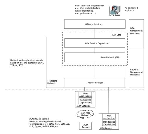
Figure A.1: M2M high level system overview
