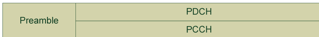
Figure 4.3: The Up-Link Burst and its constituent parts
