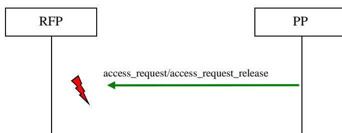
Figure 27: Packet Mode Connection setup fail (access message wrong)
