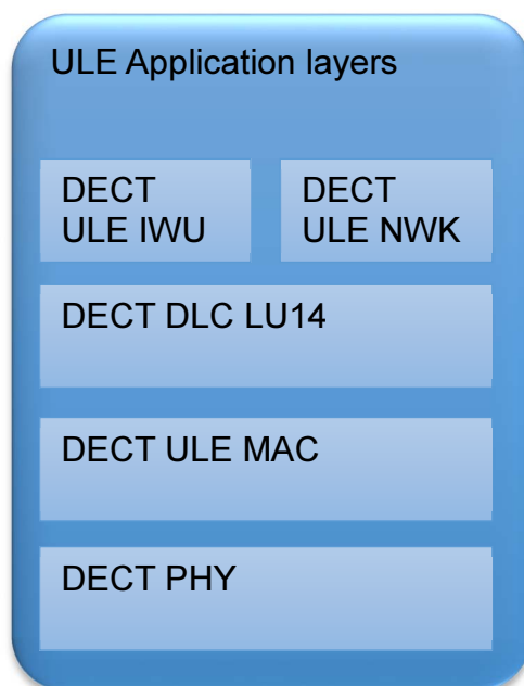
Figure 4: Reference model of the ULE U-plane and C-plane
