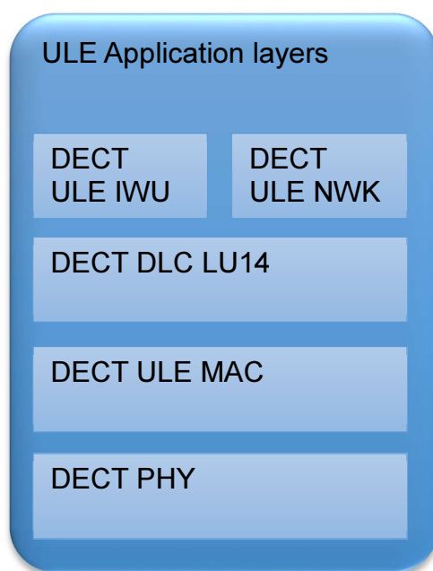
Figure 4: Reference model of the ULE U-plane and C-plane
