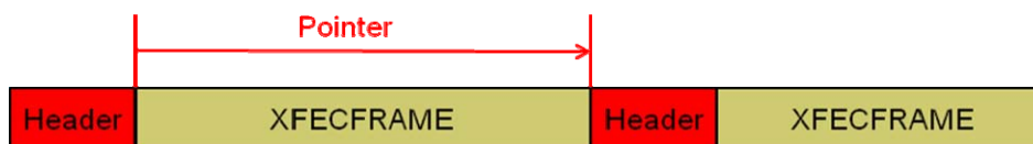
Figure 62: Calculation of the position of the following Data Slice Packet Header by means of the header data
