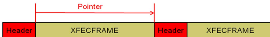
Figure 76: Calculation of the position of the following Data Slice Packet Header by means of the header data
