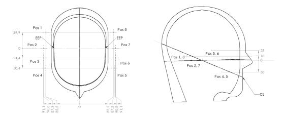
Figure 4: Positions of the recording microphones for binaural applications
