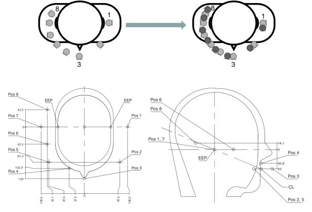
Figure 1: Positions of the recording microphones
