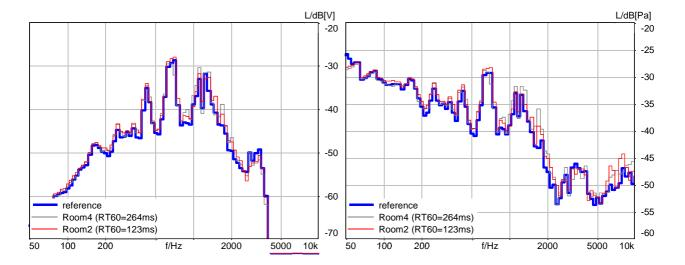
NOTE: The left diagram shows the sending signal of the mobile phone whereas the right diagram shows the measured signal using a measurement microphone at the hands-free main microphone position.
