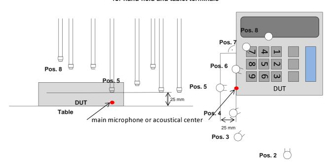
Figure 3: Positions of the recording microphones in a hands-free setup for desktop operated hands-free terminals
