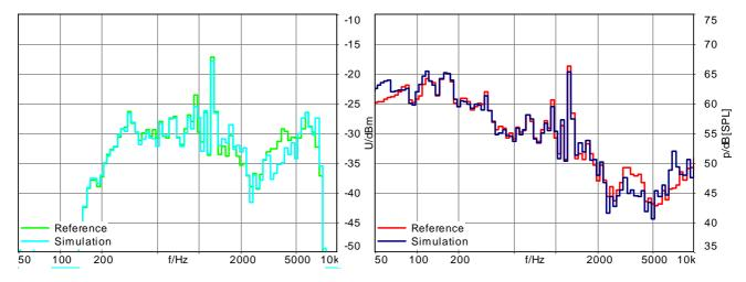
Figure 21: Desktop phone equalization - Comparison of 12<sup>th</sup> octave spectra of reference recording vs. simulated recording for the "mix"-signal
