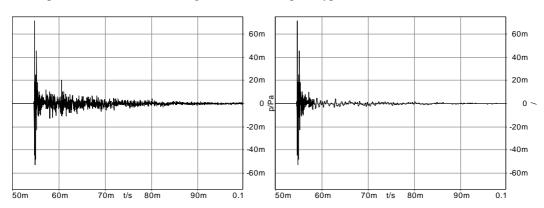
Figure 8: Original (measured) impulse response (left) and processed impulse response (right)
