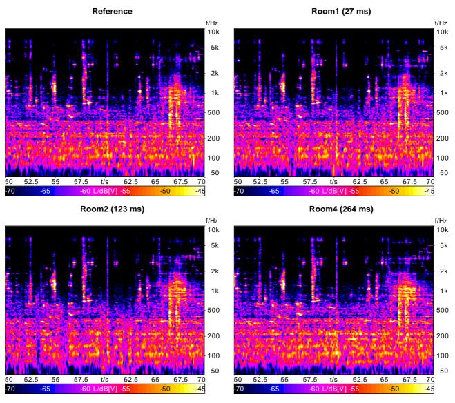
NOTE: The top left diagram shows the spectrum vs. time analysis of the reference recording.
