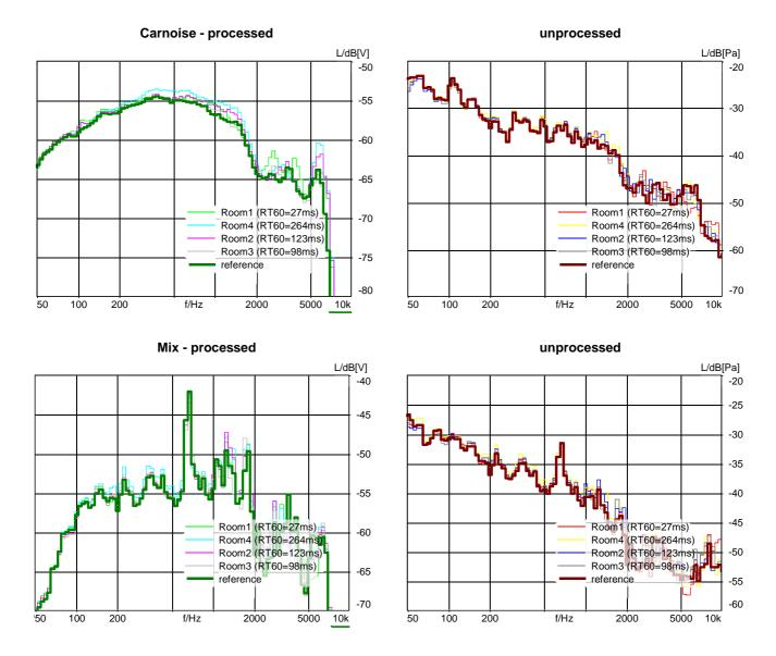
Figure 16: Phone1, handset mode, Comparison of 12<sup>th</sup> octave spectra for carnoise and mix-signal in different rooms (processed on the left, unprocessed on the right)
