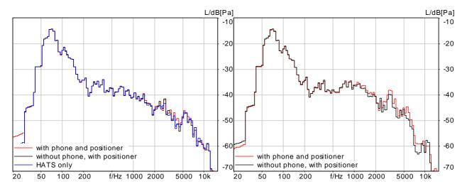
NOTE: The left diagram shows the deviations at the main microphone location whereas the right diagram shows the deviations at the rear microphone location.
