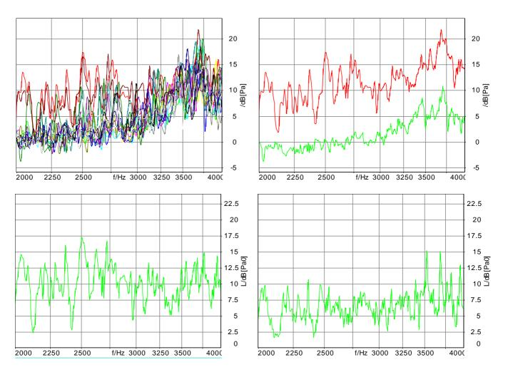
NOTE: Top left: absolute error before optimization at 16 microphone positions; top right: minimum and maximum of error; bottom left: error range before optimization (difference between minimum and maximum);
