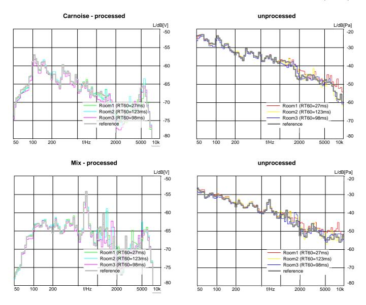
Figure 17: Phone2, handset mode, Comparison of 12<sup>th</sup> octave spectra for carnoise and mix-signal in different rooms (processed on the left, unprocessed on the right)
