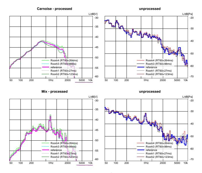
Figure 18: Phone3, handset mode, Comparison of 12<sup>th</sup> octave spectra for carnoise and mix-signal in different rooms (processed on the left, unprocessed on the right)
