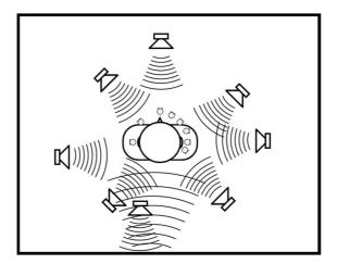
Figure 15: Setup for generating a reference sound field
