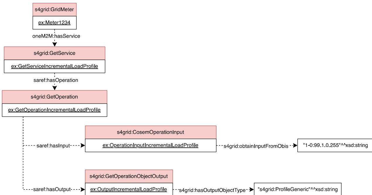
Figure 31: Example of electric grid meter get service I
