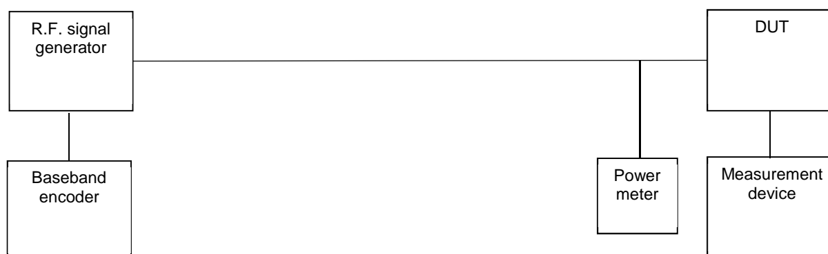
Figure 5: Conducted test set up for Gaussian sensitivity
