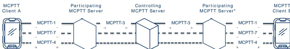
**Figure 9: CFG\_ONN\_OTT-1 Interfaces for the unicast case**
