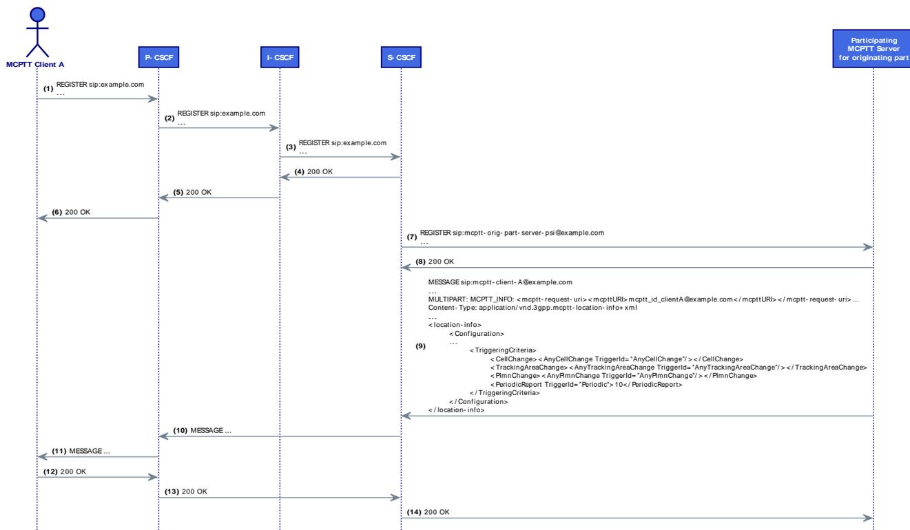
Figure 89: LOC/3PRTYREG/CONFIG/01 Message Sequence
