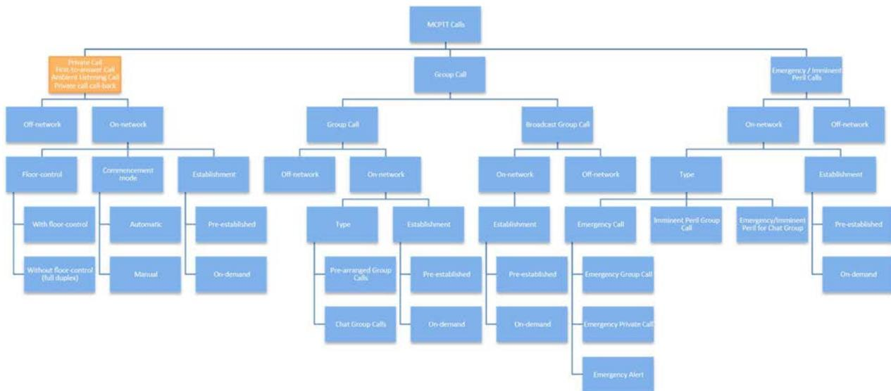
Figure 3: MCPTT call types in Release 14
