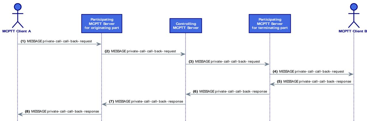
Figure 34: CONN-MCPTT/ONN/CALLBACK/SETUP/01 Message Sequence
