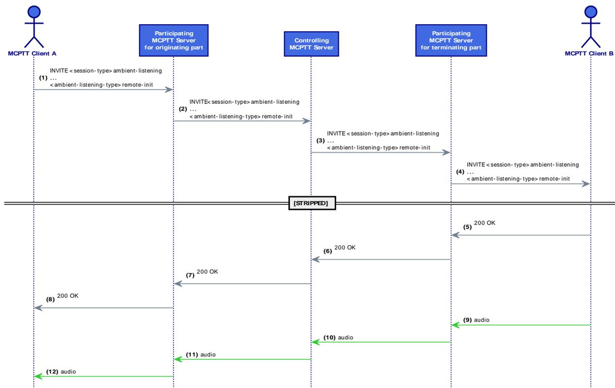
Figure 41: CONN-MCPTT/ONN/AMBIENT/ONDEM/REMOTE/01 Message Sequence
