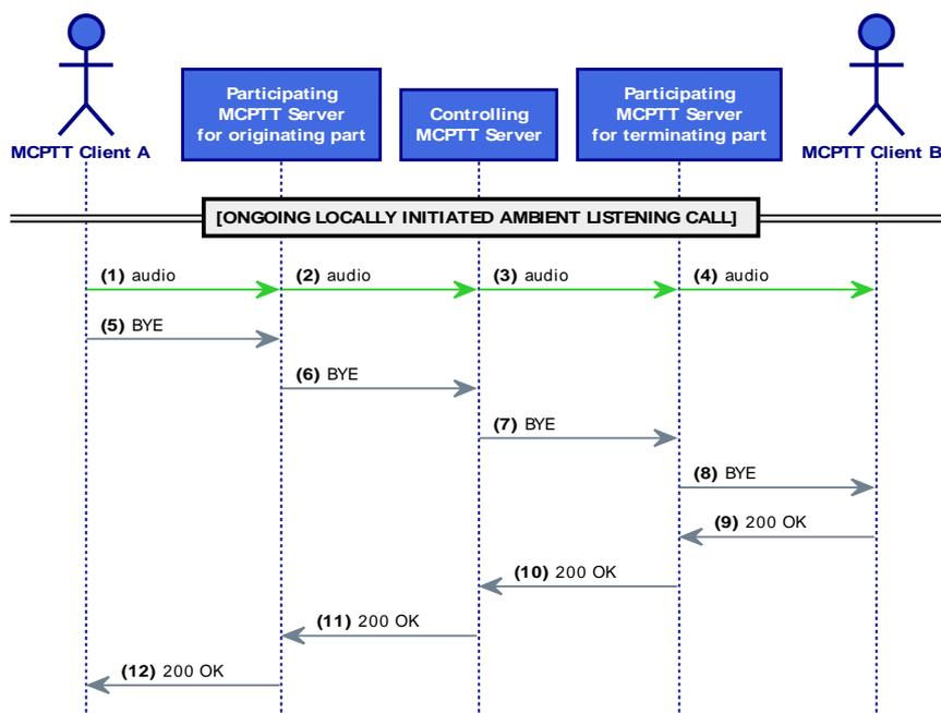
Figure 38: CONN-MCPTT/ONN/AMBIENT/ONDEM/LOCAL/02 Message Sequence
