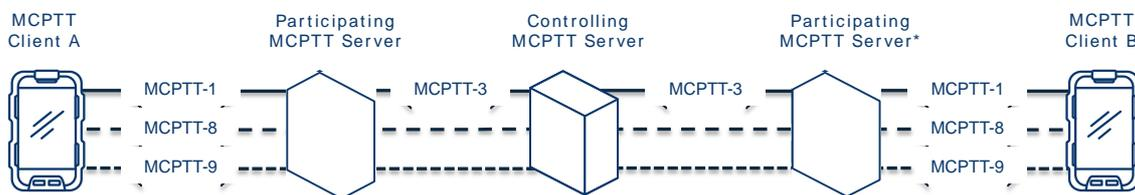
**Figure 10: CFG\_ONN\_OTT-1 Interfaces for the multicast case**
