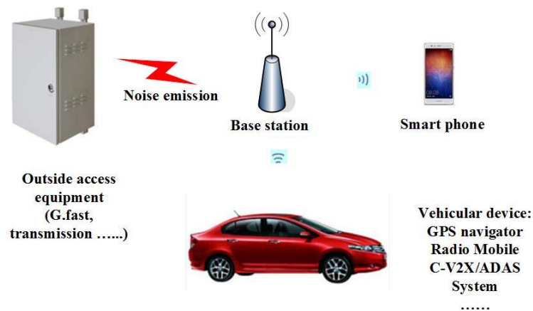
Figure 2: Disturbance to vehicles and base stations due to outside access equipment on the street
