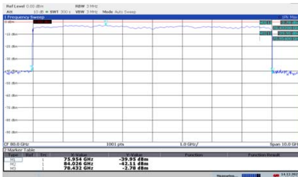
Figure B.11: TX spectrum of conducted measurement at -20 °C (source: VEGA Grieshaber KG)
