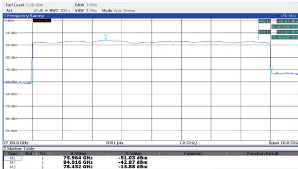
Figure B.20: TX spectrum of \frac{3}{4} " horn antenna at 0 °C (source: VEGA Grieshaber KG)
