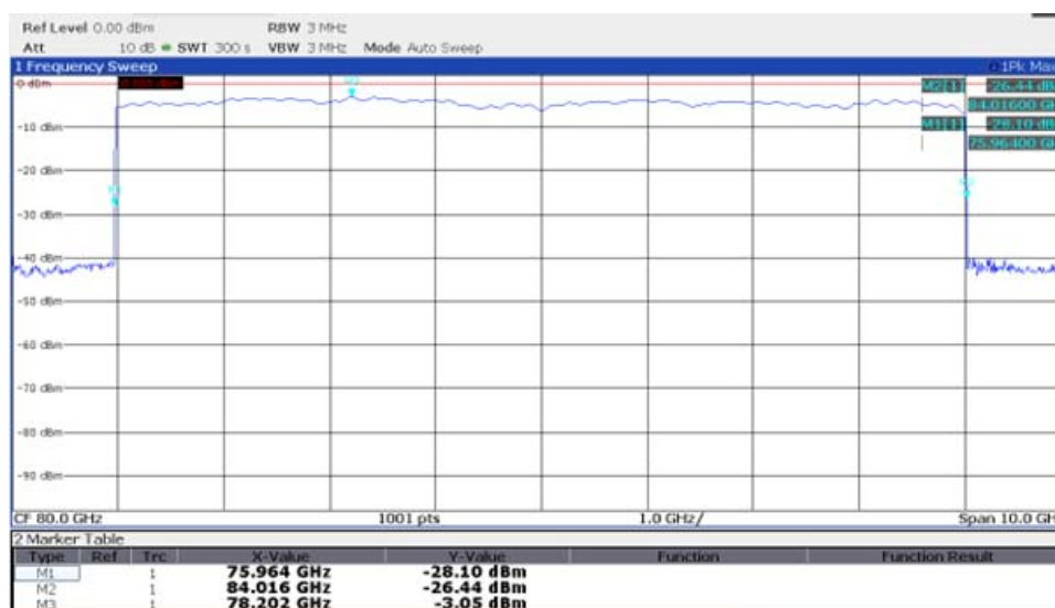
Figure B.12: TX spectrum of conducted measurement at 0 °C (source: VEGA Grieshaber KG)
