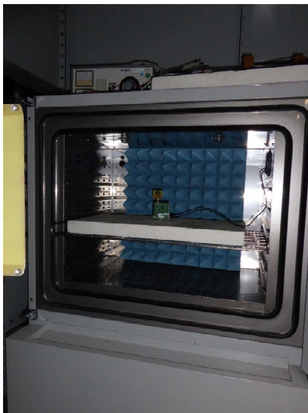
Figure B.61: Setup-photo with door opened and one absorber behind the EUT (Source: PHOENIX TESTLAB GmbH)
