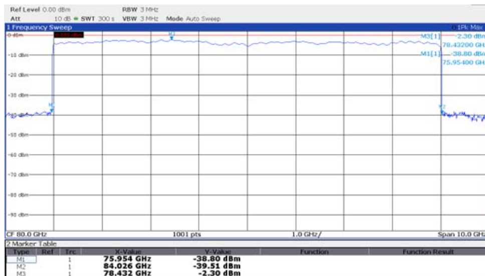
Figure B.10: TX spectrum of conducted measurement at -40 °C (source: VEGA Grieshaber KG)
