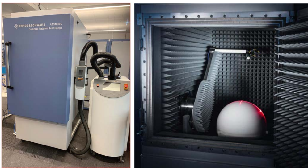
Figure 2: OTA chamber with the thermal compartment (left side) and the inside of the OTA chamber with the RF transparent compartment (right side) (source: ROHDE & SCHWARZ GmbH & Co.KG)
