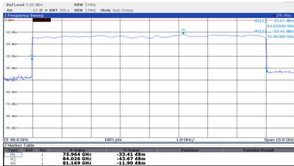
Figure B.26: TX spectrum of 3" plastic horn antenna at -40 °C (source: VEGA Grieshaber KG)
