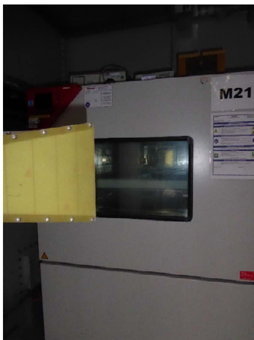
Figure B.54: Setup with measurement through window of temperature chamber (Source: PHOENIX TESTLAB GmbH)
