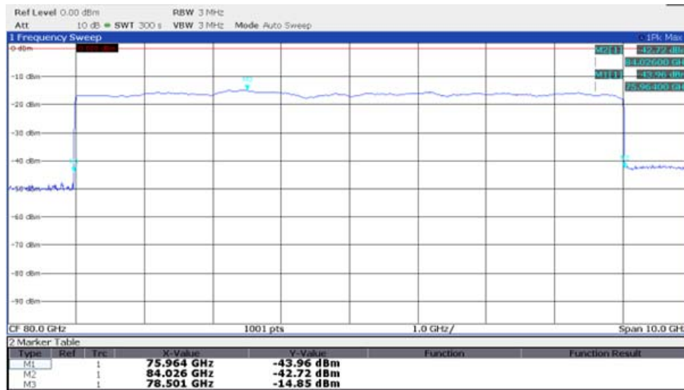
Figure B.18: TX spectrum of \frac{3}{4} " horn antenna at -40 °C (source: VEGA Grieshaber KG)
