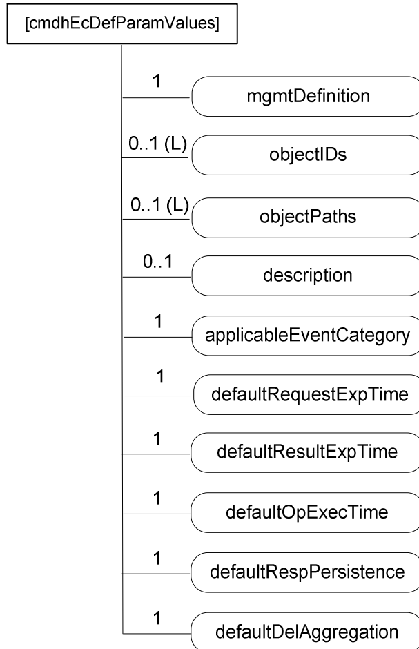
Figure D.12.4-1: Structure of [cmdhEcDefParamValues] resource
