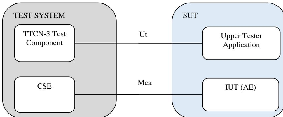
Figure 5.2.1-1: AE test configuration
