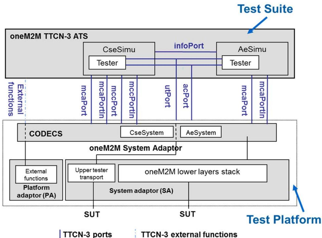
Figure 5.3-2: oneM2M Test Architecture
