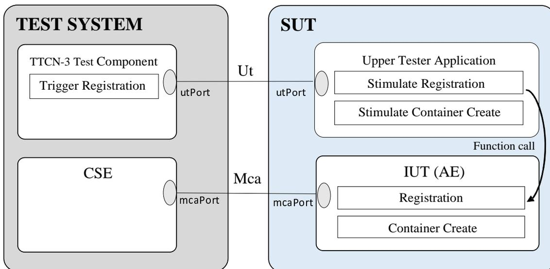
Figure 5.4.2.1-1: Example of automated AE test using Ut interface
