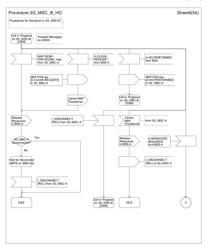
Figure 44 (sheet 6 of 54): Handover control procedure in 3G\_MSC-B
