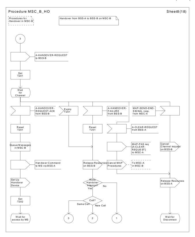
Figure 42 (Sheet 8 of 18): Handover control procedure in MSC-B
