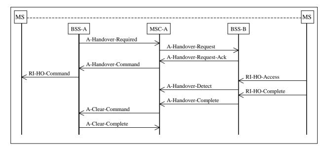
Figure 7: Basic External Intra-MSC Handover Procedure
