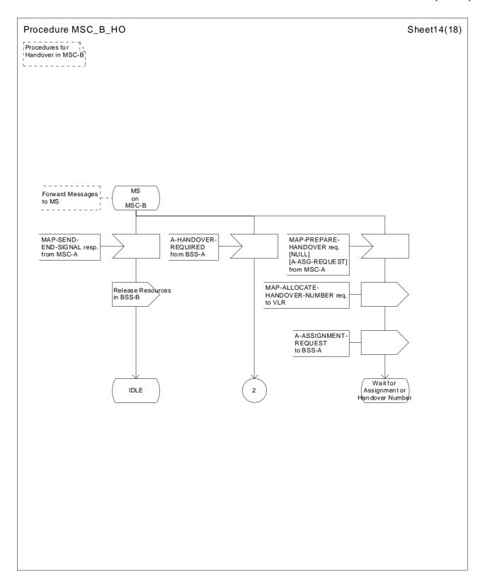
Figure 42 (Sheet 14 of 18): Handover control procedure in MSC-B
