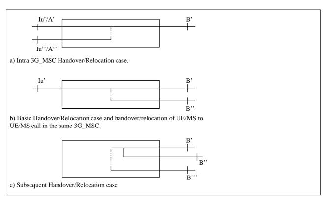
NOTE: In a) and b) Iu" is released after handover/relocation; In c) B"" is released after handover/relocation.
