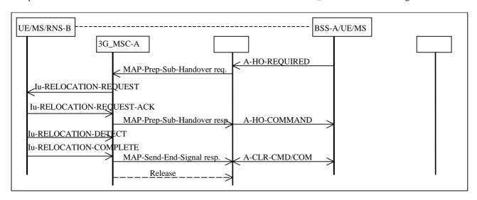
Figure 26: Subsequent GSM to UMTS handover procedure i): successful handover from MSC-B to 3G\_MSC-A using a circuit connection
