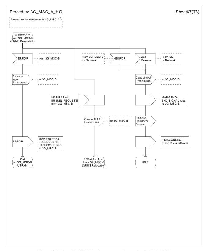
Figure 43 (sheet 67 of 78): Handover control procedure in 3G\_MSC-A
