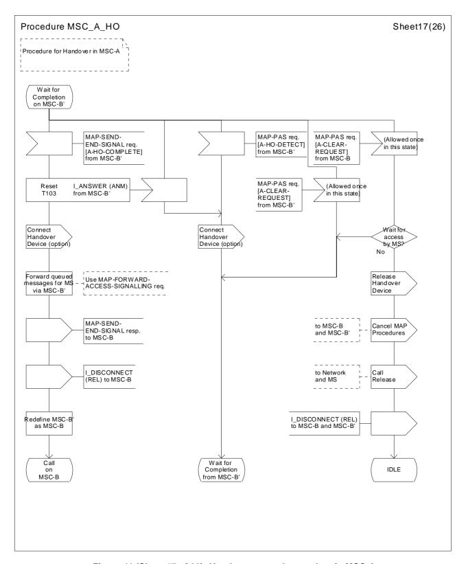
Figure 41 (Sheet 17 of 26): Handover control procedure in MSC-A
