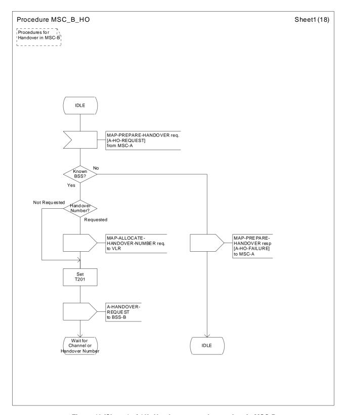
Figure 42 (Sheet 1 of 18): Handover control procedure in MSC-B
