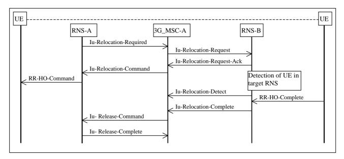
Figure 11 Basic intra-3G\_MSC SRNS Relocation Procedure combined with hard change of radio resources (Hard Handover with switch in the Core Network)
