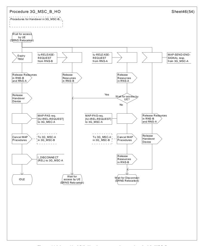
Figure 44 (sheet 46 of 54): Handover control procedure in 3G\_MSC-B
