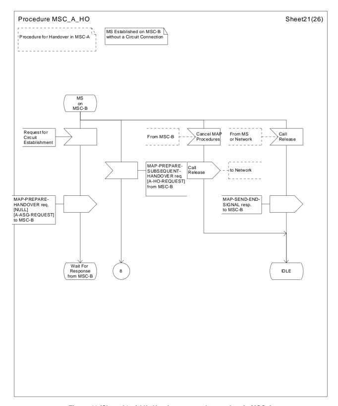
Figure 41 (Sheet 21 of 26): Handover control procedure in MSC-A
