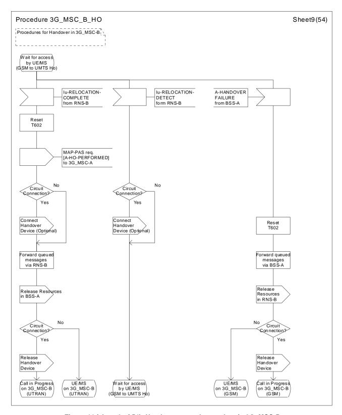
Figure 44 (sheet 9 of 54): Handover control procedure in 3G\_MSC-B
