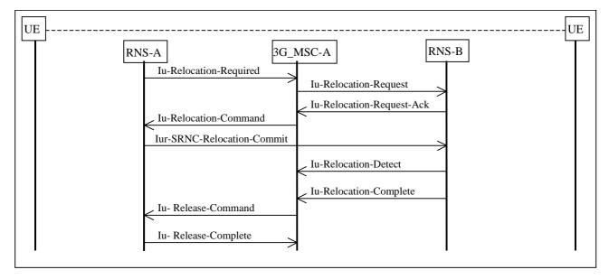
Figure 10 Basic intra-3G MSC SRNS Relocation Procedure
