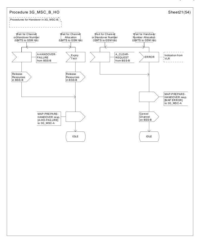
Figure 44 (sheet 21 of 54): Handover control procedure in 3G\_MSC-B
