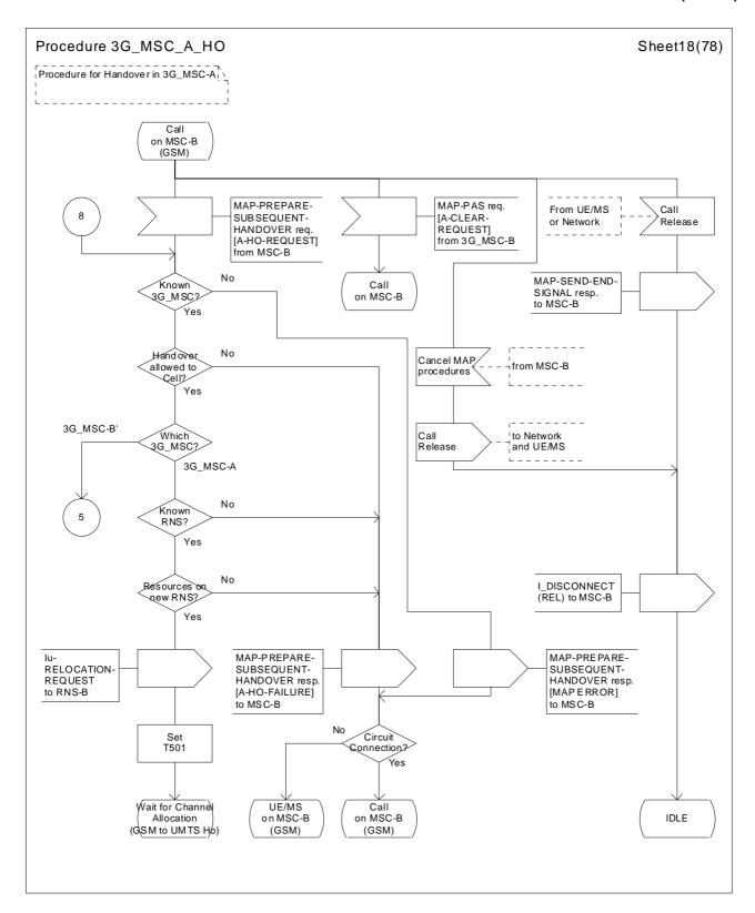
Figure 43 (sheet 18 of 78): Handover control procedure in 3G\_MSC-A
