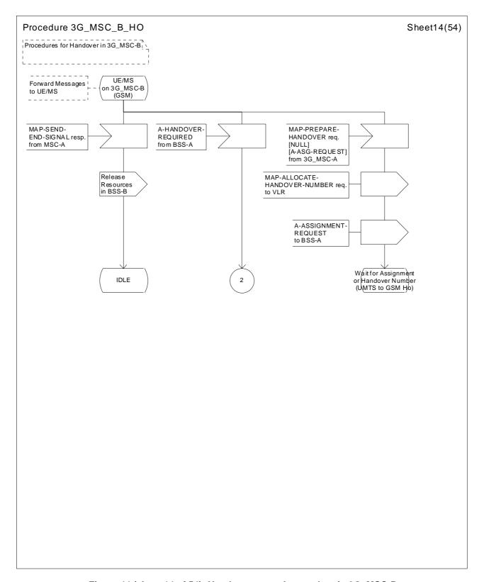
Figure 44 (sheet 14 of 54): Handover control procedure in 3G\_MSC-B
