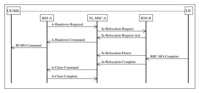
Figure 9: Basic External Intra-3G\_MSC GSM to UMTS Handover Procedure
