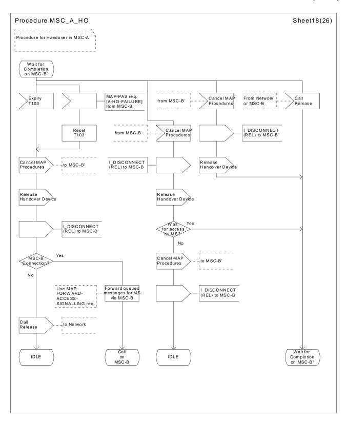
Figure 41 (Sheet 18 of 26): Handover control procedure in MSC-A
