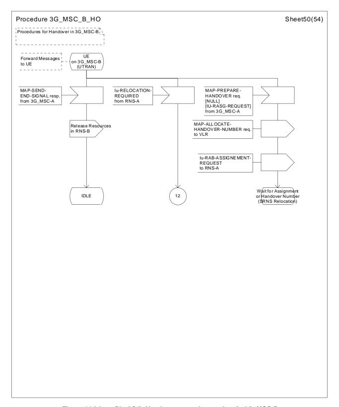
Figure 44 (sheet 50 of 54): Handover control procedure in 3G\_MSC-B
