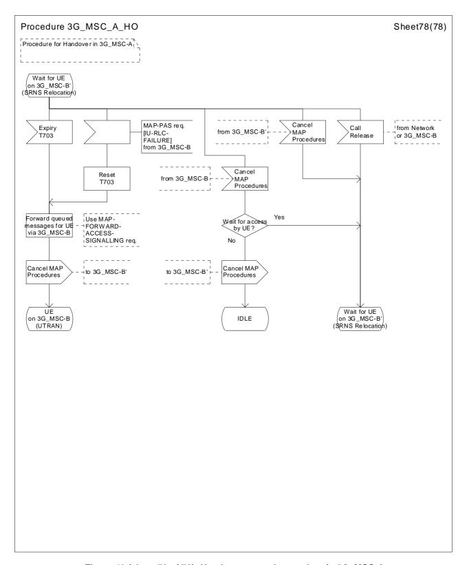
Figure 43 (sheet 78 of 78): Handover control procedure in 3G\_MSC-A
