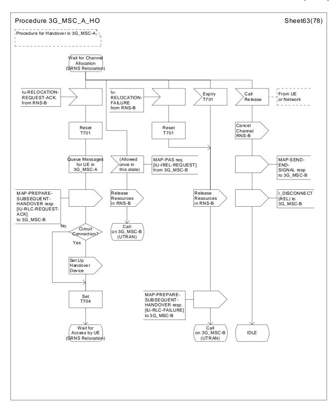
Figure 43 (sheet 63 of 78): Handover control procedure in 3G\_MSC-A
