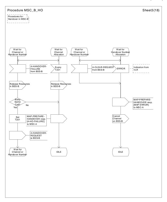
Figure 42 (Sheet 3 of 18): Handover control procedure in MSC-B
