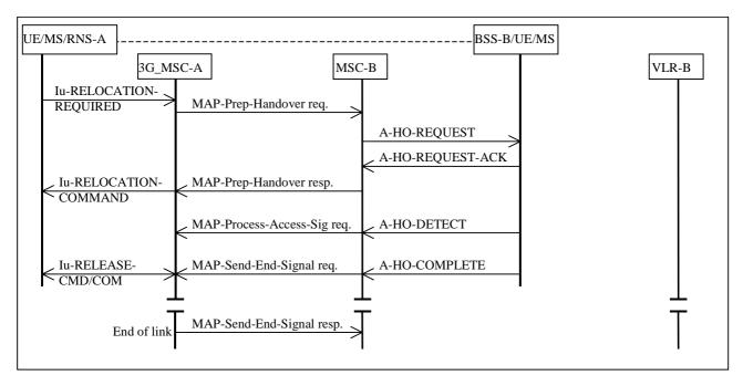
Figure 19: Basic UMTS to GSM Handover Procedure without circuit connection
