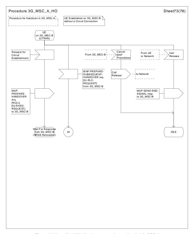
Figure 43 (sheet 73 of 78): Handover control procedure in 3G\_MSC-A
