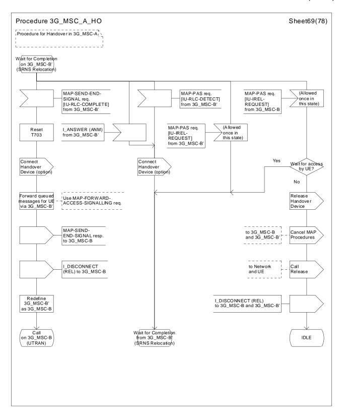
Figure 43 (sheet 69 of 78): Handover control procedure in 3G\_MSC-A
