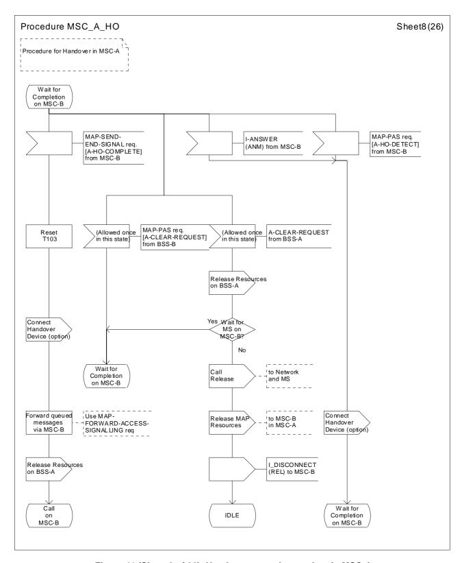
Figure 41 (Sheet 8 of 26): Handover control procedure in MSC-A
