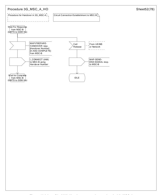
Figure 43 (sheet 52 of 78): Handover control procedure in 3G\_MSC-A
