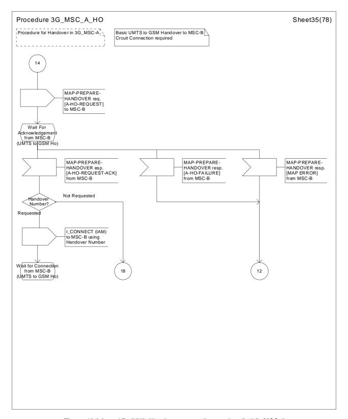
Figure 43 (sheet 35 of 78): Handover control procedure in 3G\_MSC-A
