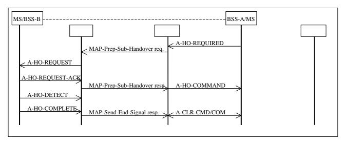
Figure 16: Subsequent handover procedure i): Successful handover from MSC-B to MSC-A not requiring a circuit connection
