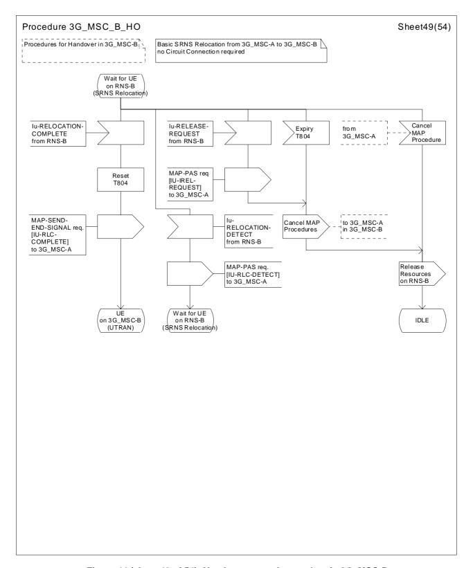
Figure 44 (sheet 49 of 54): Handover control procedure in 3G\_MSC-B
