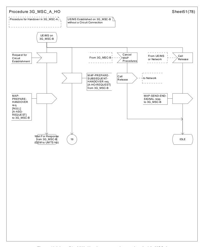
Figure 43 (sheet 51 of 78): Handover control procedure in 3G\_MSC-A
