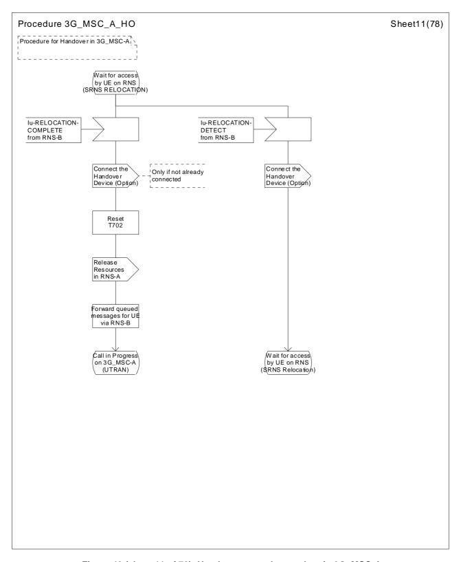
Figure 43 (sheet 11 of 78): Handover control procedure in 3G\_MSC-A
