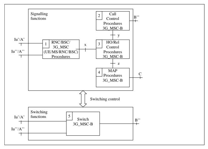
Figure 6: Functional composition of 3G\_MSC-B for supporting handover/relocation
