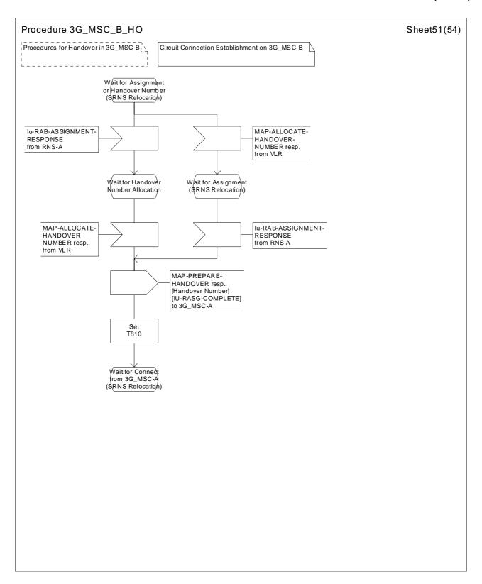
Figure 44 (sheet 51 of 54): Handover control procedure in 3G\_MSC-B
