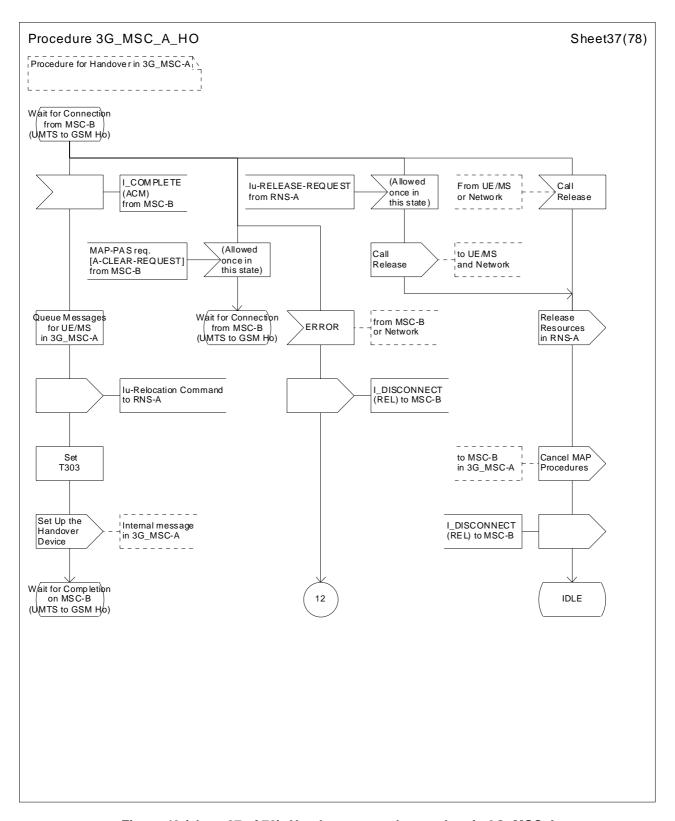
Figure 43 (sheet 37 of 78): Handover control procedure in 3G\_MSC-A
