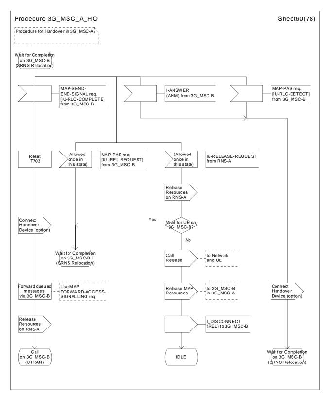
Figure 43 (sheet 60 of 78): Handover control procedure in 3G\_MSC-A
