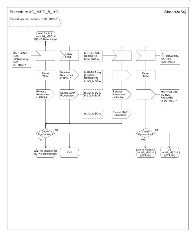
Figure 44 (sheet 48 of 54): Handover control procedure in 3G\_MSC-B
