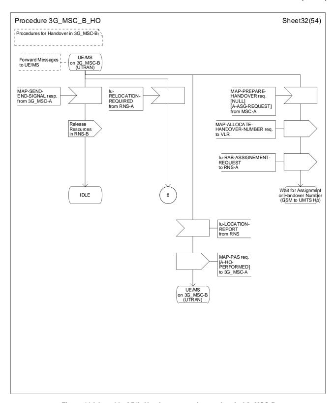
Figure 44 (sheet 32 of 54): Handover control procedure in 3G\_MSC-B
