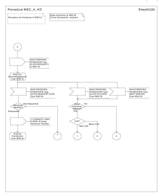
Figure 41 (Sheet 5 of 26): Handover control procedure in MSC-A
