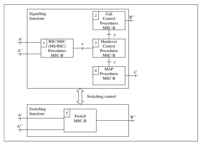
Figure 3: Functional composition of MSC-B for supporting handover
