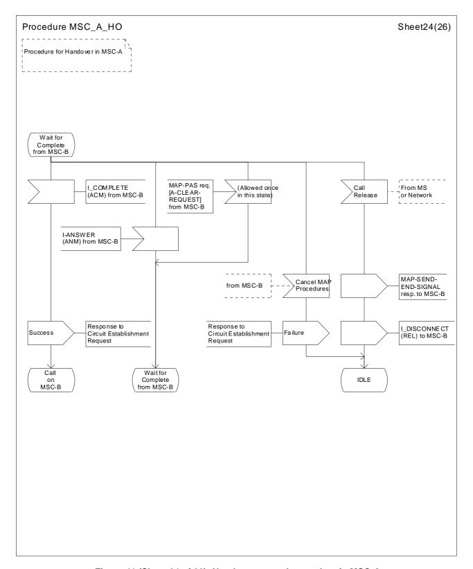
Figure 41 (Sheet 24 of 26): Handover control procedure in MSC-A
