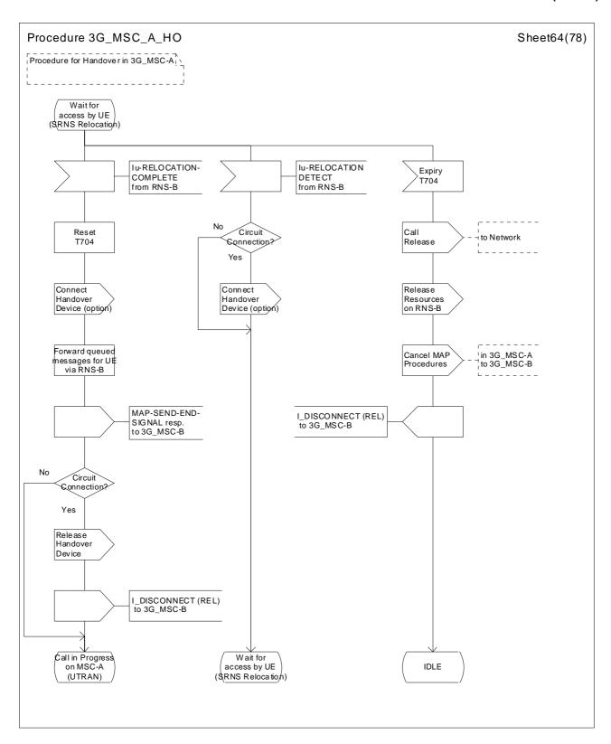
Figure 43 (sheet 64 of 78): Handover control procedure in 3G\_MSC-A
