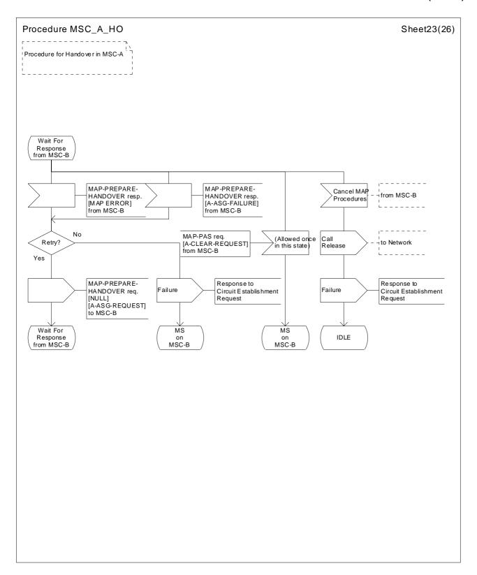
Figure 41 (Sheet 23 of 26): Handover control procedure in MSC-A
