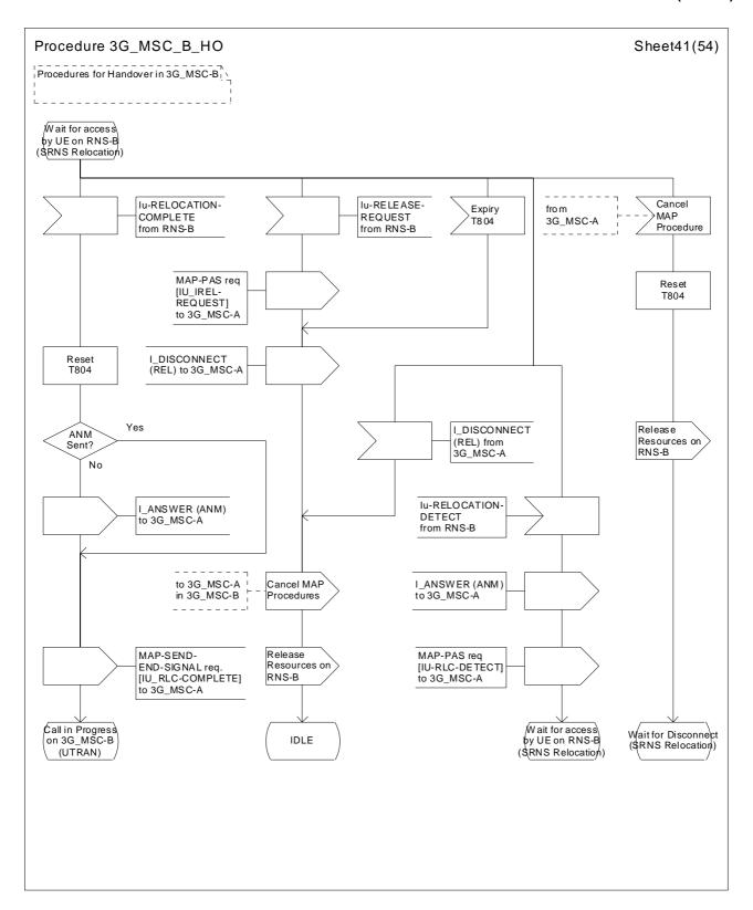
Figure 44 (sheet 41 of 54): Handover control procedure in 3G\_MSC-B
