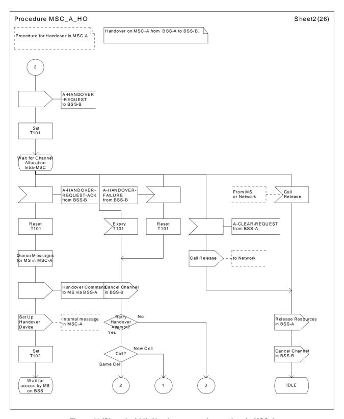
Figure 41 (Sheet 2 of 26): Handover control procedure in MSC-A
