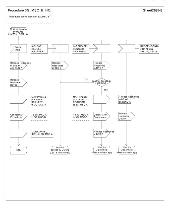
Figure 44 (sheet 28 of 54): Handover control procedure in 3G\_MSC-B
