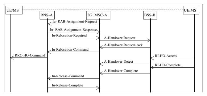
Figure 40b: Example of a Directed Retry Intra-3G\_MSC UMTS to GSM Handover Procedure
