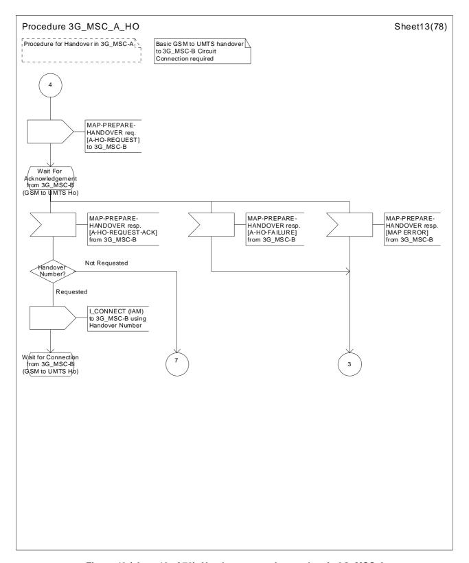
Figure 43 (sheet 13 of 78): Handover control procedure in 3G\_MSC-A
