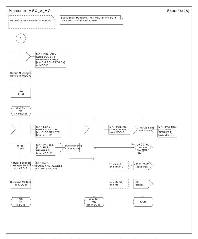
Figure 41 (Sheet 25 of 26): Handover control procedure in MSC-A
