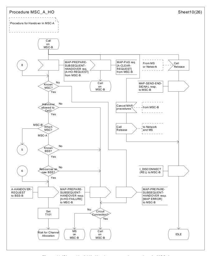
Figure 41 (Sheet 10 of 26): Handover control procedure in MSC-A
