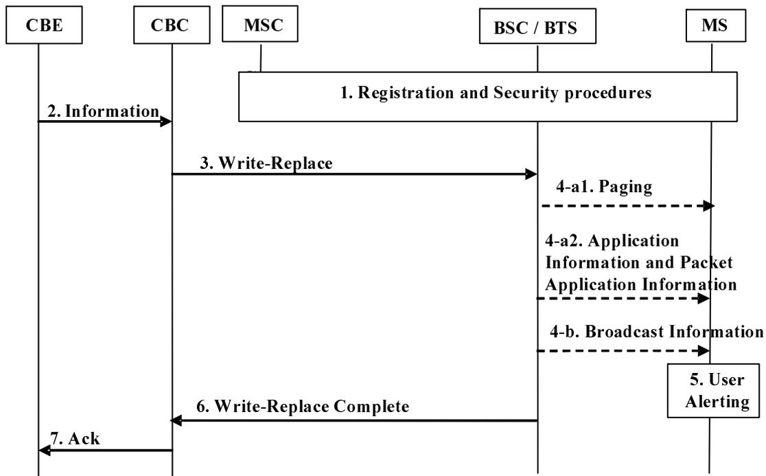
**Figure 9.1.3.2-1: Warning message delivery procedure in GERAN**
