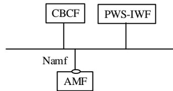
**Figure 9A.1-1: 5GS PWS system architecture – CBCF/PWS-IWF - AMF**
