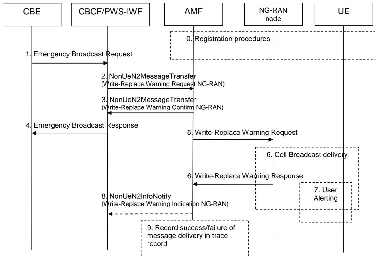
**Figure 9.1.3.5.2-1: Warning message delivery procedure in NG-RAN**
