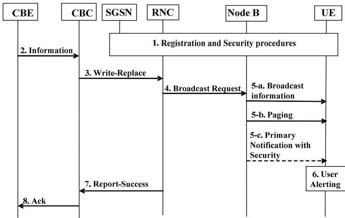
**Figure 9.1.3.3-1: Warning message delivery procedure in UTRAN**
