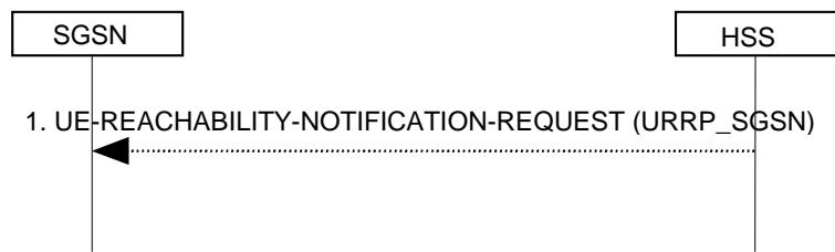
Figure 6.15-1: UE Reachability Notification Request Procedure
