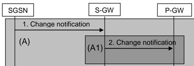
**Figure 15.1.3-3: Cell Update triggering a report of change in CGI, Iu-mode Location report triggering a report of change in SAI and User CSG information change triggering a report of change in user CSG information**
