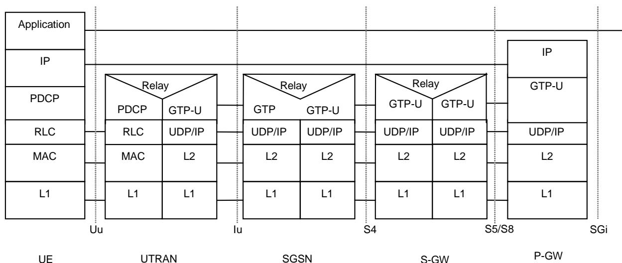
Figure 6c: User Plane with UTRAN for GTP-based S5/S8
