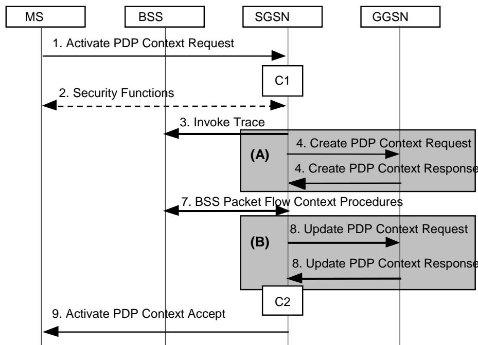
**Figure 63: PDP Context Activation Procedure for A/Gb mode**
