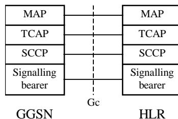
**Figure 14: Control Plane GGSN - HLR Using MAP**
