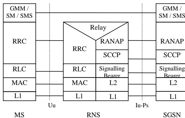
**Figure 8: Control Plane MS - SGSN in Iu mode**
