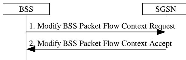
**Figure 86: BSS-Initiated BSS Packet Flow Context Modification Procedure**
