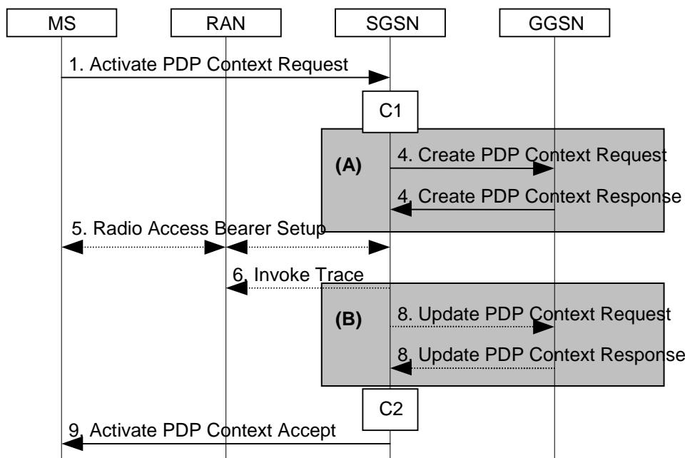
**Figure 64: PDP Context Activation Procedure for Iu mode**
