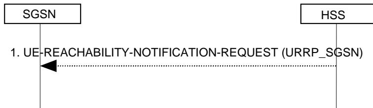
**Figure 6.15-1: UE Reachability Notification Request Procedure**
