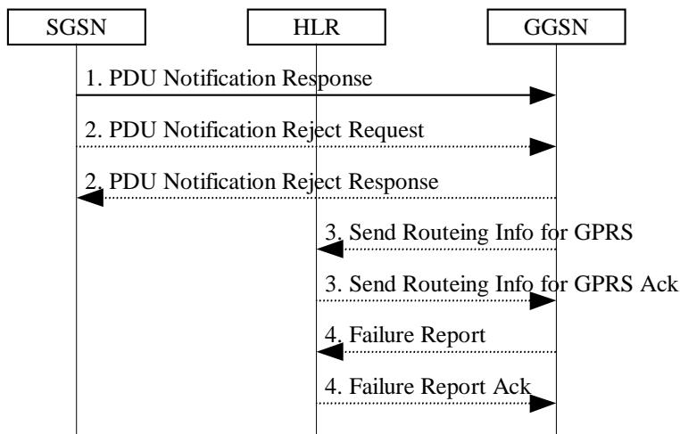
**Figure 68: Protection Procedure**
