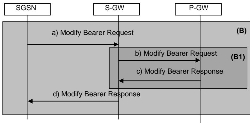
**Figure 55-3: step 8 for A/Gb mode to Iu mode Inter-SGSN Change using S4**
