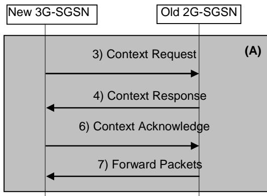
**Figure 55-2: steps 3, 4, 6, 7 for A/Gb mode to Iu mode Inter-SGSN Change using S4**
