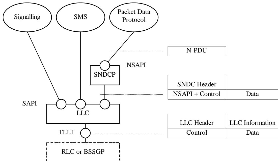
**Figure 80: Multiplexing of Network Protocols**
