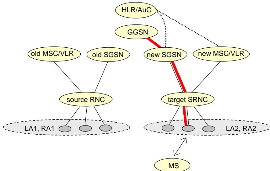
**Figure 38: After SRNS Relocation and Routeing Area Update**
