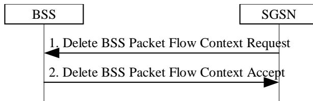
**Figure 87: SGSN-Initiated BSS Packet Flow Context Deletion Procedure**
