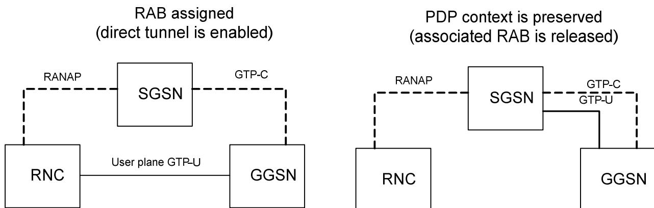
**Figure 15.6-1: IDLE mode handling for Gn/Gp connectivity**
