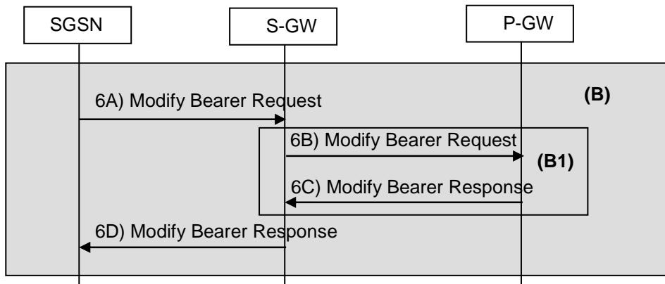
**Figure 33b: Step 6 for Inter SGSN Routeing Area Update Procedure and Combined Inter SGSN RA / LA Update to S4-SGSNs**
