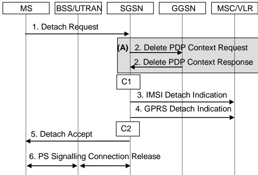
**Figure 23: MS-Initiated Combined GPRS / IMSI Detach Procedure**
