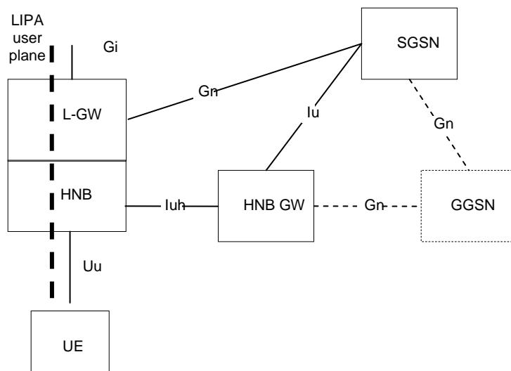
**Figure 5.4.9-2: LIPA architecture for HNB subsystem connected to a Gn-based SGSN**
