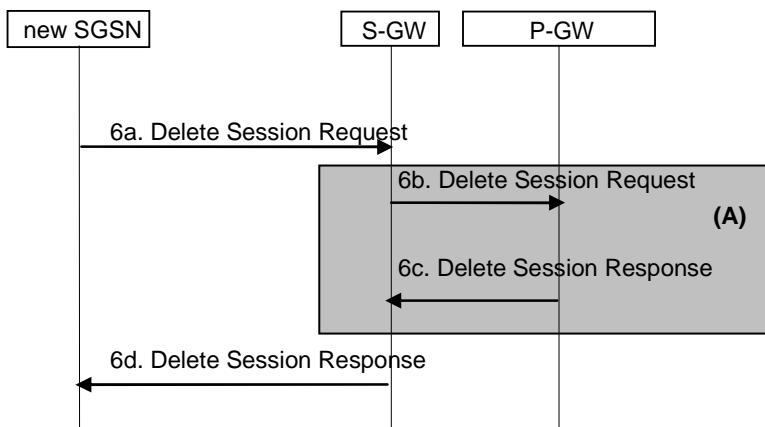
**Figure 22A: Combined GPRS / IMSI Attach Procedure**
