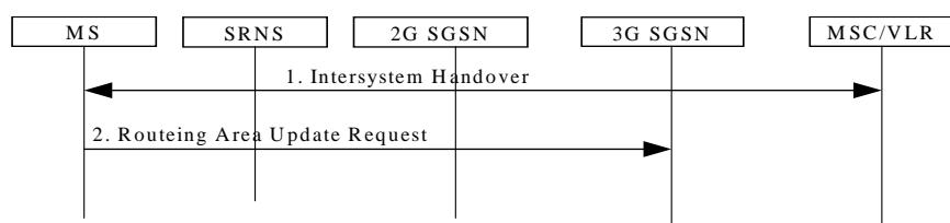
**Figure 104: Resume of GPRS traffic at inter SGSN**
