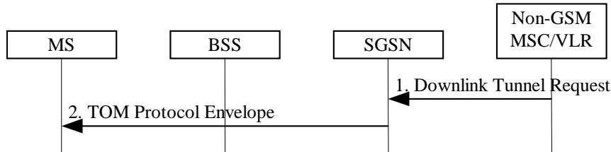
**Figure 47: Downlink Tunnelling of non-GSM Signalling Messages Procedure**
