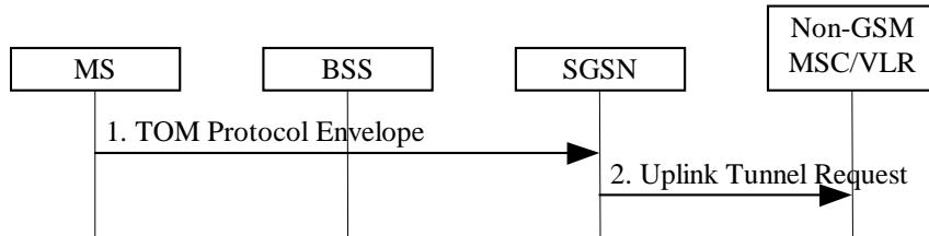
**Figure 46: Uplink Tunnelling of non-GSM Signalling Messages Procedure**
