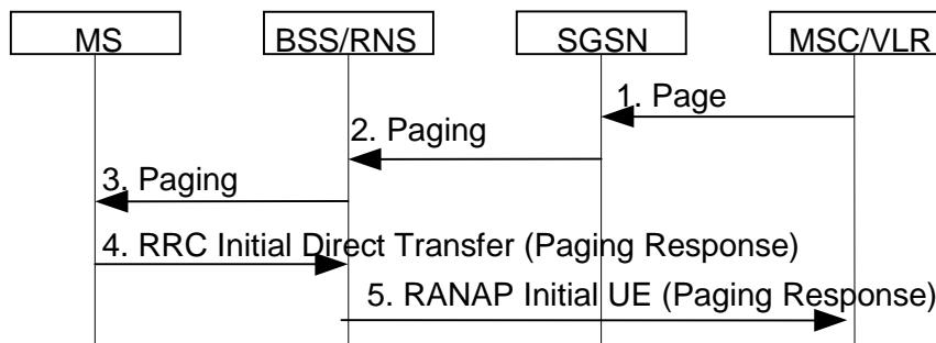
**Figure 19: CS Paging Procedure in Iu mode**
