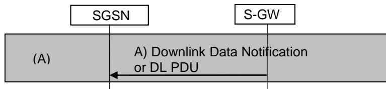
**Figure 58a: Serving GW triggered paging with S4**
