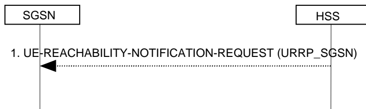
Figure 6.15-1: UE Reachability Notification Request Procedure
