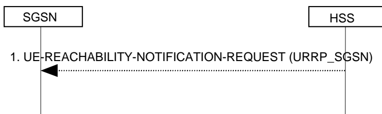
Figure 6.15-1: UE Reachability Notification Request Procedure
