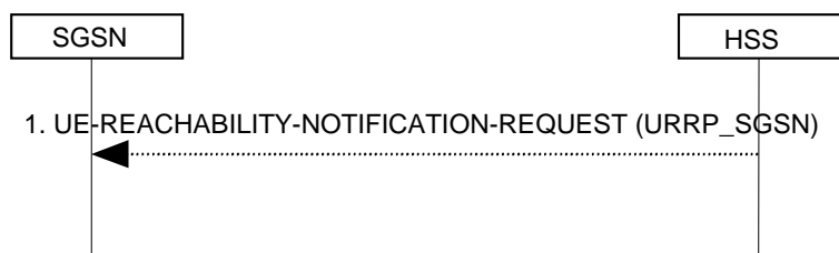
Figure 6.15-1: UE Reachability Notification Request Procedure
