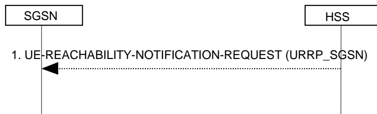
Figure 6.15-1: UE Reachability Notification Request Procedure
