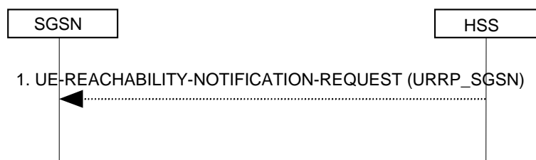
Figure 6.15-1: UE Reachability Notification Request Procedure
