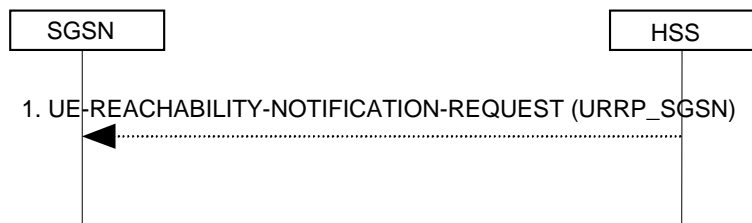
Figure 6.15-1: UE Reachability Notification Request Procedure
