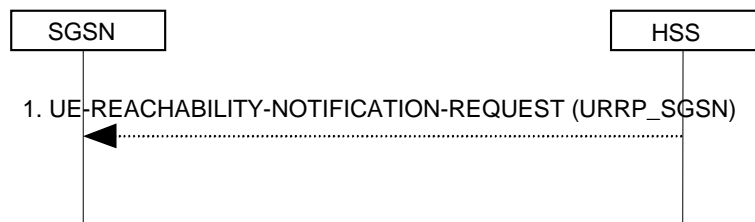
Figure 6.15-1: UE Reachability Notification Request Procedure
