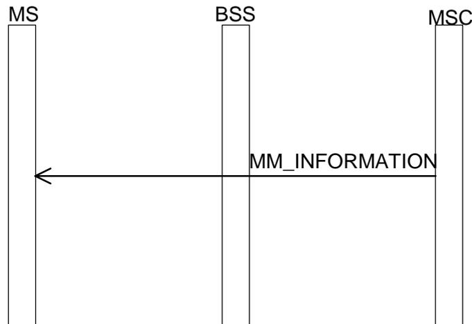
Figure 9: Signalling information required at notification of LSA change in active mode
