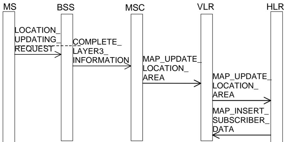
**Figure 2: Signalling information required at location registration**
