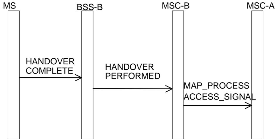
Figure 8: Signalling information required at BSS internal handover
