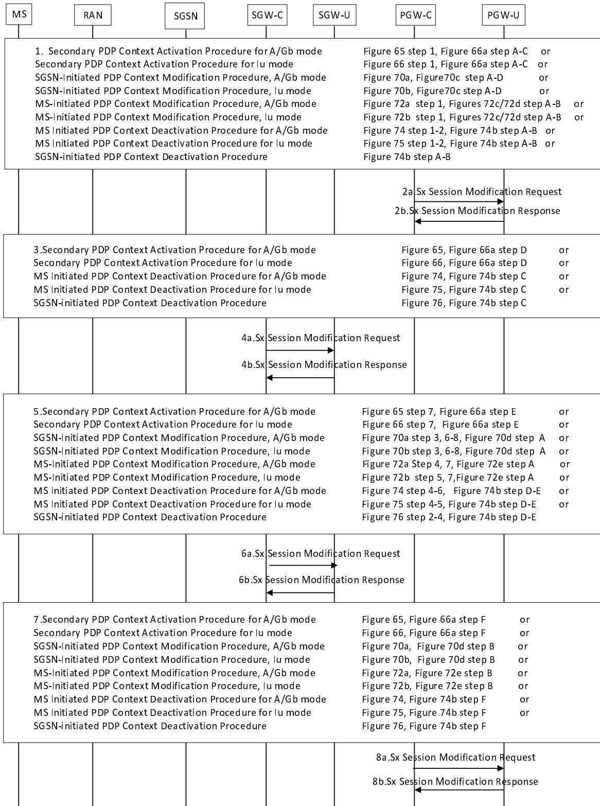
Figure 6.3.4.2.1-2: Interaction between CP and UP function with PDN connection modification, Group 2
