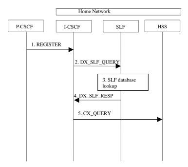
Figure 5.20: SLF on register (1st case)
