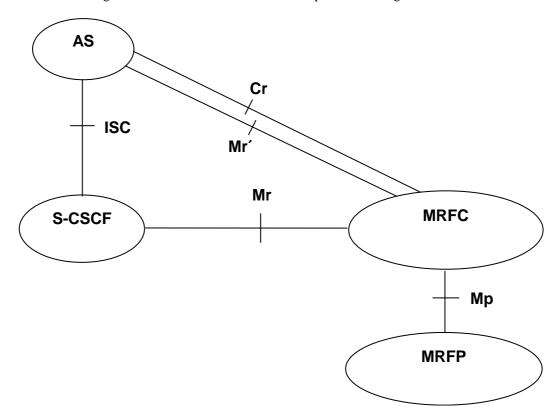
Figure 4.7: Architecture of MRF
