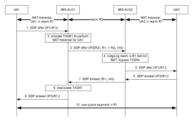
Figure Q.4: IMS-ALG bypasses TrGWs performing NAT traversal
