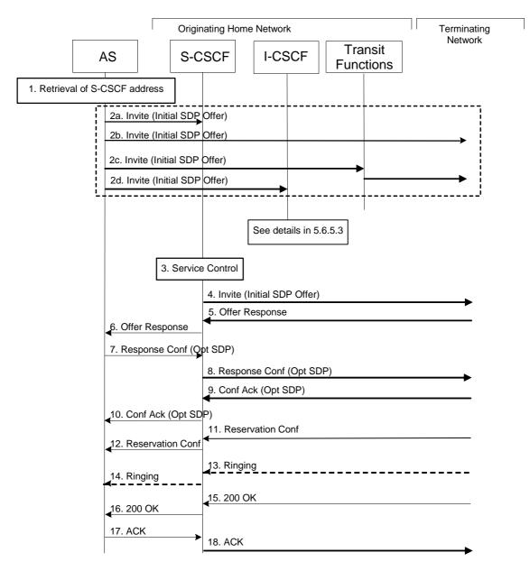
Figure 5.16b: Application Server origination procedure
