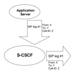
Figure 4.3b: Application Server acting as originating UA
