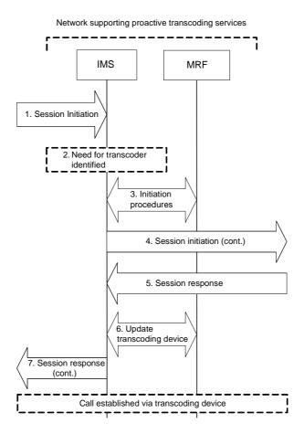
Figure P.1.3.2-1: Proactive transcoding triggering logic
