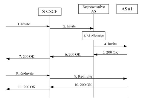
Figure J.2.2: Bypassing Representative AS procedure
