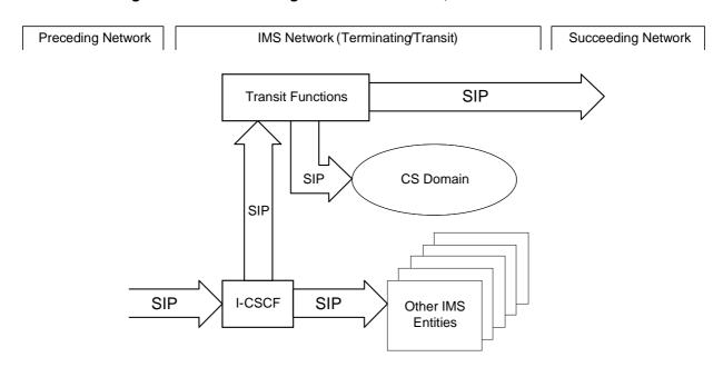
Figure 5.50b: Terminating/Transit IMS network, I-CSCF first
