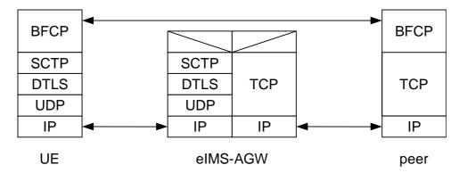
Figure U.1.5.2-1: Protocol architecture for BFCP
