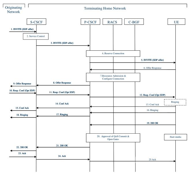
Figure N.2.1: Fixed xDSL terminating - home (example flow)
