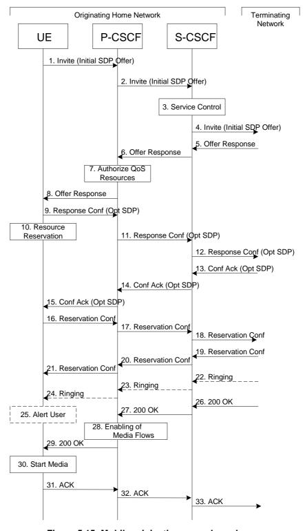
Figure 5.15: Mobile origination procedure - home
