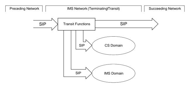
Figure 5.50a: Terminating/Transit IMS network, Transit Functions first
