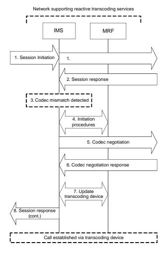
Figure P.1.3.3-1: Reactive transcoding triggering logic
