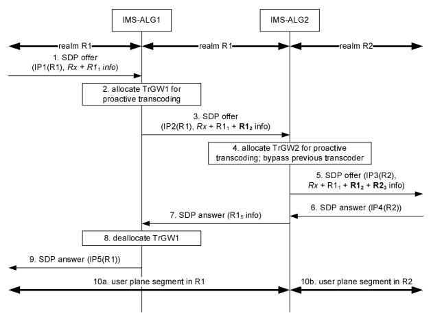
Figure Q.8: IMS-ALG replaces prior proactive transcoder
