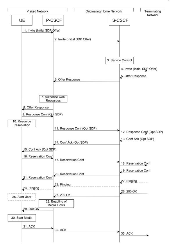
Figure 5.14: Mobile origination procedure - roaming
