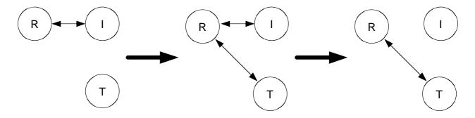
An Assured Transfer is identical to the above, except that I waits until the Refer successfully completes before issuing the BYE message to terminate its connection with R. If the new session from R to T were to fail, R would still have a session with I.
