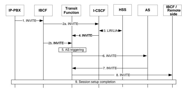
Figure S.2-2: Originating procedures for IP-PBXs using static mode business trunking and served by the Transit Function
