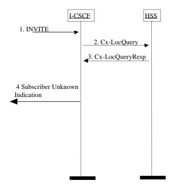
Figure 5.45: HSS determination of unknown user
