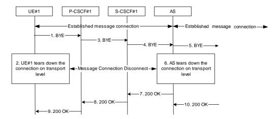
Figure 5.48e: Message session release procedure with intermediate node
