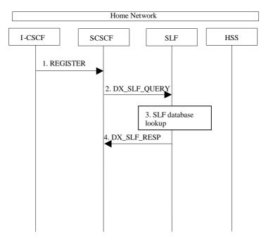
Figure 5.20a: SLF on register (2<sup>nd</sup> case)
