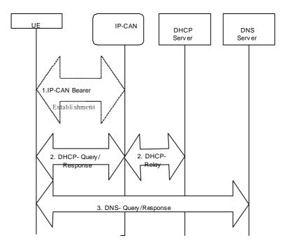
Figure 5.0a: P-CSCF discovery using DHCP and DNS
