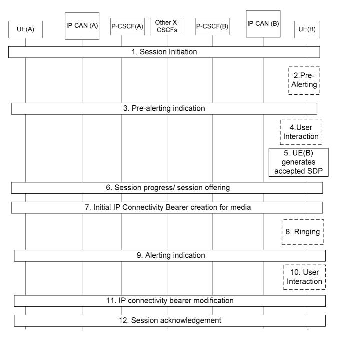
Figure 5.7: Bearer establishment showing optional pre-alerting
