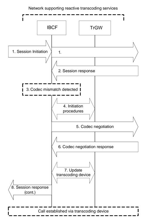
Figure I.5: Reactive transcoding invocation
