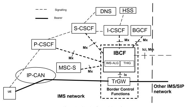
**Figure I.1: Border Control Functions**
