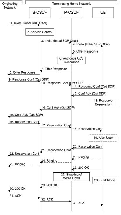
Figure 5.18: Mobile termination procedure - home
