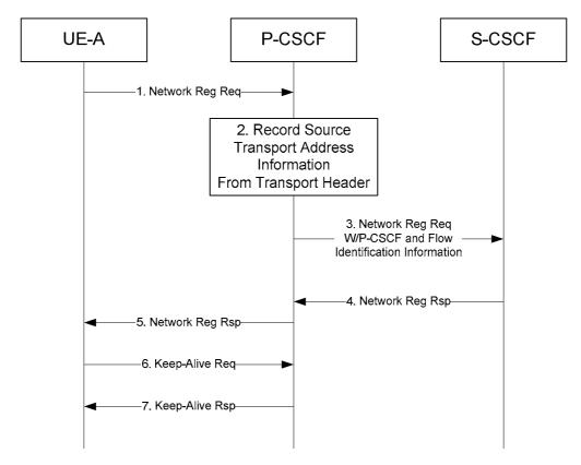
Figure G.7: Flow Establishment Procedures for Outbound
