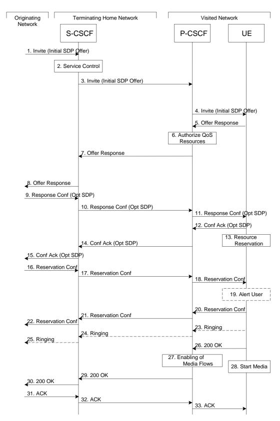
Figure 5.17: Mobile termination procedure - roaming
