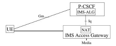
Figure G.2: Reference model for IMS access when NAT is needed between the IP-CAN and the IMS domain
