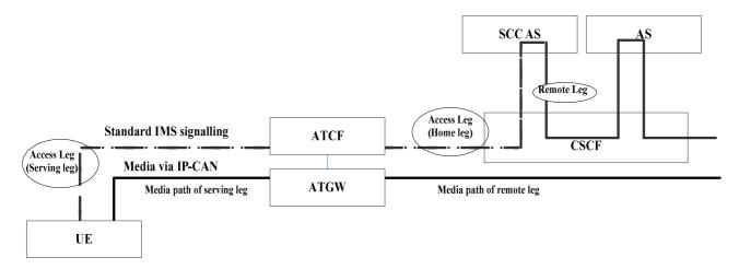
Figure 5.4.2a-1: Signalling and bearer paths for sessions with PS media using ATCF
