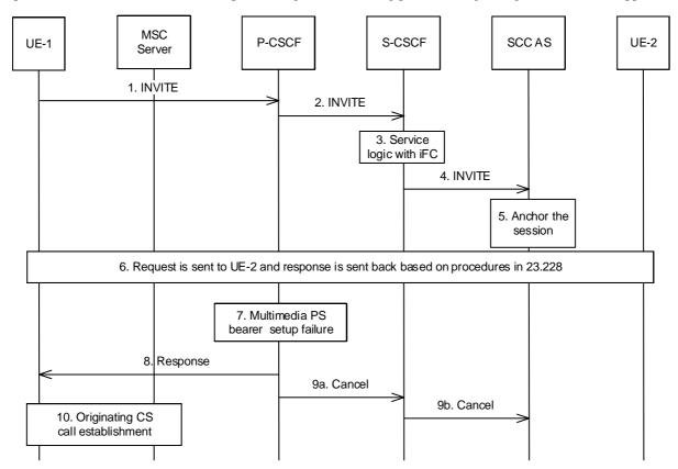
Figure 6.2.1.3a-1: Originating session that uses only PS media - fallback to CS domain in pre-alerting phase
