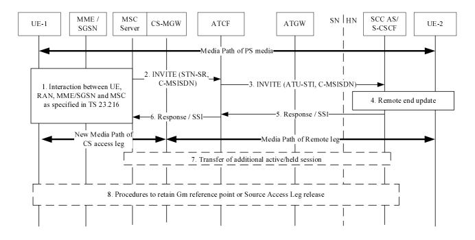
Figure 6.3.2.1.9.2-1: PS to CS access transfer
