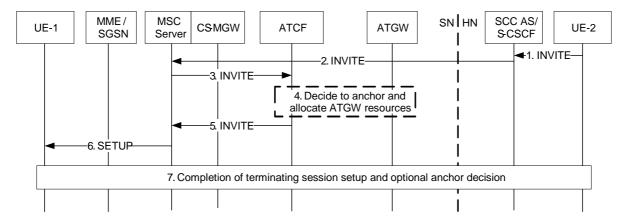
Figure 6.2.2.6-1: Terminating call setup over CS through ATCF
