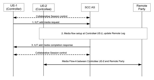
Figure 6a.4.2.1-1: Controller UE initiated add new media on Controllee UE belonging to the same IMS subscription
