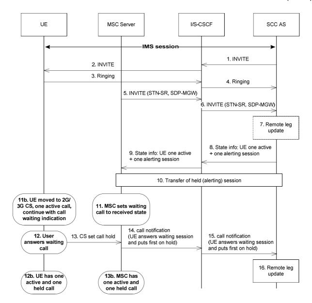
Figure 6.3.2.1.7a-1: PS-CS: PS to CS - Single Radio, mid-call service with an incoming waiting call in alerting phase
