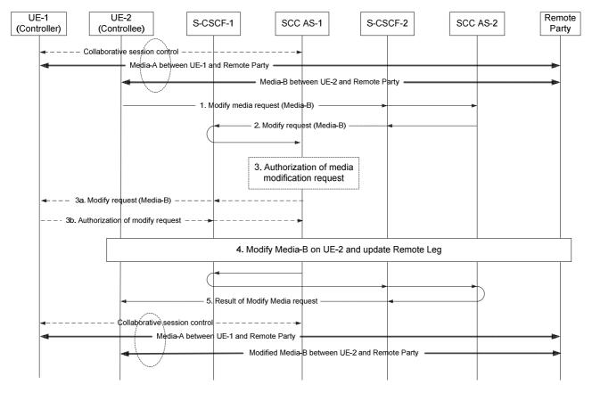
Figure 6a.4.6.2-1: Controllee UE initiated media modify on itself (different IMS subscriptions under the same operator)
