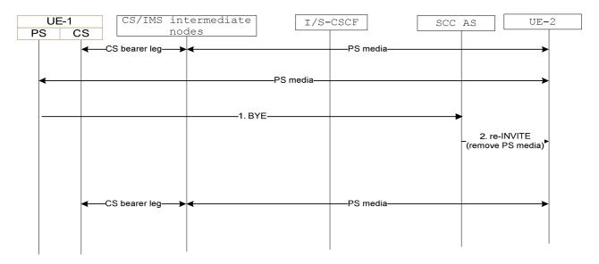
Figure 6.3.3.7-1: Local End Initiation case – Removing media from split CS and PS sessions
