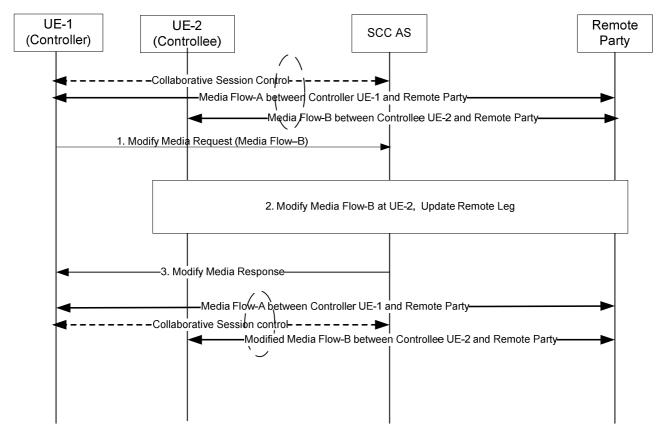
Figure 6a.4.4a.1-1: Controller UE initiated media modify on a Controllee UE belonging to the same IMS subscription
