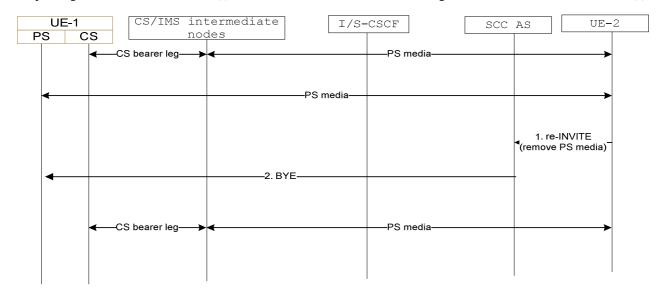
Figure 6.3.3.8-1: Remote End Initiation case – Removing media from split CS and PS sessions
