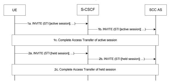
Figure 6.3.2.3.5-1: PS-PS in conjunction with PS-CS Access transfer: Active/Held sessions
