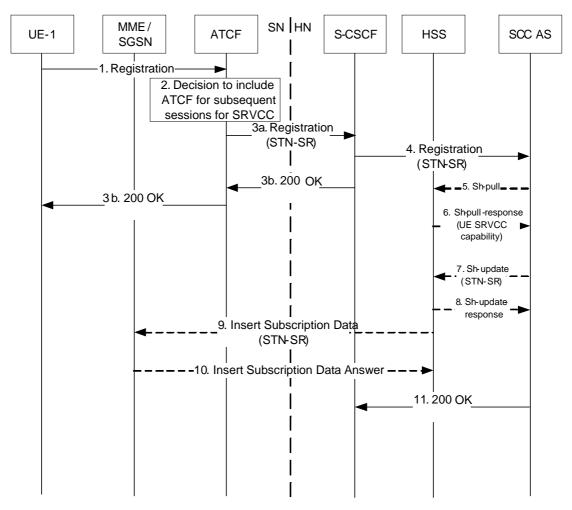
Figure 6.1.2-1: IMS Registration using ATCF enhancements
