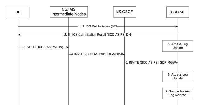
Figure 6.3.2.3.8-1: PS-CS in conjunction with PS-CS Access Transfer: PS to CS access - using I1 reference point
