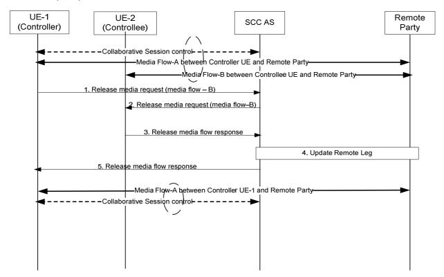
Figure 6a.4.4.1-1: Controller UE Initiated Media release – media flow on Controllee UE (Controller and Controllee belong to the same IMS subscription)
