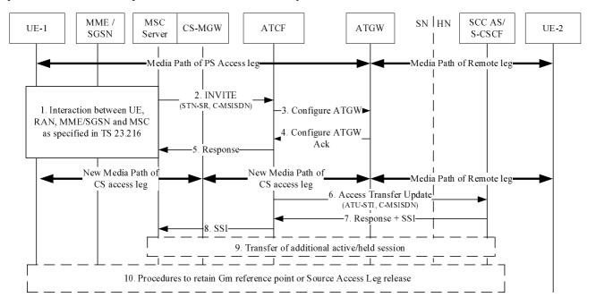
Figure 6.3.2.1.9.1-1: PS to CS Access Transfer when using ATCF enhancements and media anchored.
