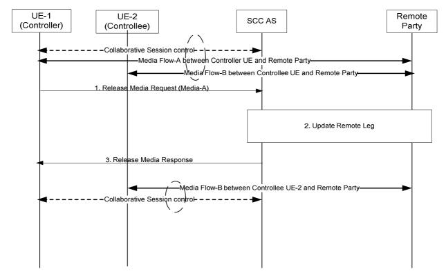
Figure 6a.4.3-1: Controller UE Initiated Media release – media on Controller UE
