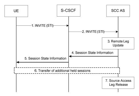
Figure 6.3.2.1.2a-1: CS to PS Access Transfer - Dual Radio with Session State Information
