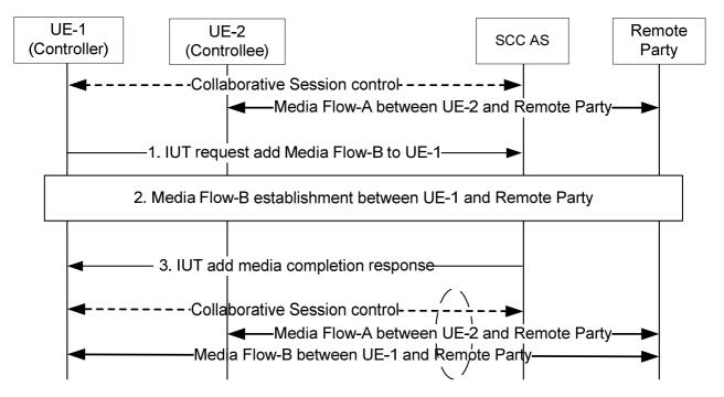
Figure 6a.4.1-1: Controller UE initiated add new media On Controller UE
