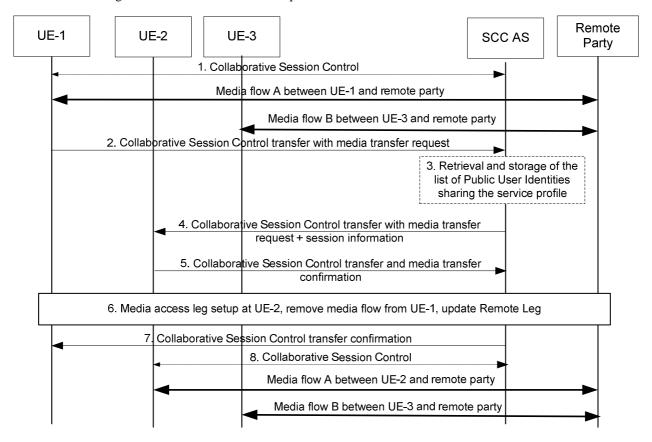
Figure 6a.4a.2-1: Controller UE initiated transfer of Collaborative Session Control with transfer of media flow
