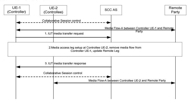
Figure 6a.3.1.1-1: Controller UE initiated media transfer from Controller UE to Controllee UE belonging to the same IMS subscription
