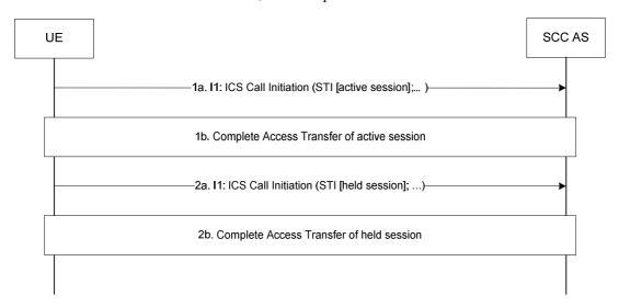
Figure 6.3.2.3.10-1: PS – PS in conjunction with PS – CS Access Transfer: PS to CS for Active/Held sessions – using I1 reference point
