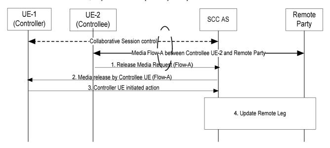
Figure 6a.4.5-1: Controllee UE initiated release media flow on itself
