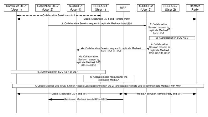
Figure 6a.10.4-1: Replicating media in network from Controller UE to another UE belonging to different IMS subscription – pull mode
