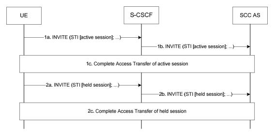
Figure 6.3.2.3.11-1: PS – PS in conjunction with PS – CS Access Transfer: CS to PS for Active/Held sessions - using I1 reference point
