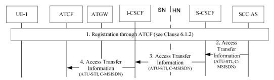
Figure 6.3.1.7-1: Access Transfer Information provided to ATCF from SCC AS
