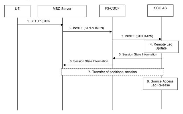
Figure 6.3.2.1.1a-1: PS - CS Access Transfer: PS to CS - Dual Radio with Session State Information
