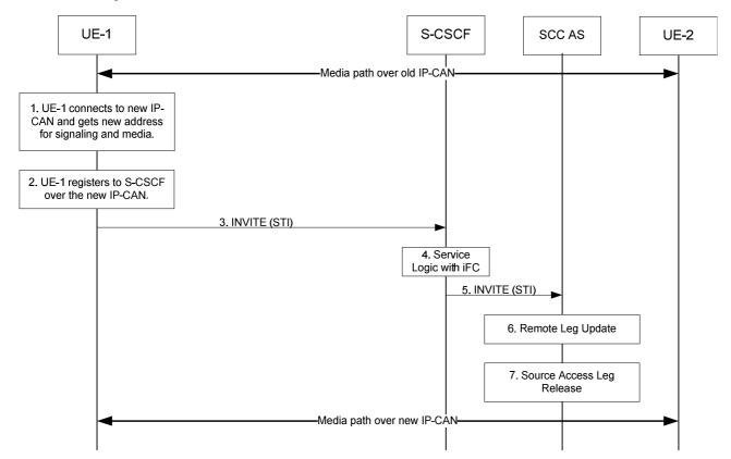
Figure 6.3.2.2.1-1: Information flow for PS-PS Access Transfer
