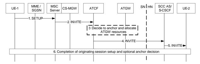
Figure 6.3.3.5.3-1: Originating call setup over CS through ATCF
