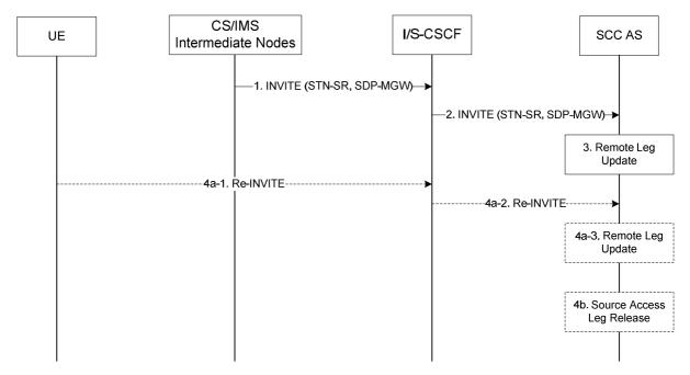
Figure 6.3.2.1.4-1: PS-CS: PS to CS - Single Radio
