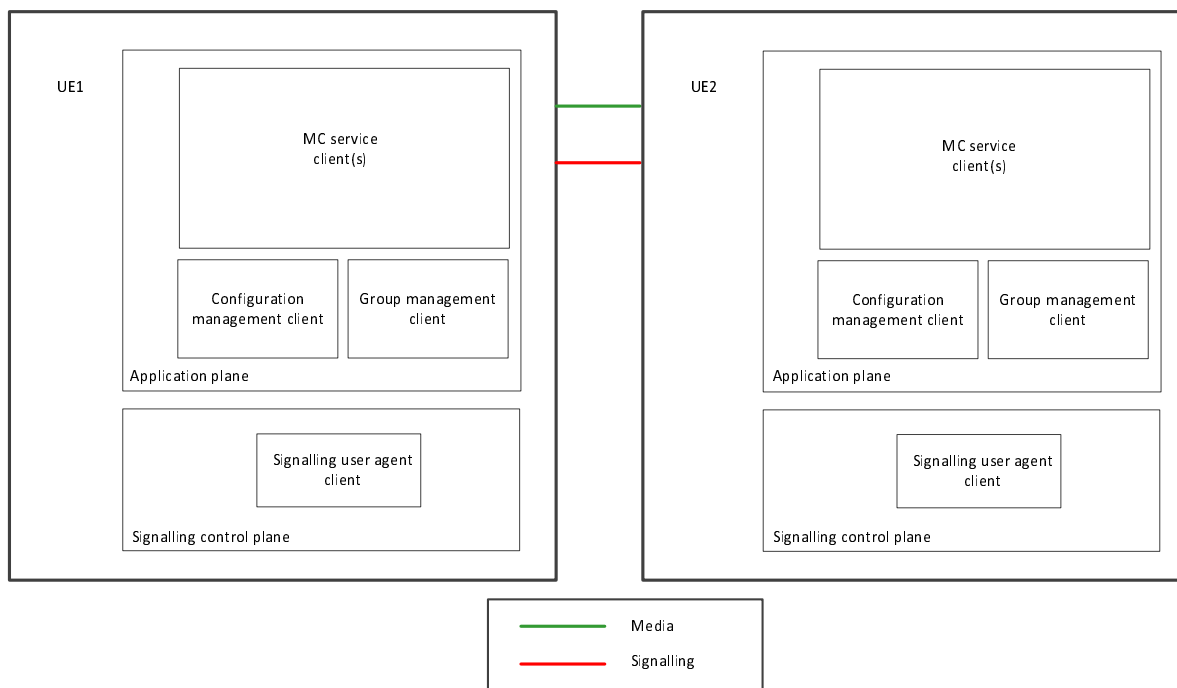
Figure 7.3.2-1: Functional model for MC service off-network operation
