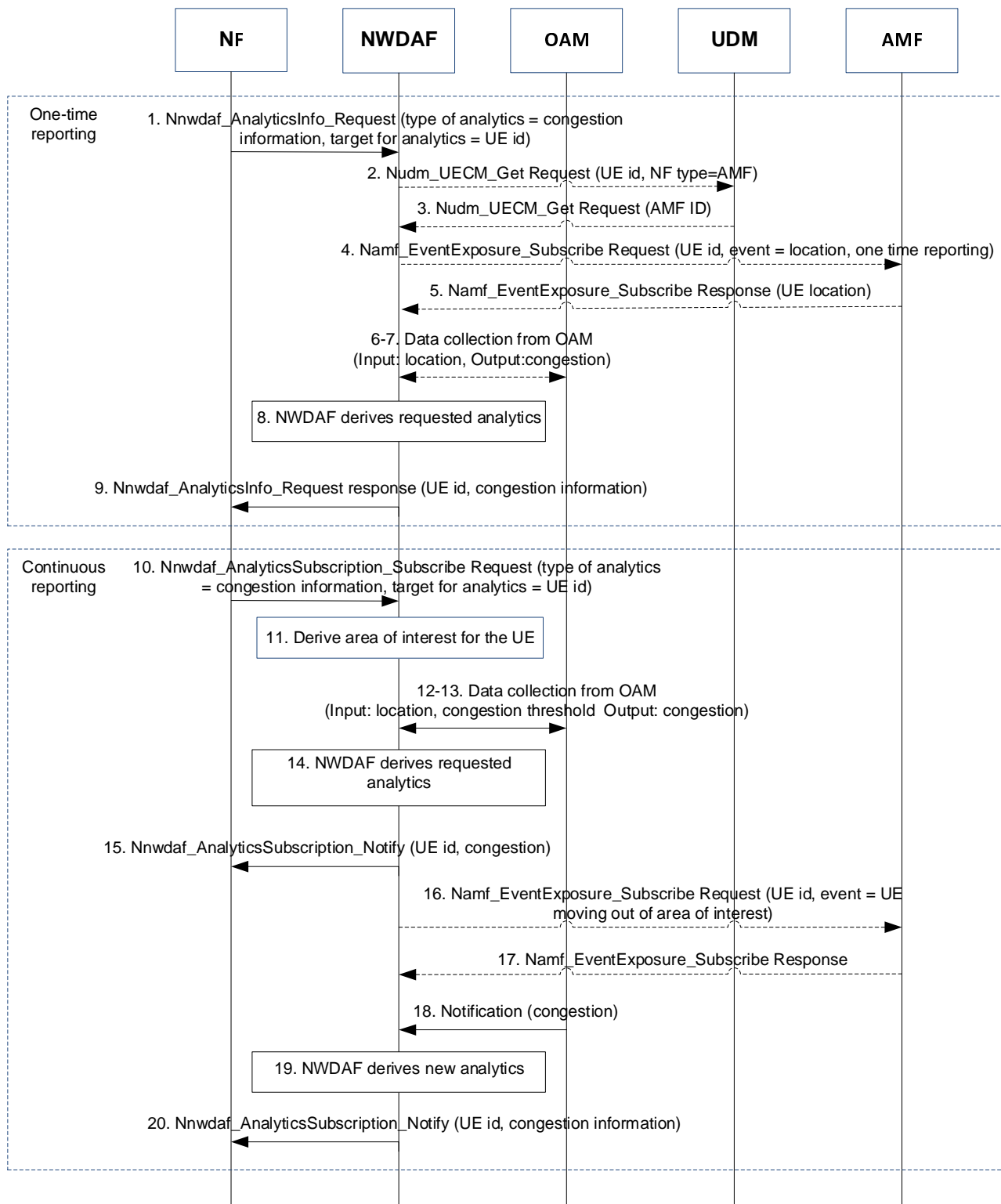
Figure 6.8.4.2-1: Procedure for one-time or continuous reporting of analytics for congestion for a specific UE
