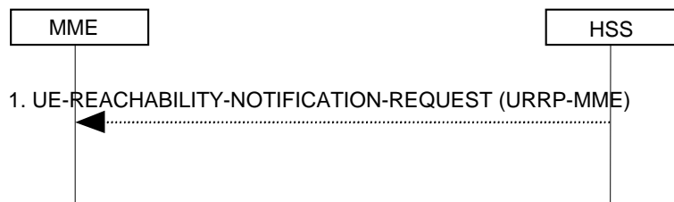
Figure 5.3.11.2-1: UE Reachability Notification Request Procedure
